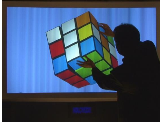
Figure 2-12 Multi-beam light field 3D display using the Holograik technique to produce a natural 3D view [64].
