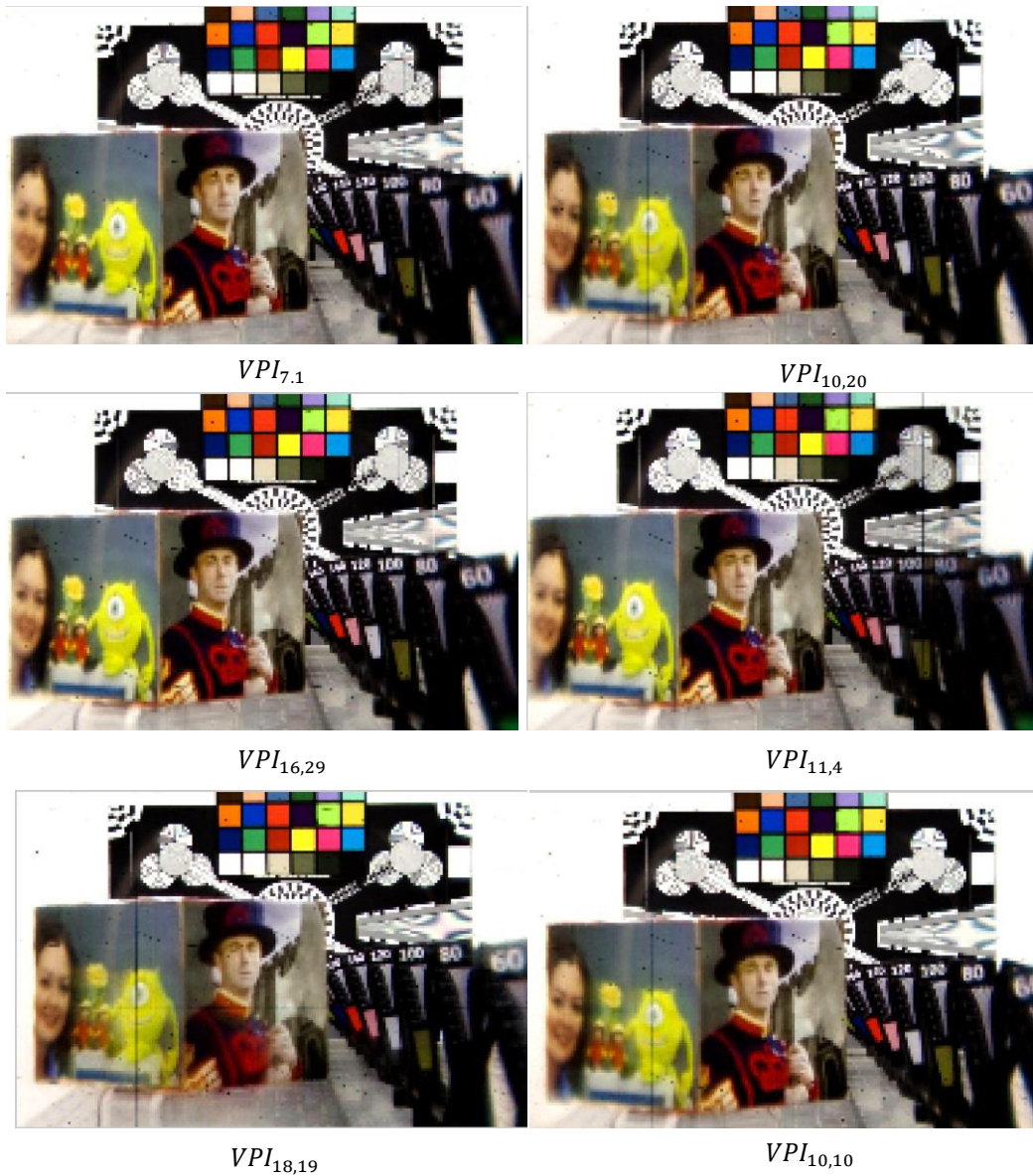
Figure 3-14 Various display positions of VPIs extracted from the OH3DI “Box” by periodically extracting pixels from the captured EIs. It is a real-world image captured at the 3D VIVANT project lab. The resolution of the image is 5616 \times 3744 pixels. A 29 \times 29 grid of VPIs was extracted from the image each with 193 \times 129 pixels.
