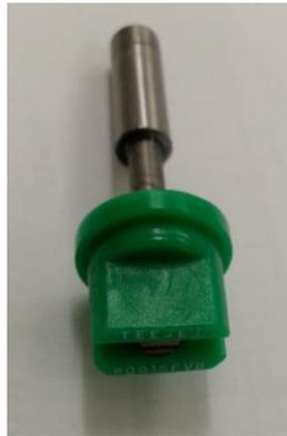
**Figure 4.1: The fan hydraulic nozzle.**
