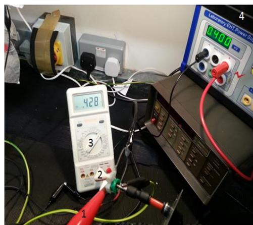
**Figure 6.14: The procedure used to check the nozzle electrode voltage: high voltage prop (1), induction nozzle (2) multimeter (3) and high voltage supply (4).**
