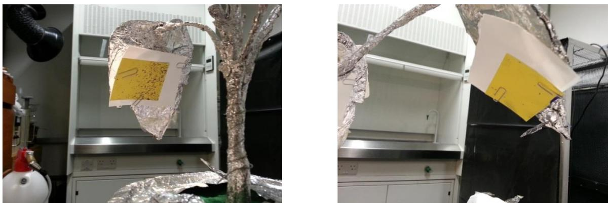
**Figure 6.23: The coverage area on the back of the leaf target under the charged (left) and uncharged condition (right).**
