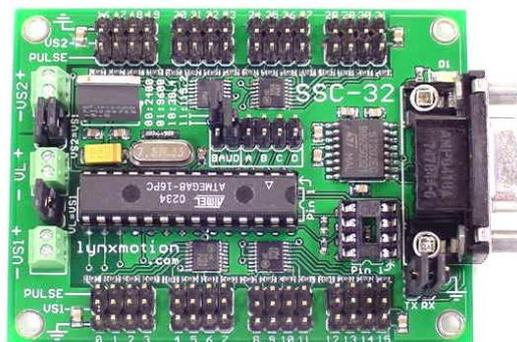
**Figure 5.10: The SSC-32 robot arm control board.**
