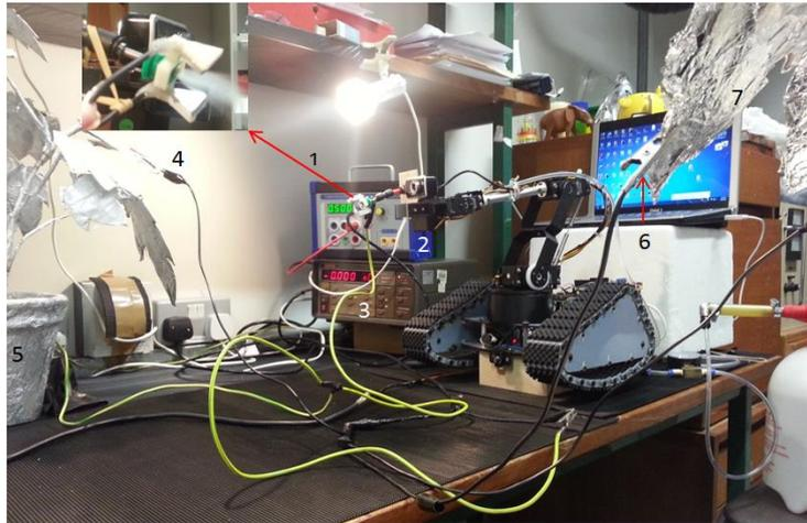
**Figure 6.13: The experimental setup for measuring the spray current on the artificial plant: induction nozzle (1), high voltage supply (2), electrometer (3), electrometer nippers with the target (4, 6) and artificial plants (5 and 7).**
