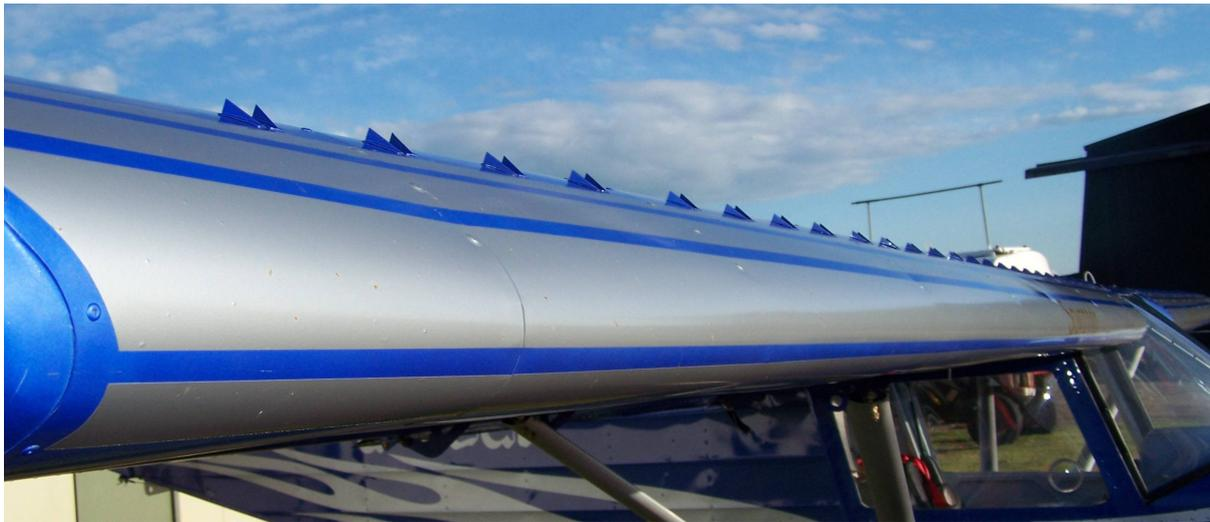
Figure 3, Savannah VG leading edge vortex generators
