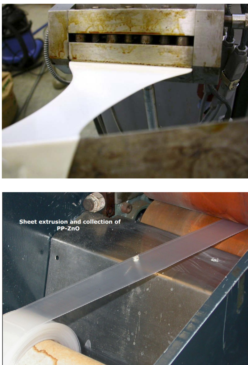
Figure 5.6 Sheet extrusion and collection of the PP – ZnO nanocomposites
