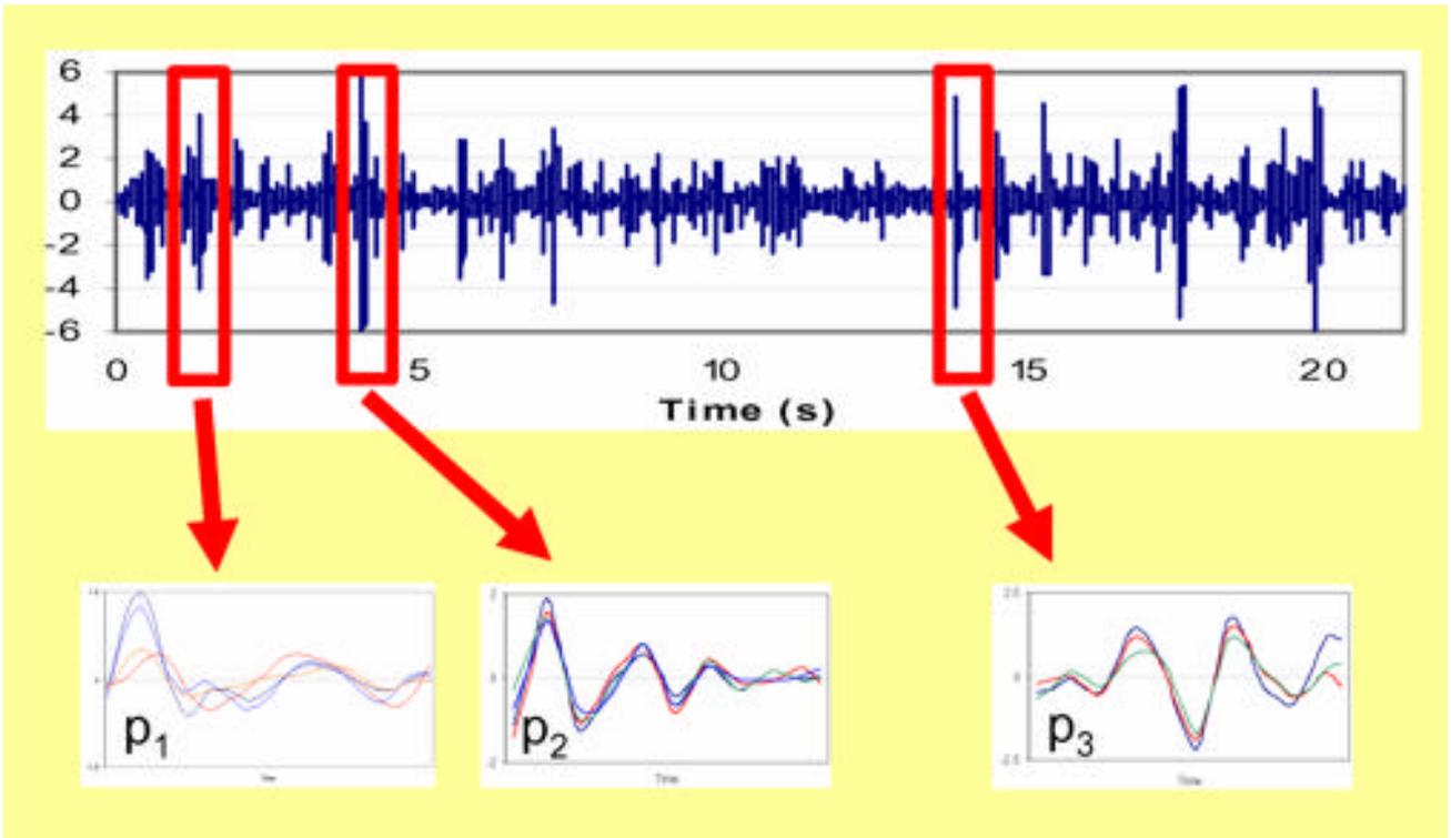
Figure 6 Feature extraction from a steering vibration time history.
