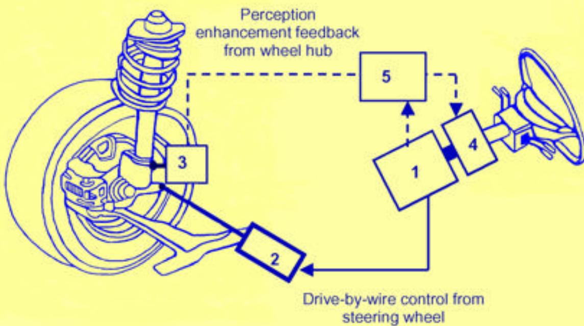
Figure 1 A perception enhancement system for by-wire steering.
