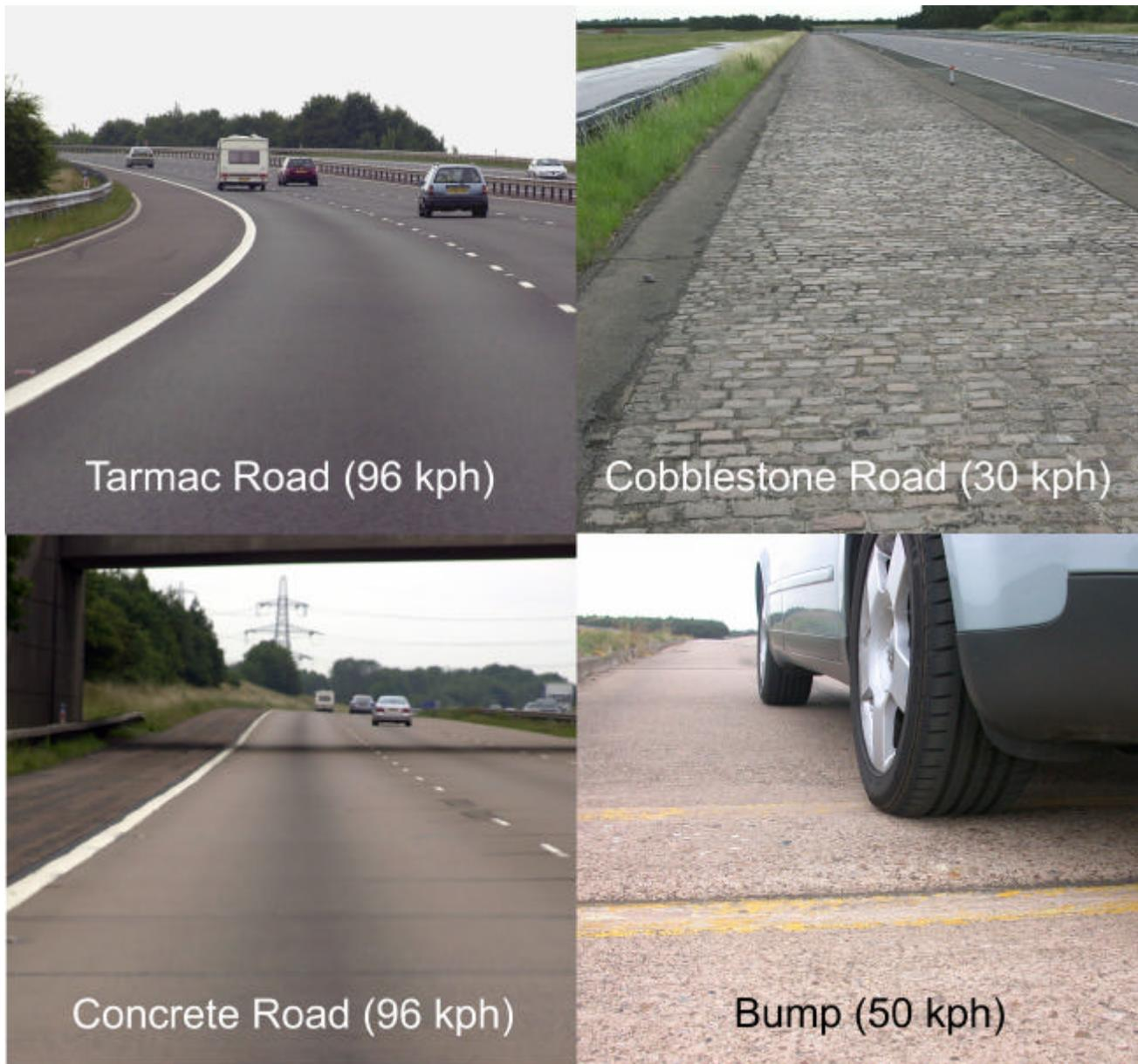
Figure 2 Road surfaces which produced the steering wheel acceleration time histories used in the laboratory experiments.
