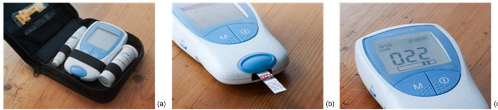
Figure 2: (a) CoaguChek testing kit; (b) Test Strip inserted; (c) Test results on CoaguChek [35] 338x75mm (96 x 96 DPI)
