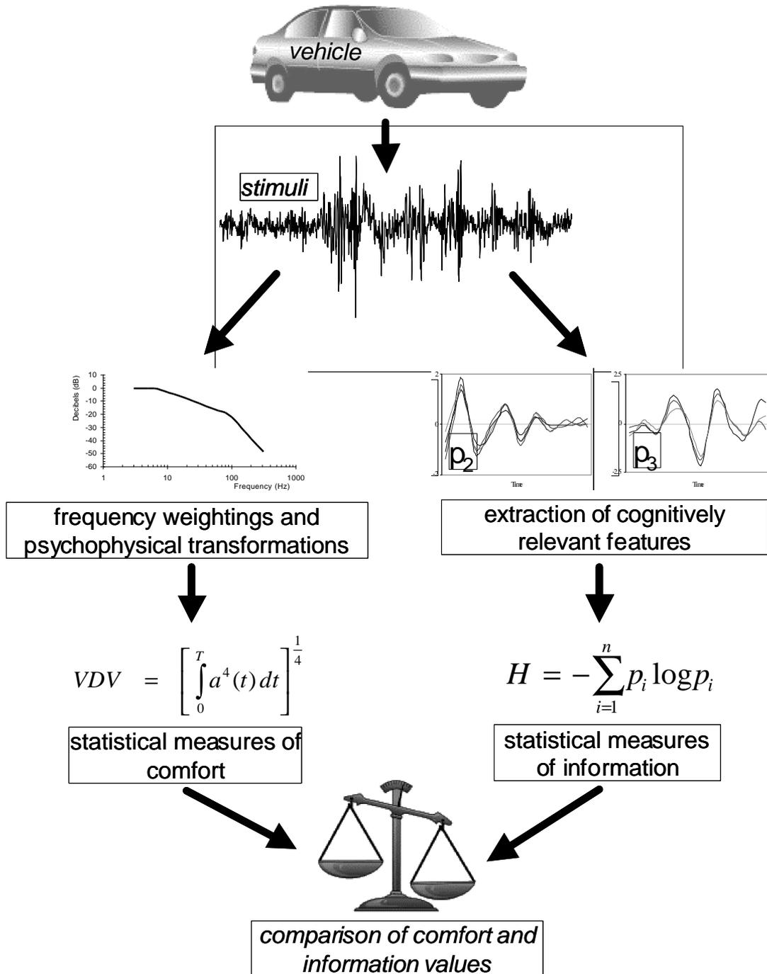
Figure 1 Evaluation of the comfort and information properties of vehicle vibrational stimuli.
