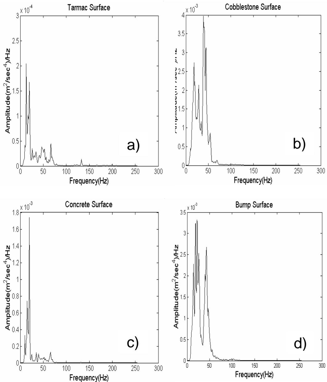
Figure 5 Acceleration power spectral densities of the steering wheel tangential direction acceleration time histories.
