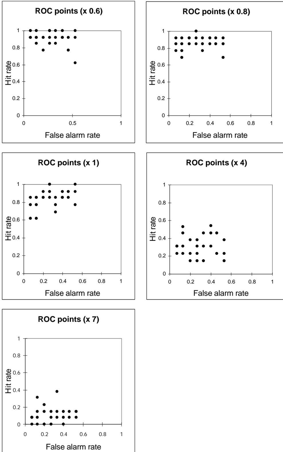
Figure 8 ROC points for the tarmac surface stimuli determined from the data of the experiment to investigate the effect of stimuli acceleration level.
