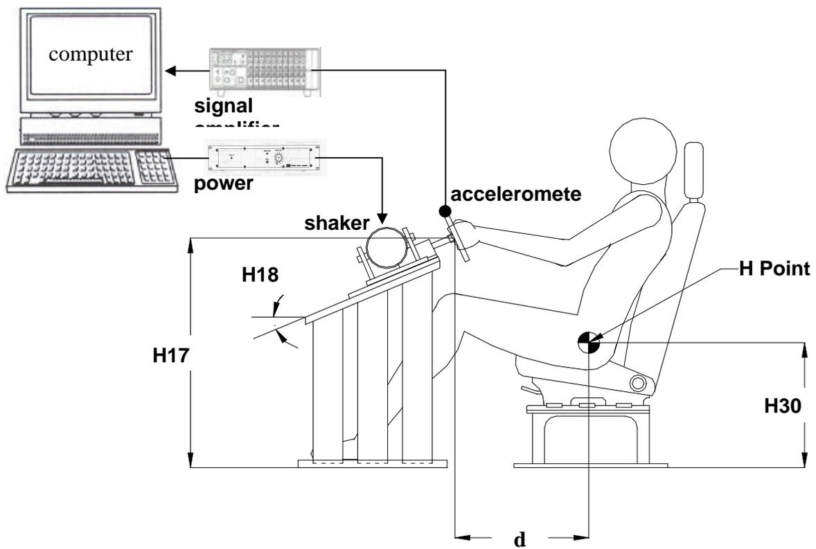
Figure 6 Steering wheel rotational vibration test facility.
