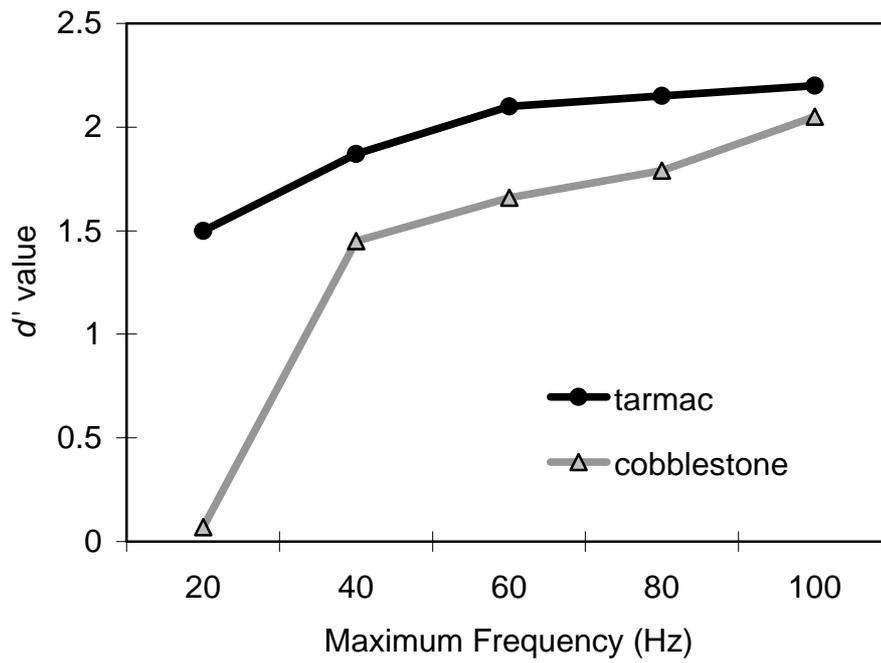
Figure 10 Sensitivity  $d'$  determined from the data of the experiment to investigate the effect of stimuli frequency bandwidth.
