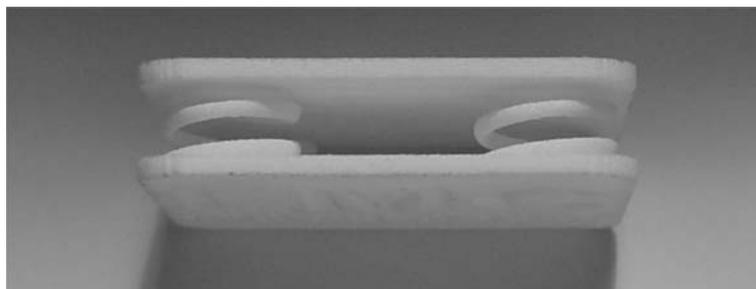
**Figure 11. Product created with internal springing (single material)**
