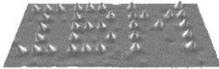
**Figure 12. IBM logo built from 35 individual atoms
