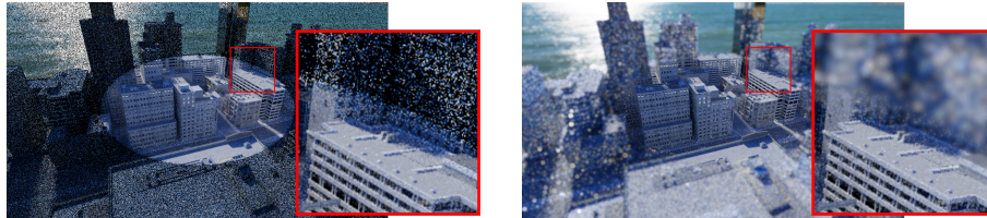
(a) An unfiltered image with at most 128 samples per pixel (b) Result of the Gaussian filtering approach applied to the same image
