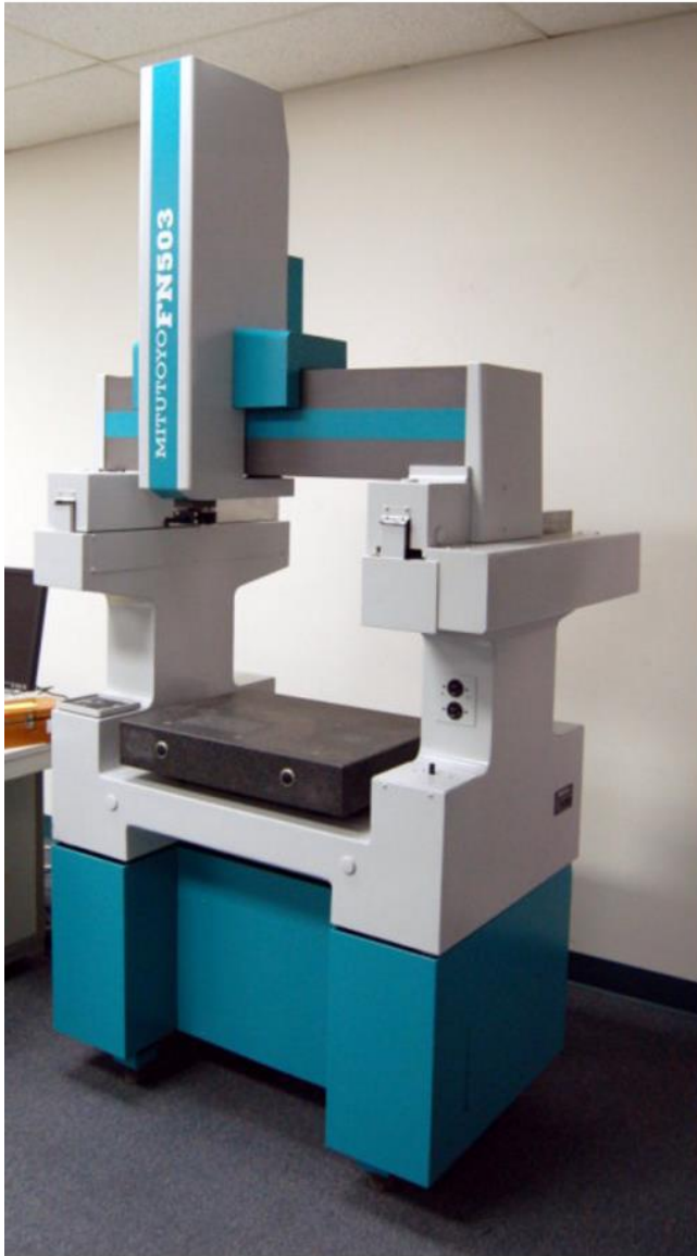
Figure D8. Specifications of Coordinate Measuring Machine (CMM) – MITUTOYO FN503
