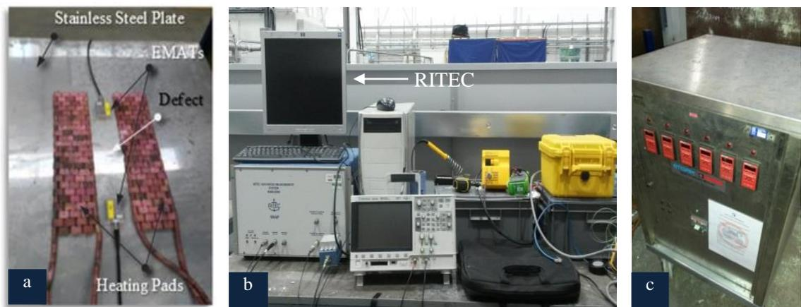
Figure 5.5. High temperature experimental set-up (a) EMATs attached upon specimen (b) electrical instrumentation - RITEC (c) thermal instrumentation
