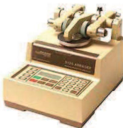
Figure 3.2 Taber rotary platform abrasion tester (pic. Source Falex Tribology)
