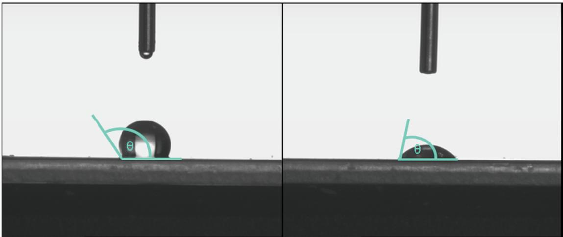
*Figure 6.2 WCA (left) and DCA (right) measurements principle taken using a DSA100 from KRÜSS*
