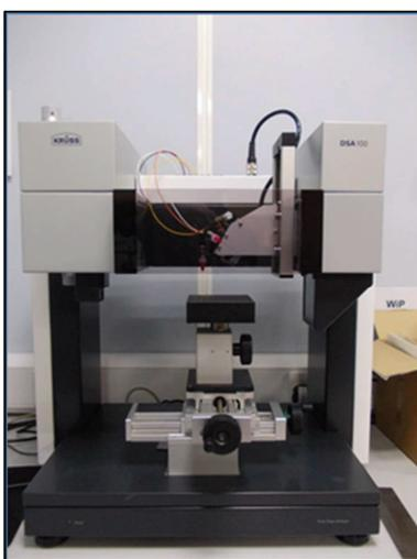
Figure 5.1 Drop shape analyser from KRÜSS
