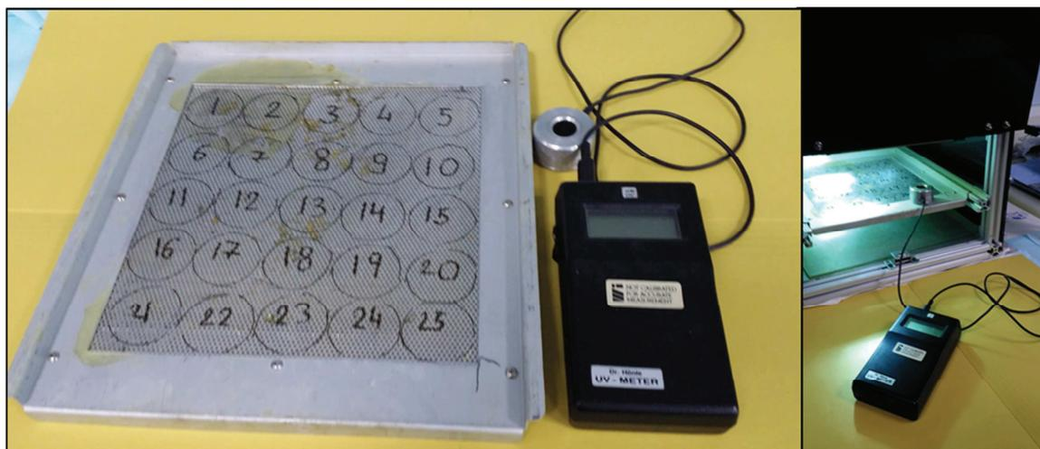
Figure 4.6 Calibration procedure of selected UV curing system
