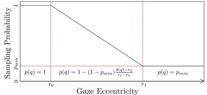
Figure 1. The sampling probability of each individual pixel is computed by evaluating the foveal function with freely adjustable parameters ( $r_0, r_1, p_{min}$ ). Image adapted from Roth et al. (2016).
