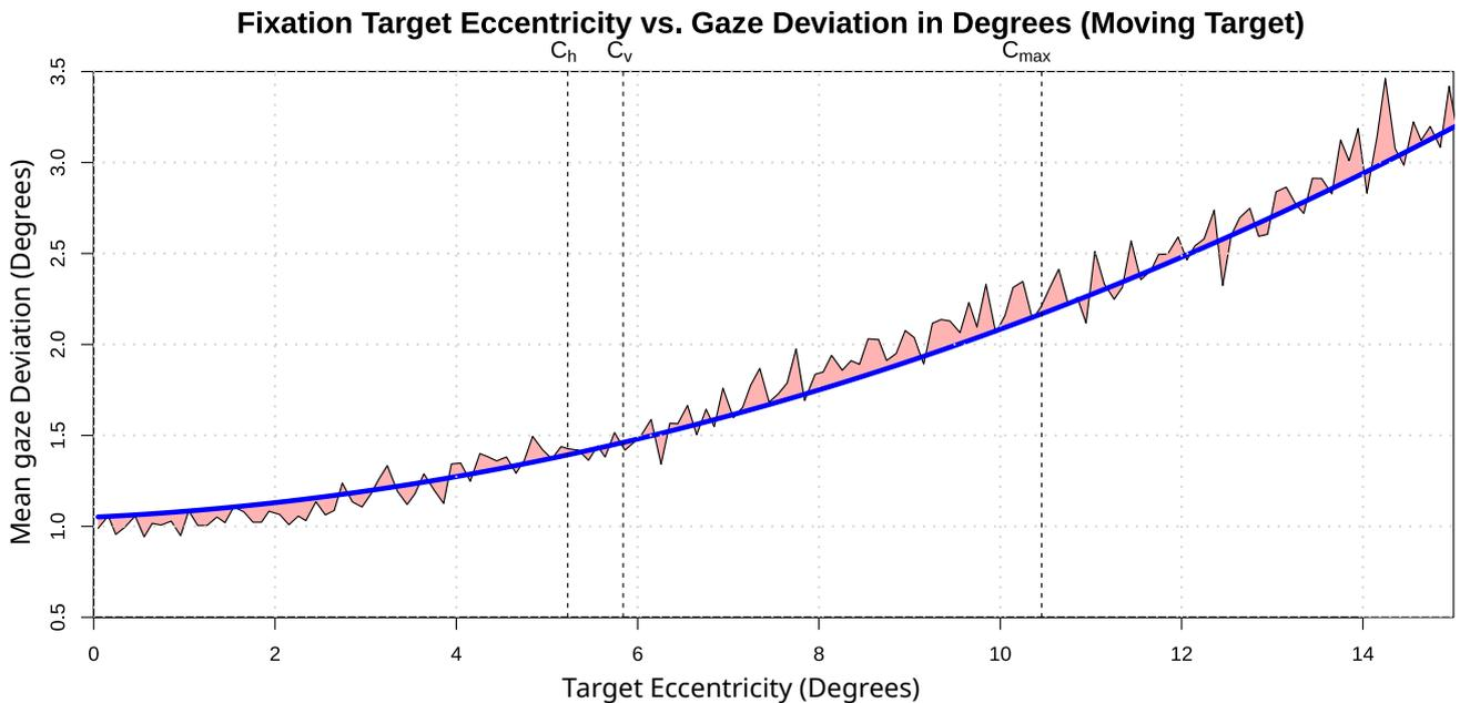
Figure 4. Tracking precision vs. fixation target’s distance to the image center. The area used for calibration by our tracking device is also denoted here by  $C_h$  (horizontal extent),  $C_v$  (vertical extent) and  $C_{max}$  (diagonal extent). The result of linear regression with a quadratic equation is represented by the blue line. The red area illustrates the residuals. *Image adapted from Roth et al. (2016).*
