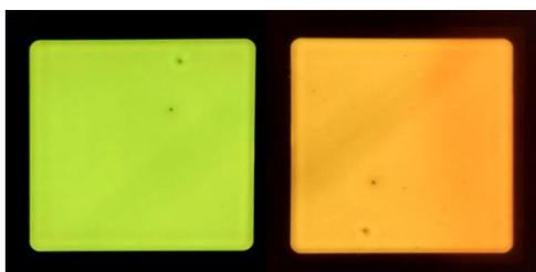
Figure 3.9: Photographs of a pure green OLED (left) and the device down-converted with the 0.5% rhodamine layer (right).
