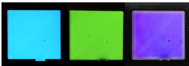
Figure 3.7: Conversion of a blue OLED (left) with the acrylic layers composed of fluorescein (middle) and rhodamine (right).
