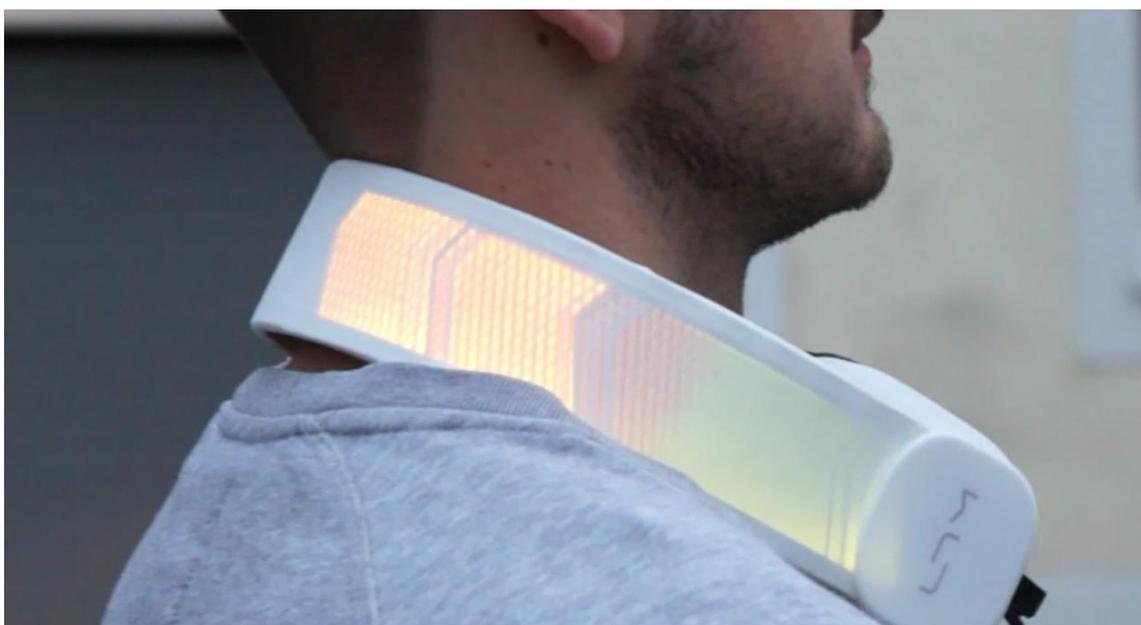
Figure 3.11: MeLite by Pilotfish; luminescent headphone consisting of a green OLED down-converted with the acrylic-rhodamine coating.
