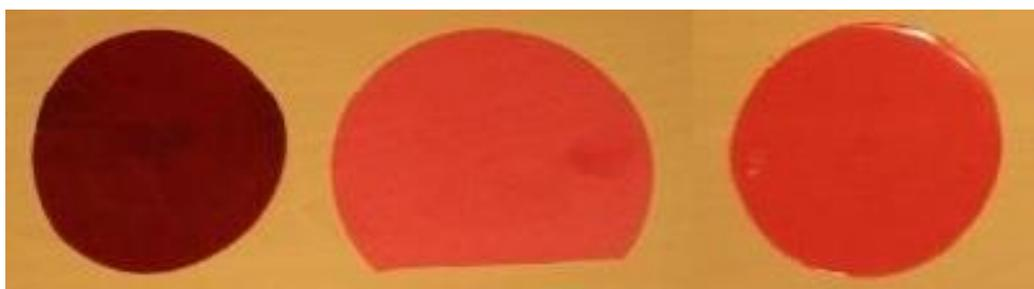
Figure 3.1: Thermoplastic polymer discs containing 0.5% w/w of rhodamine 6G, (from left to right: PMMA, PS and PC).
