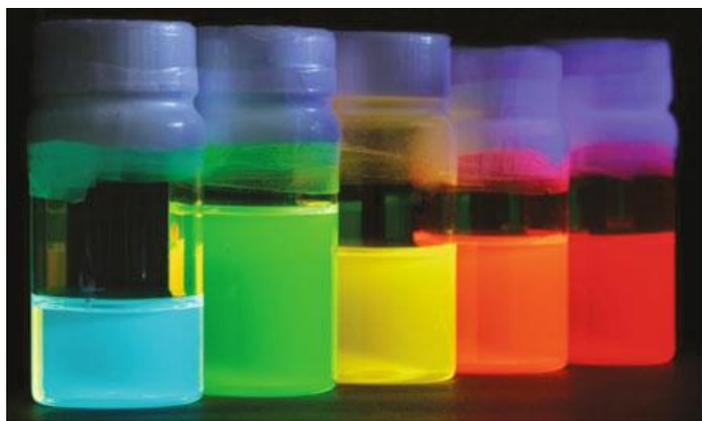
Figure 1.12: Effect of the size on the luminescence properties of CdSe quantum dots (1.7 to 4.5 nm) excited by UV light.<sup>50</sup>
