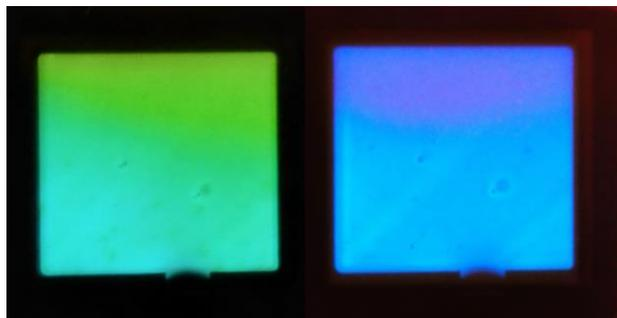
Figure 3.10: Colour gradient effects on blue OLEDs achieved by brush painting the fluorescein (left) and rhodamine (right) acrylic layers.
