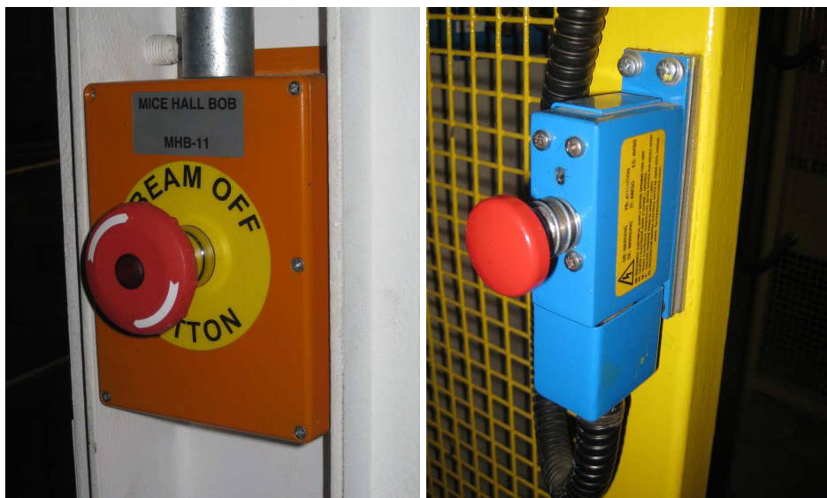
Figure 1.3: PPS “Beam-Off Button” (left) and door “Break-out” or “Crash-out” button (right); both are commonly referred to as “BOBs”.
