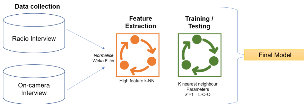
Figure 4.3. Preliminary data analysis indicating data collection, pre-processing, feature selection / extraction and k -NN parameters. F CV = 17-Fold Cross Validation; L-O-O = Leave-One-Out
