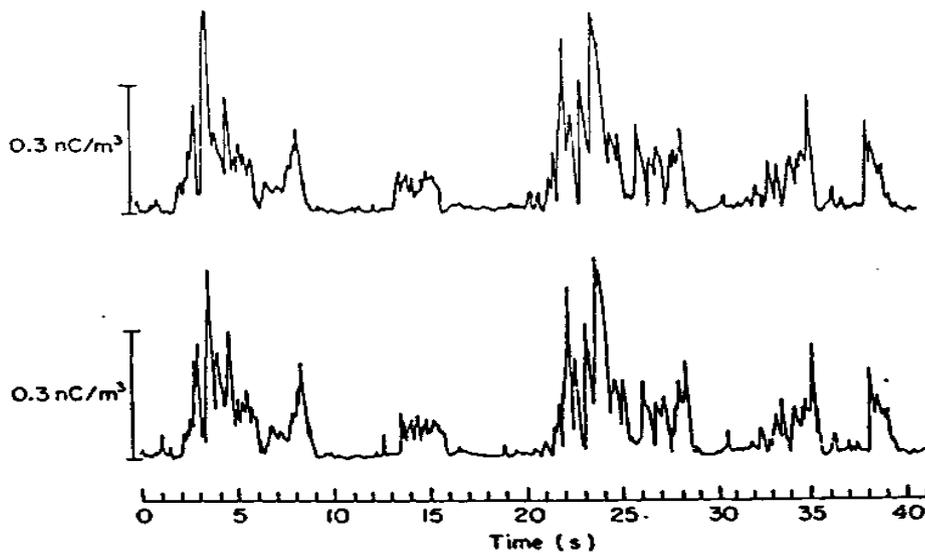
Figure 7. Simultaneous ion concentration measurements at vertically separated points. Upper trace, 1.5 m; low 1.45 m; ion collectors, 30 m downwind of a continuous point source of  $\sim 0.15 \mu A$  at 2.2 m height; wind spe 2-5 m/s; slightly unstable conditions, 22.8.75.
