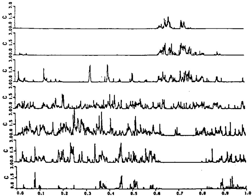
Fig. 2. An example of the signal which appears in the seven detectors in the cross-wind direction during one minute.
