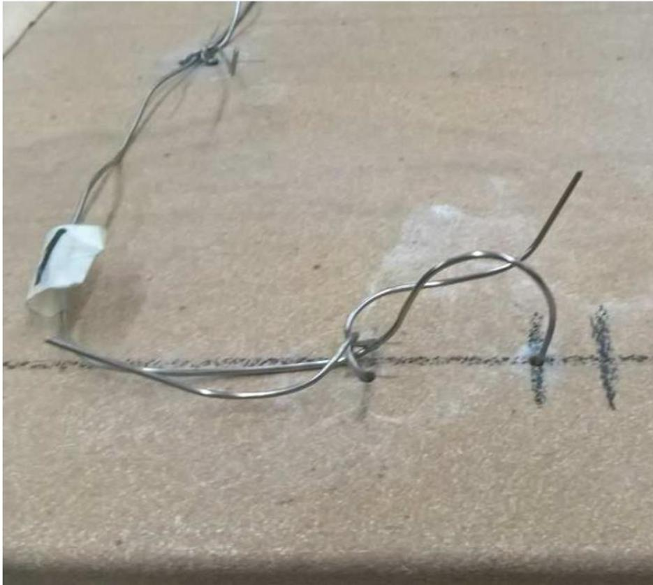
*Figure 35 Thermocouple distance from the tile*
