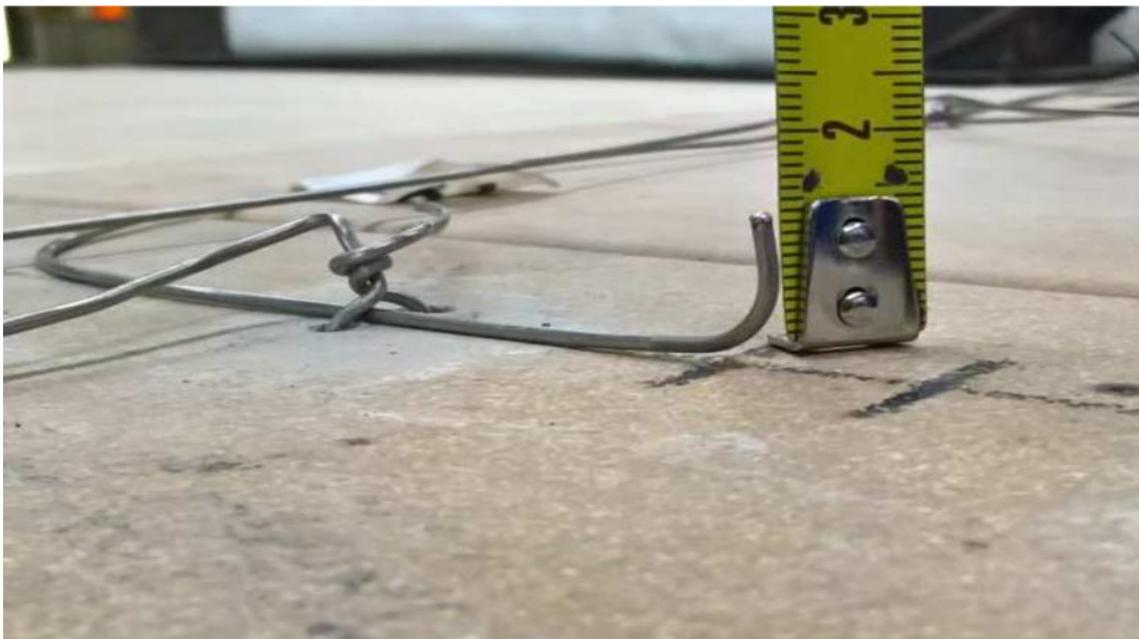
*Figure 36 Arrangement of the thermocouple on the tile*
