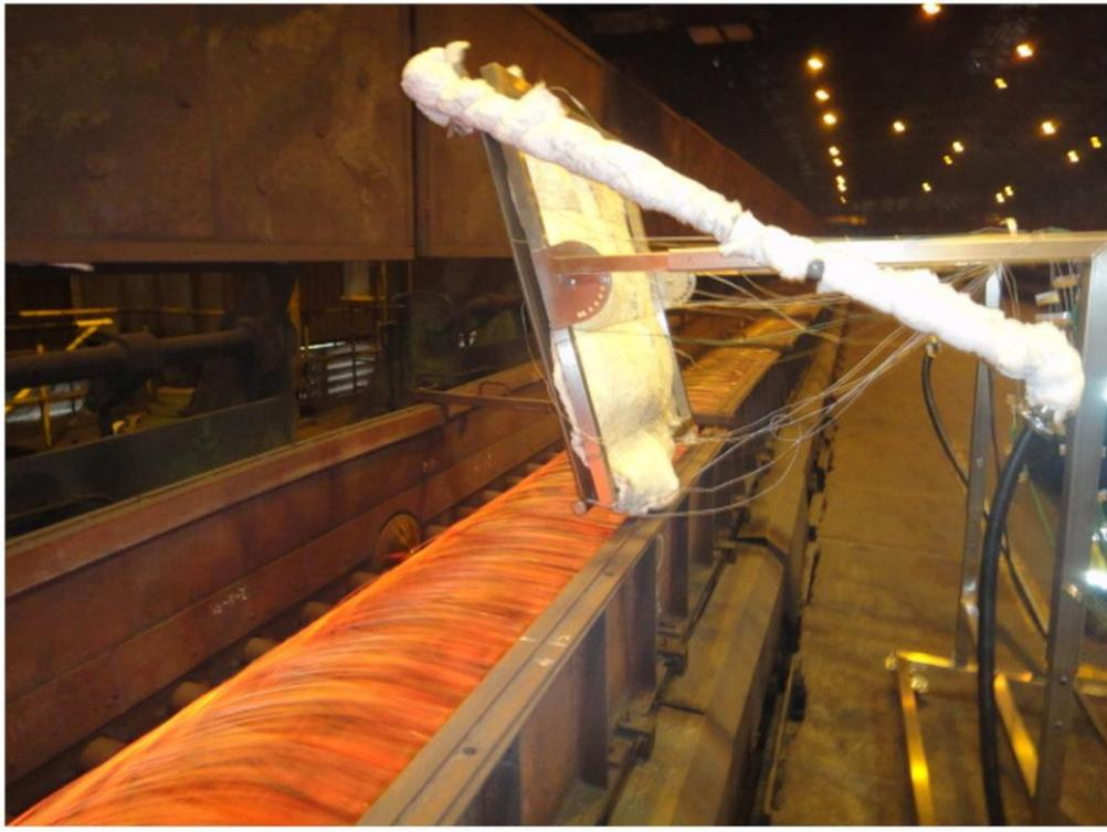
*Figure 29 Flat Heat Pipe on cooling line*
