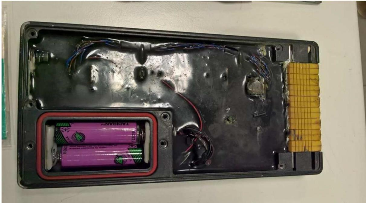
Figure 39 State of the Datapaq after the test
