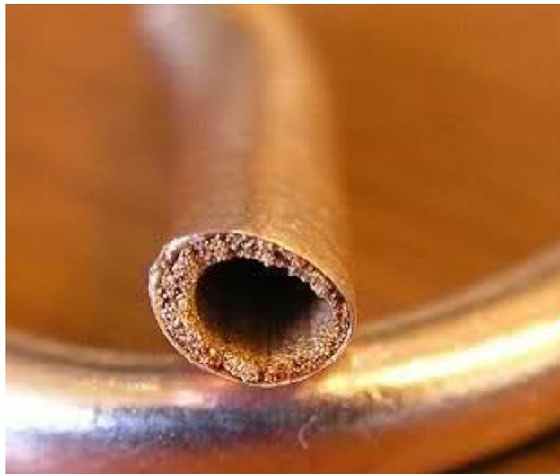
*Figure 25 Cut view sintered heat pipe*
