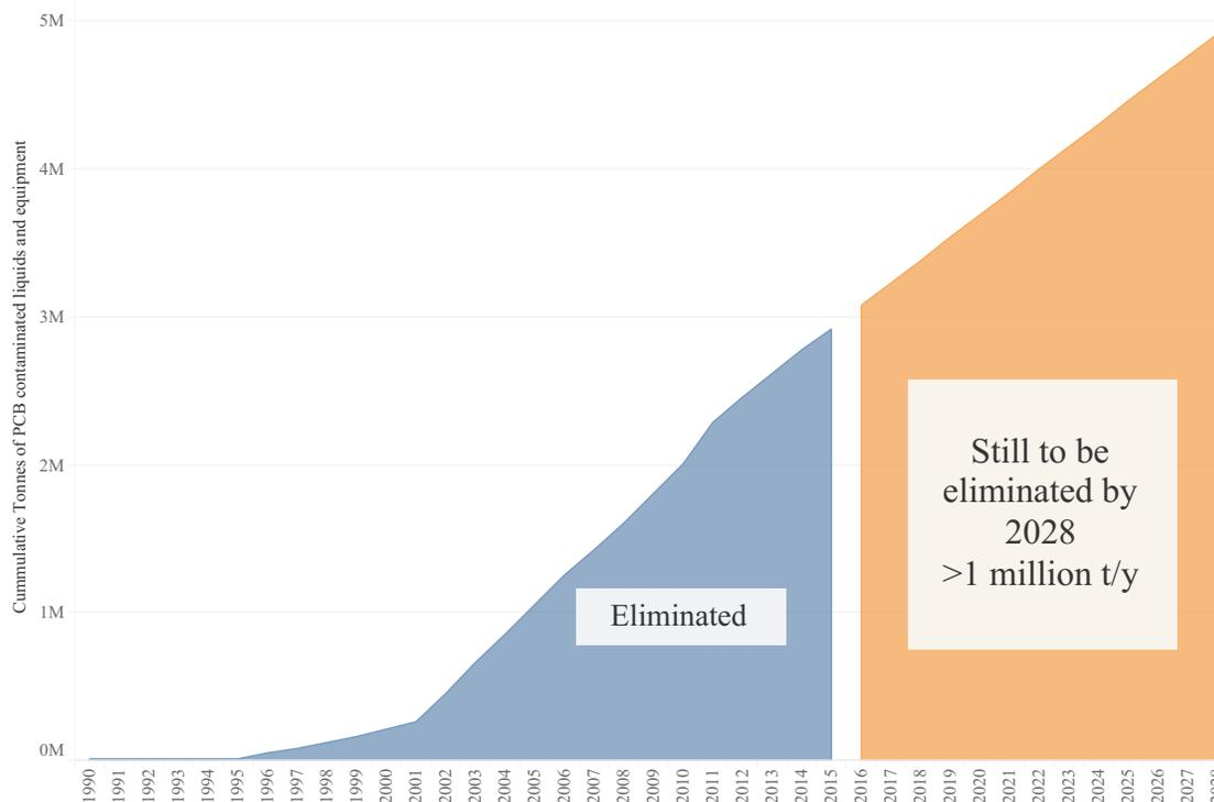
Figure 1-1: Cumulative tonnes of PCB contaminated liquids and equipment that have been eliminated up to 2015 (blue area), estimated amount that must be eliminated to meet 2028 Stockholm Convention target (orange area). Estimates are based on data from (UNEP/DTIE, 2016).
