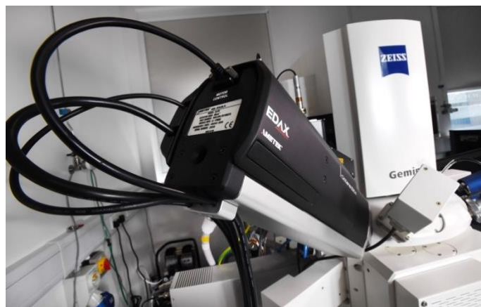
Figure 3.6 – X-Ray detector attached to SEM apparatus used for EDAX
