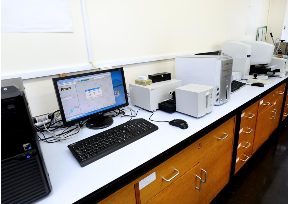
Figure 3.15 – Hewlett Packard UV-Vis spectrophotometer used to determine methylene blue and tetracycline concentration in solution
