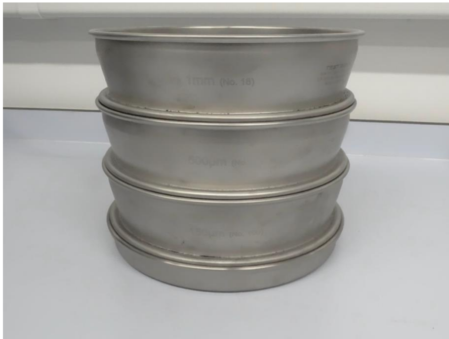
Figure 3.5 – Sieves used to ensure biochar particle sizes ranged between 1mm and 0.15mm
