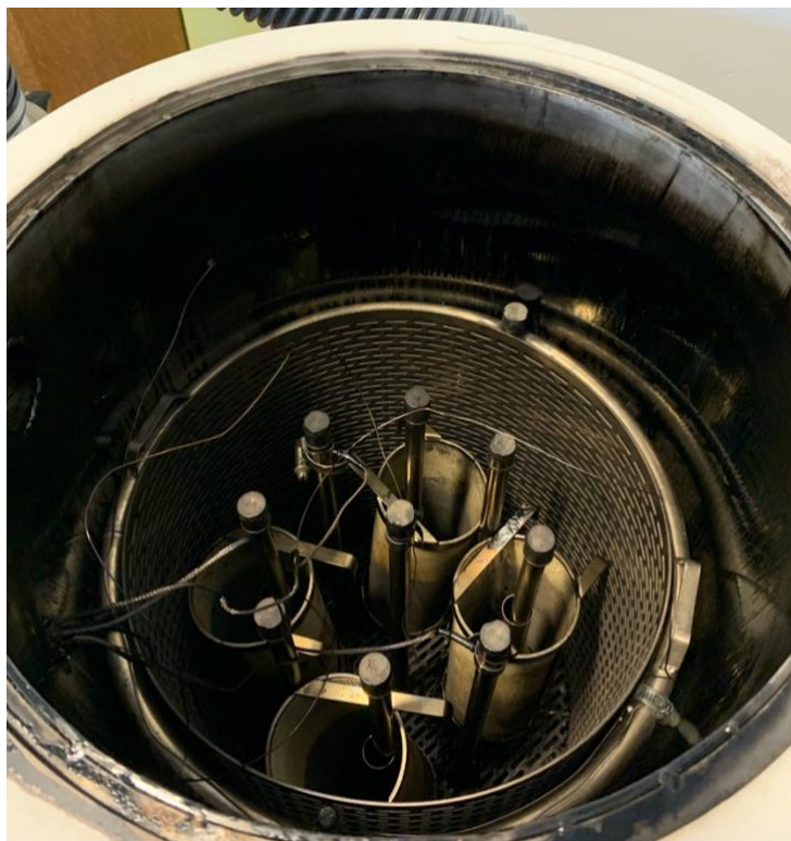
Figure 3.3 – Internal image of heat pipe reactor, with small mesh baskets for pyrolysis of fine material
