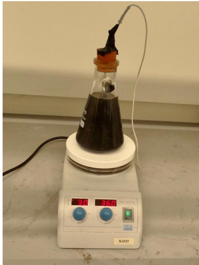
Figure 3.14 – Altered experimental set-up for methylene blue and later tetracycline experiments
