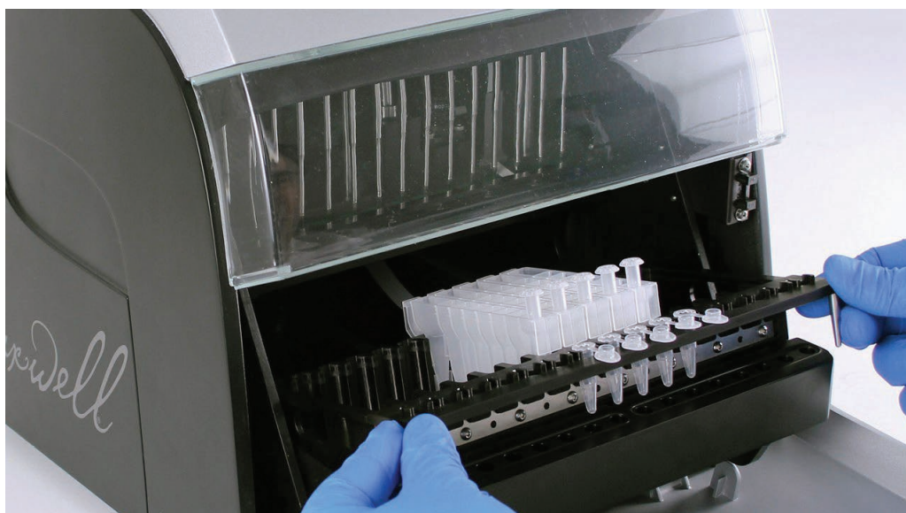
FIGURE 2.3: Maxwell RSC instrument containing several cartridge samples for purification.
