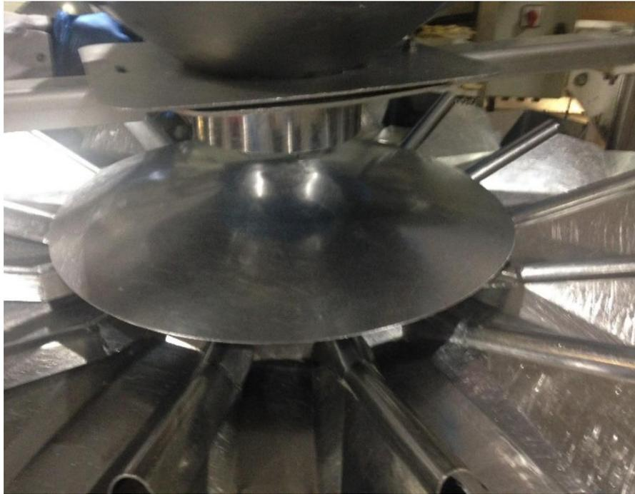
Figure 6.13 Top cover above lower feeders
