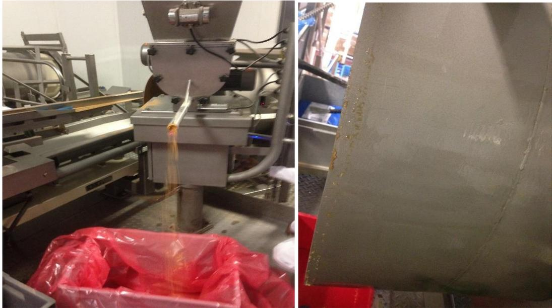
Figure 6.36(a) Flavour mixer drain to bin bag. (b) outside side of flavour mixer with flavour deposit on the surface
