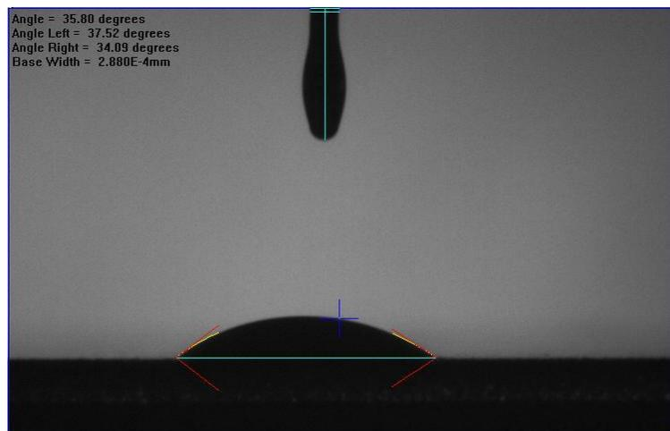
Figure 4.31 Contact angles with cooking oil
