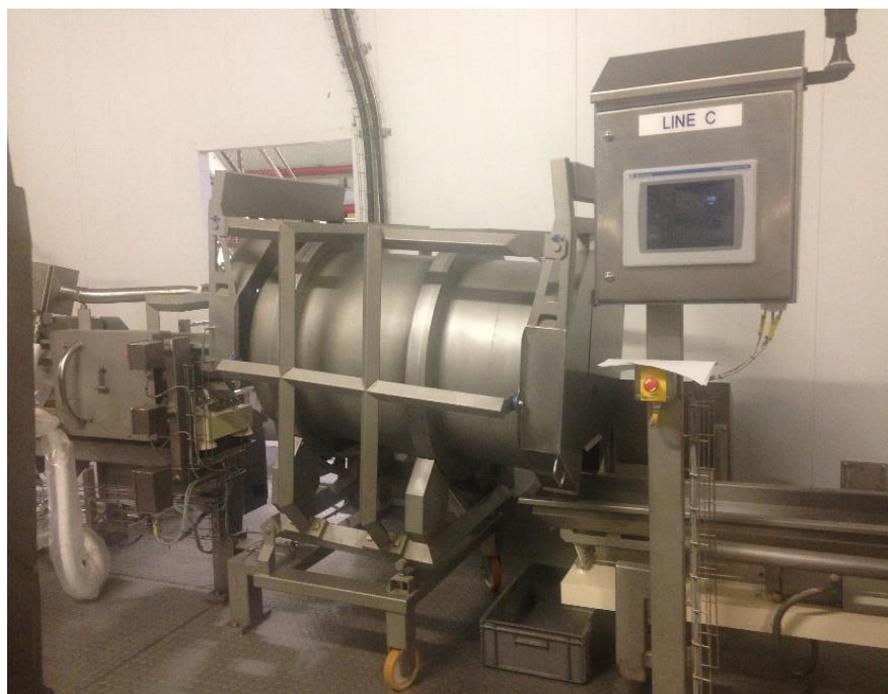
Figure 6.33 Flavour mixer drum on the production line
