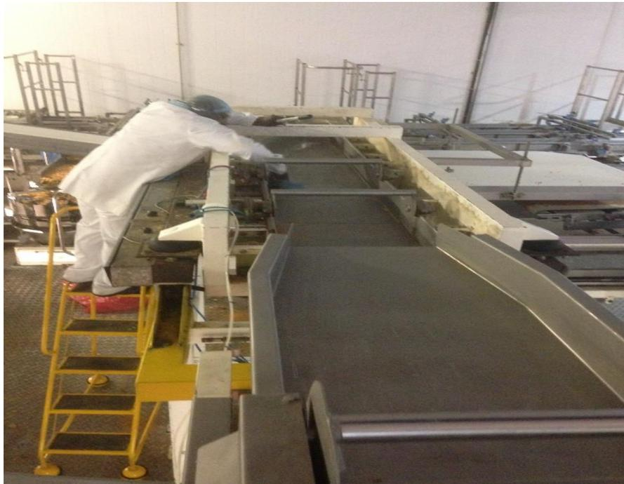
Figure 6.29 Metal vibrating conveyor
