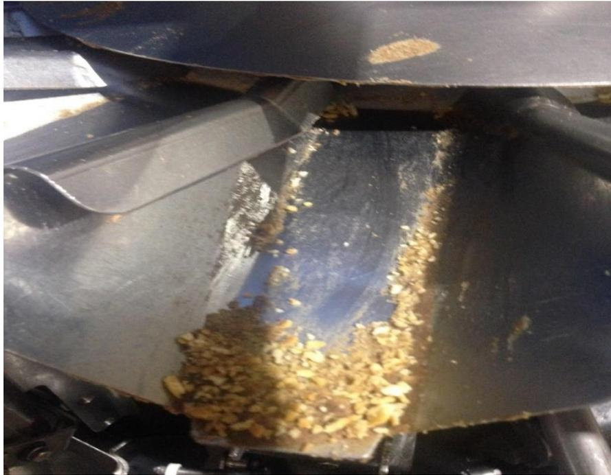
Figure 6.15 Feeder with flavour and crisps particles
