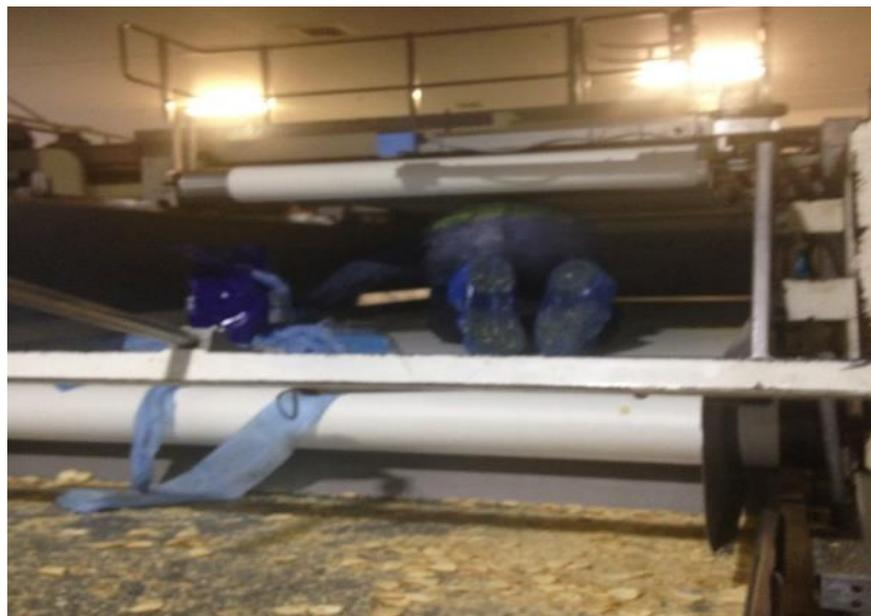
Figure 4.15 Storage conveyor cleaning process with narrow place to clean from inside
