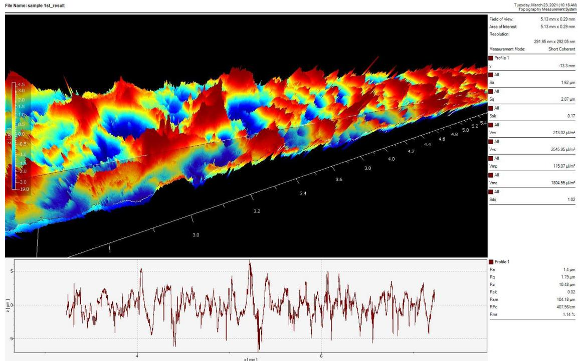
Figure 4.27 Sample surface texture with oil coating
