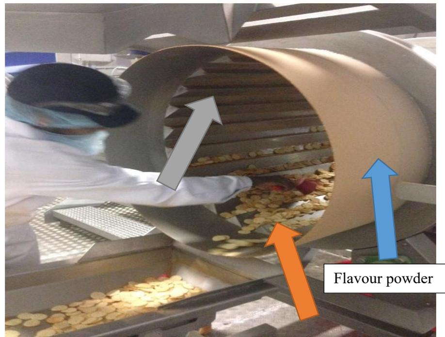
Figure 4.17 Flavour mixer drum manual cleaning process from inside
