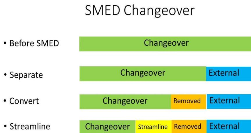
Figure 2.14 Single minute exchange die description
