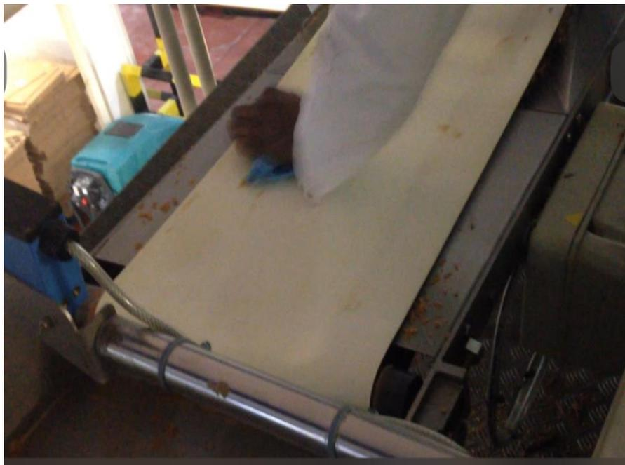
Figure 4.13 Manual cleaning of soft conveyor with wipes
