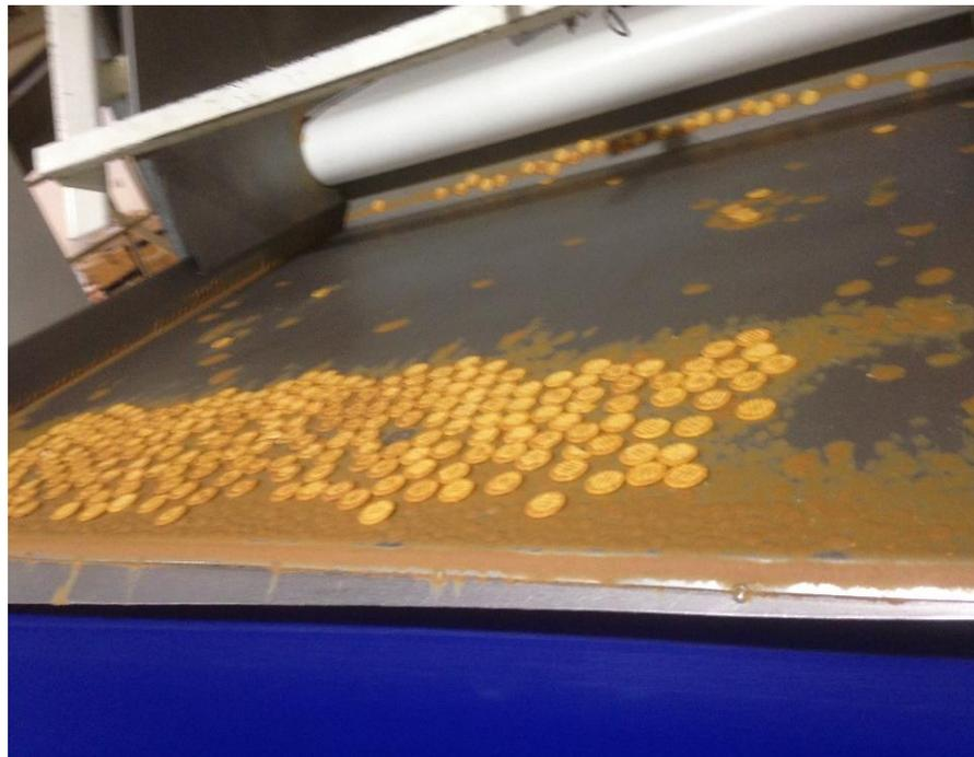
Figure 6.24 Lower portion of storage conveyor with flavour particles
