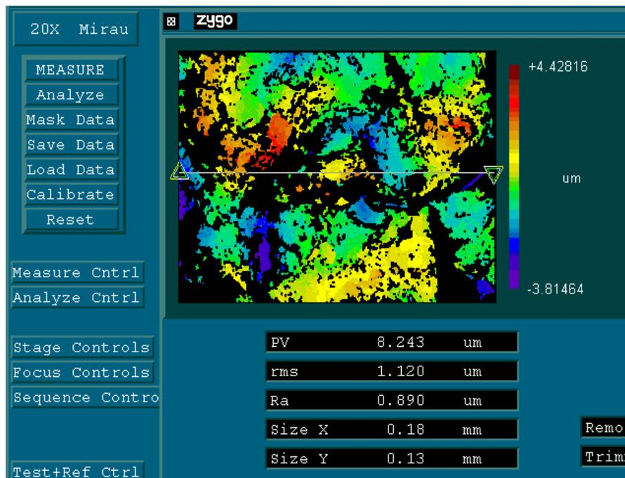
Figure 3.4 3D surface texture measurements
