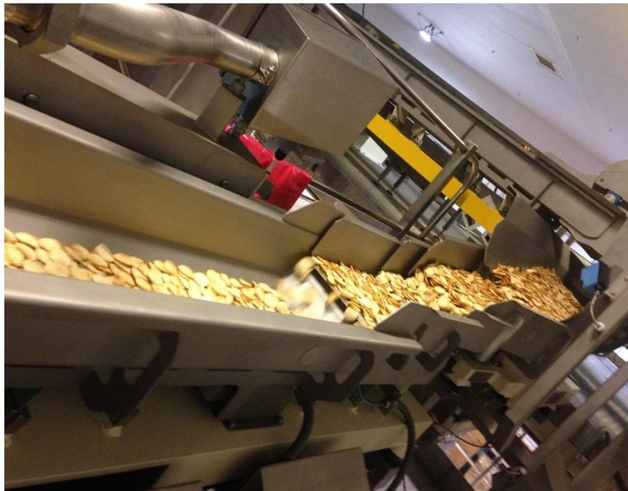
Figure 6.6 Vibrating metal conveyor towards oil drums
