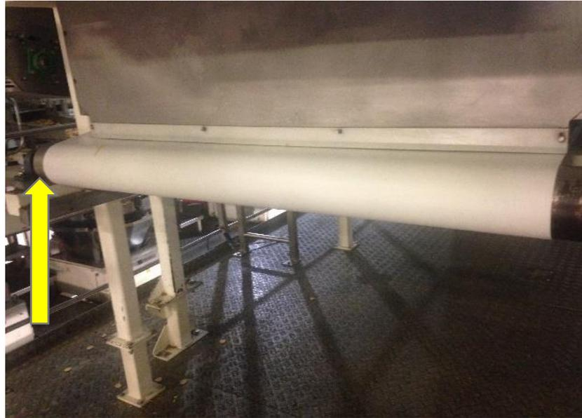
Figure 4.16 Proposed location where fixed cleaning brush can be Mounted to clean soft fabric conveyor during operation
