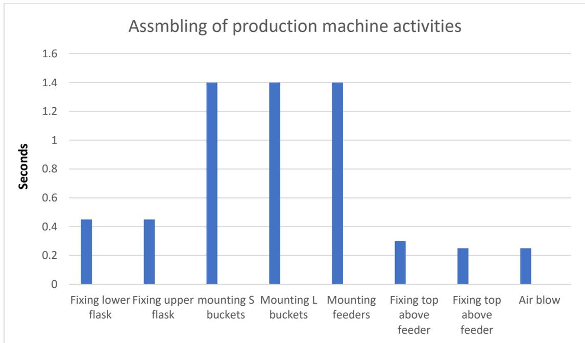
Figure 6.22 Assembling of production machine activities
