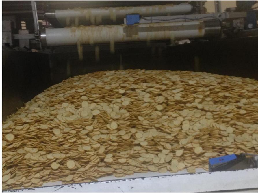
Figure 4.14 Storage vibrating metal conveyor while in operation
