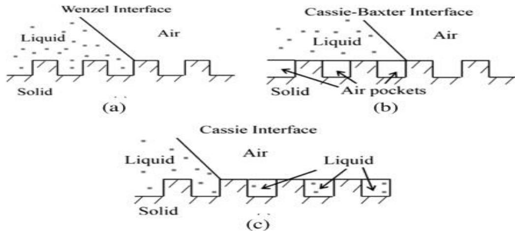
Figure 5.13 Air pockets on the surface [103]
