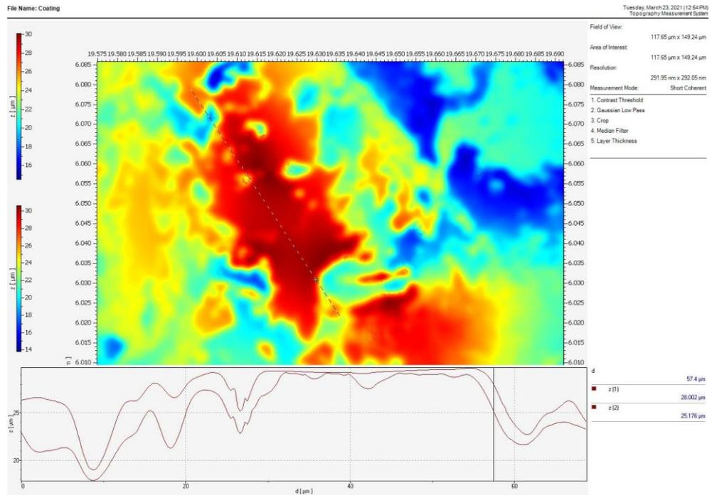
Figure 4.28 Sample surface with oil coating thickness
