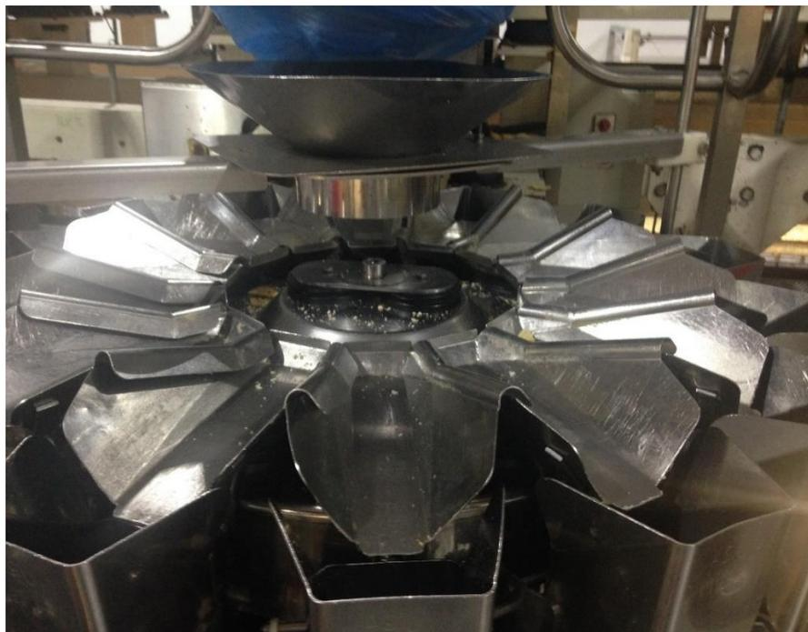
Figure 6.14 Fourteen feeders to feed crisps to the large buckets
