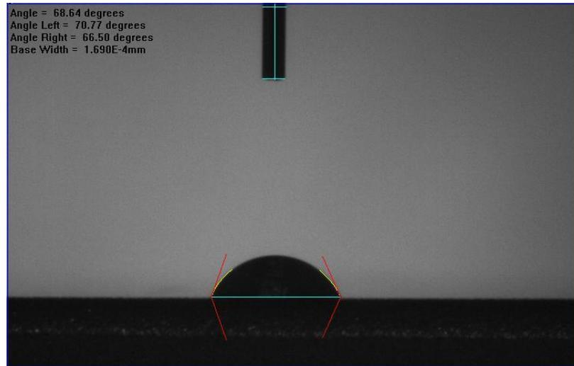
Figure. 4.30 Contact angle of the surface with water
