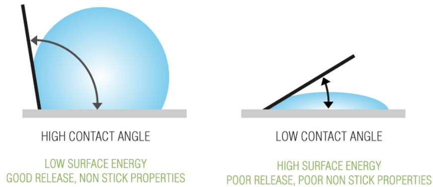
Figure 5.14 Proposed contact angle on proposed surface with low surface energy [100]
