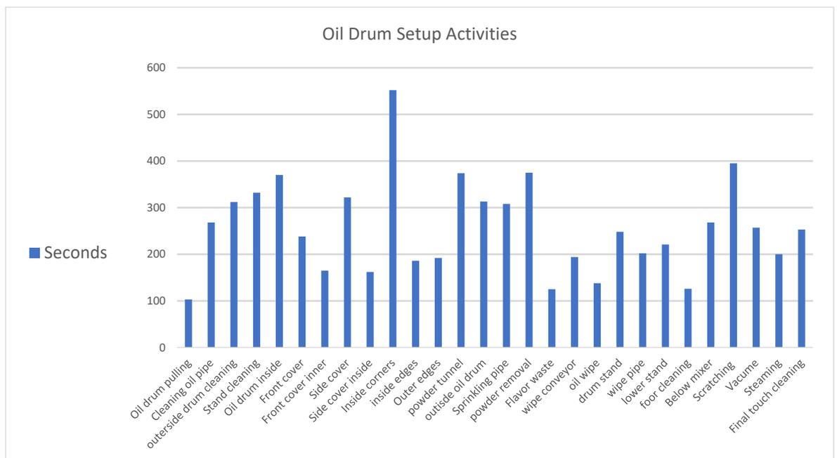
Figure 4.4 Activities in oil mixer drum setup and cleaning
