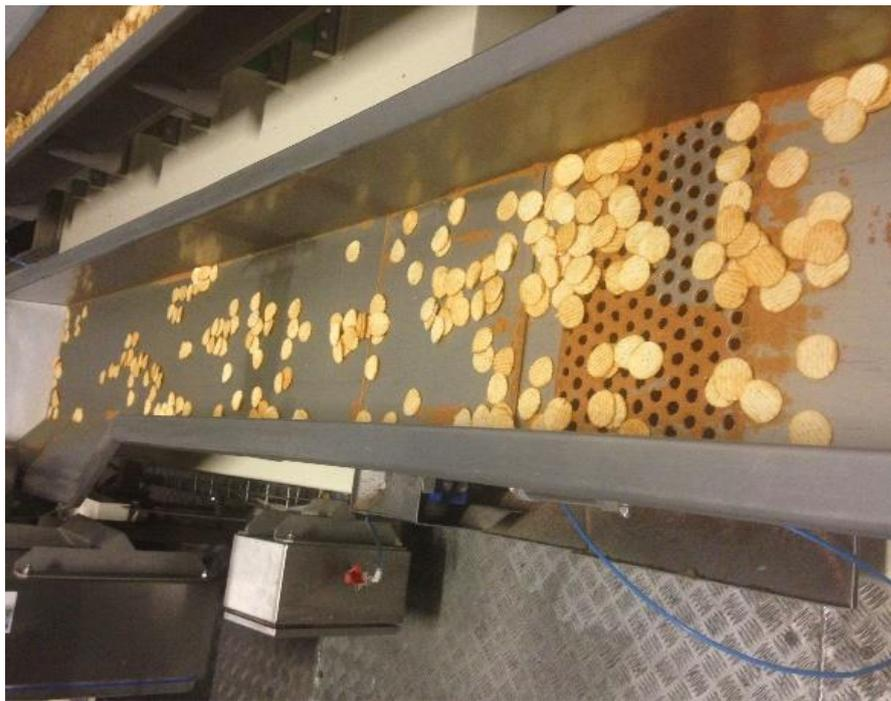
Figure 6.43 Cleaning a metal conveyor
