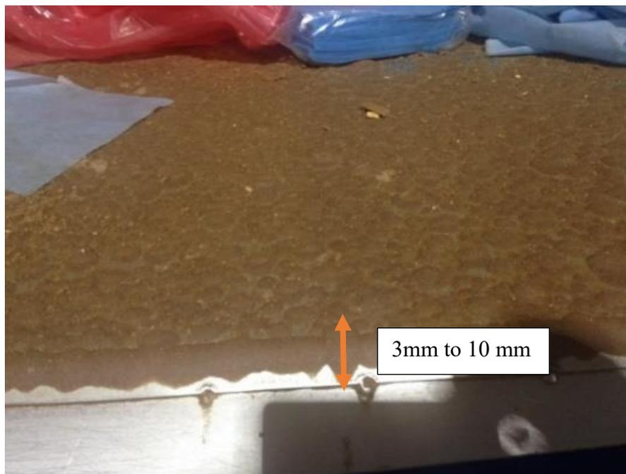
Figure 1.4 Thick material sticks on the storage conveyor surface
