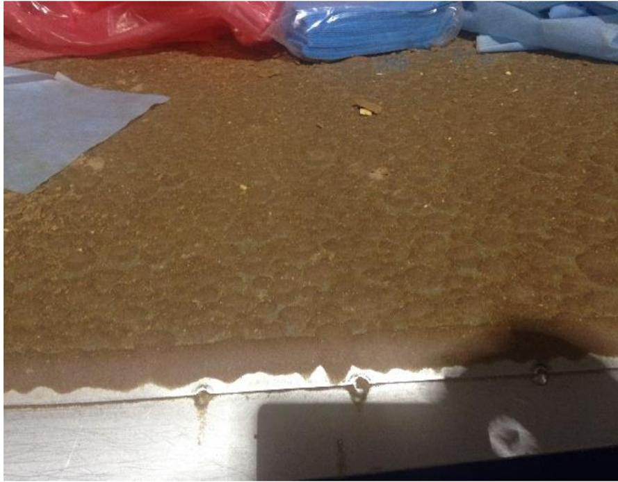
Figure 6.42 Thick material stuck to a metal conveyor
