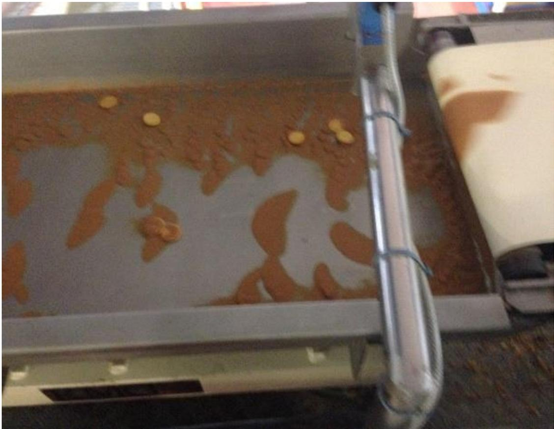
Figure 6.39 Metal vibrating conveyors before cleaning
