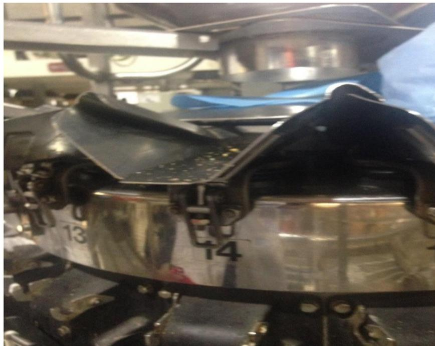
Figure 6.20 Buckets mounting location
