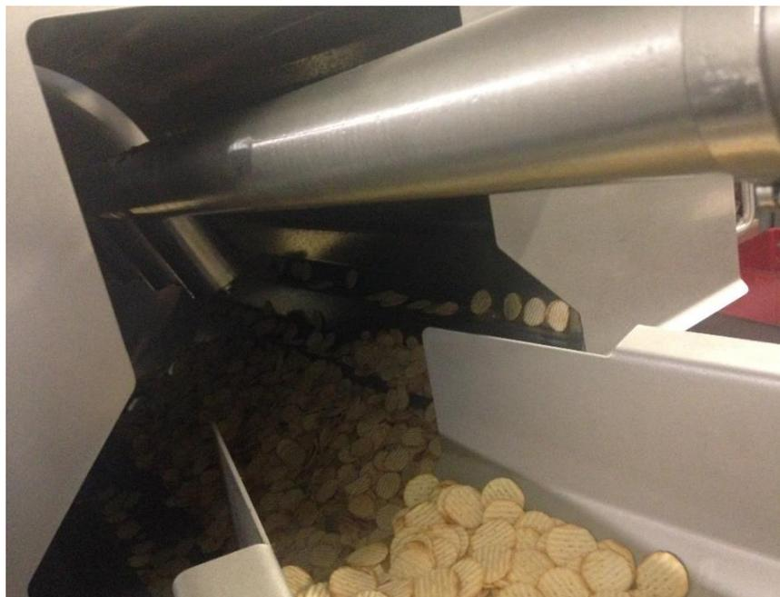
Figure 6.32 Oil sprinkle pipe inside oil drum
