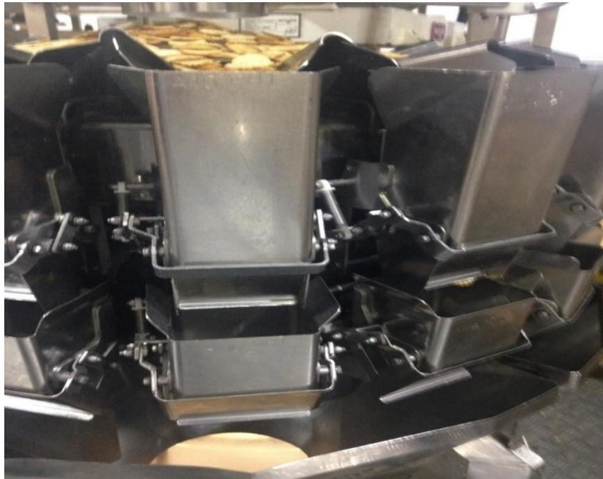
Figure 6.16 Buckets of production machine
