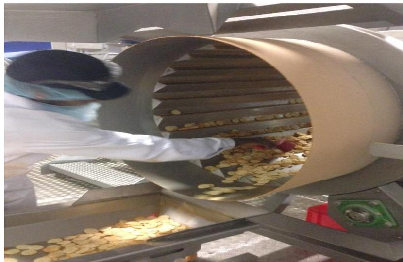
Figure 6.35 Manual removal of crisps from flavour mixer
