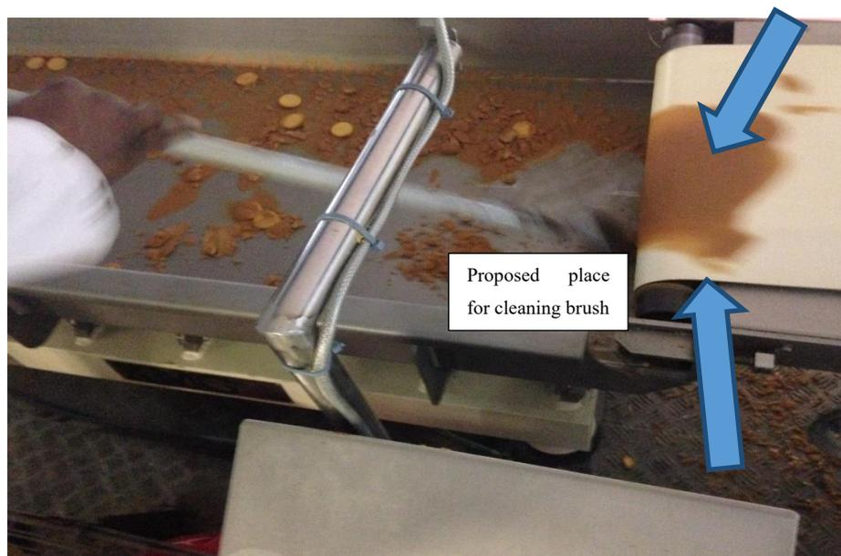
Figure 5.3 Soft conveyor belt with flavour material on it
