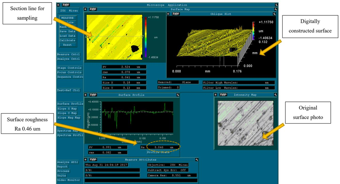
Figure 6.49 Smooth surface roughness 0.046um
