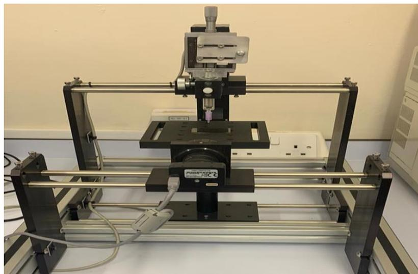
Figure 4.29 Instrument for contact angle measurements
