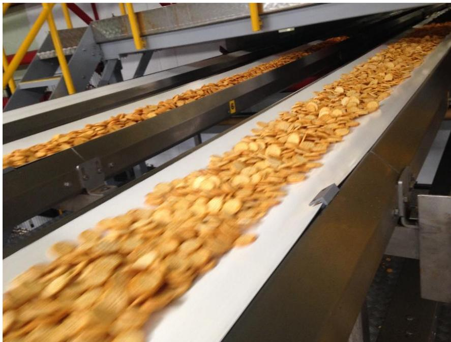
Figure 6.2 Soft conveyor belt transporting crisps from oven
