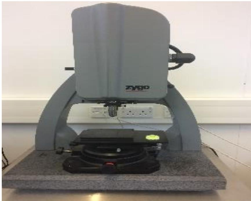
Figure 3.8 Zygo equipment for 3D surface roughness measurements
