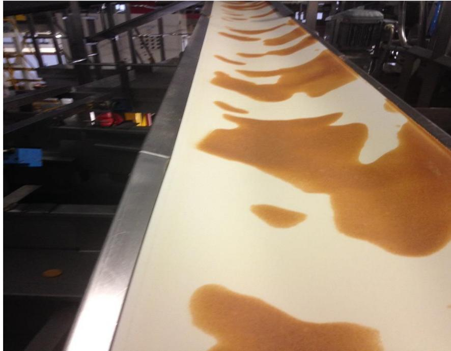
Figure 6.28 Soft conveyor belt transporting crisps from oven to storage conveyor
