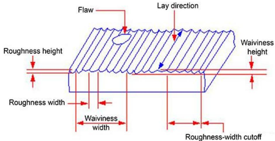
Figure 3.2 Example of machined surface [88]
