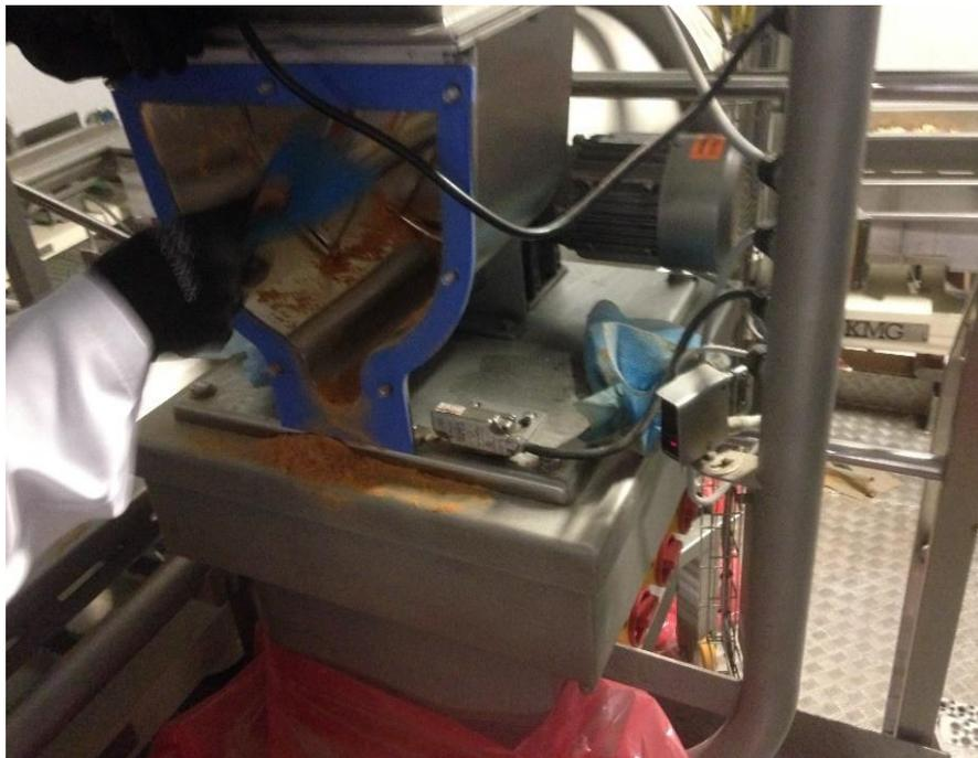
Figure 6.51 Tools used to clean flavour tank manually
