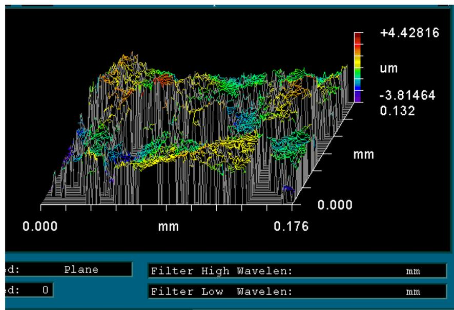
Figure 3.6 3D surface waviness diagram
