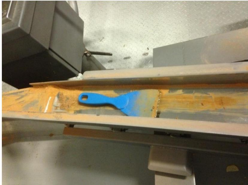
Figure 6.50 Tools used to clean narrow size flavour feeder
