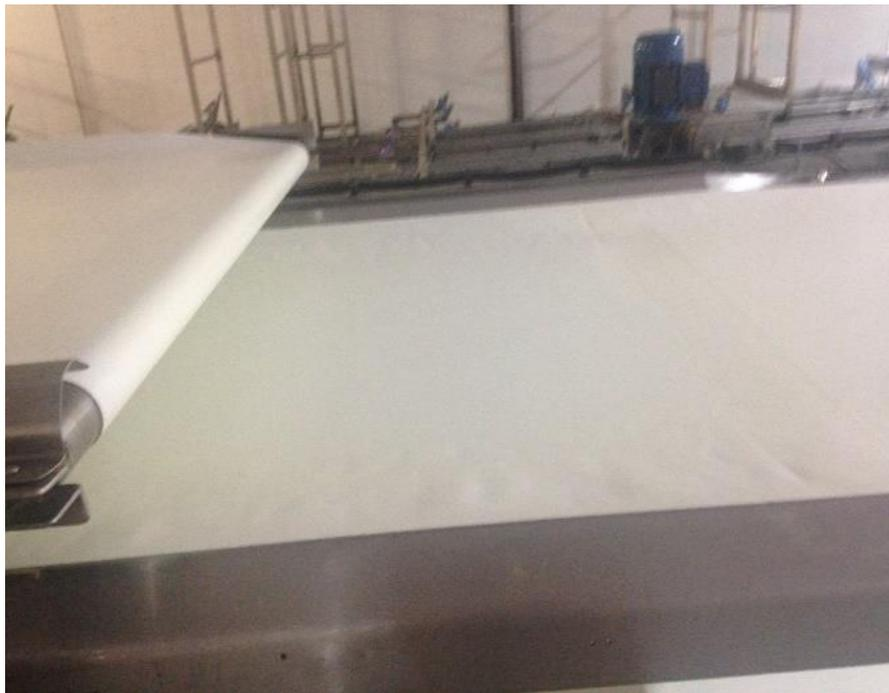
Figure 6.27 Upper side of storage soft conveyor after cleaning
