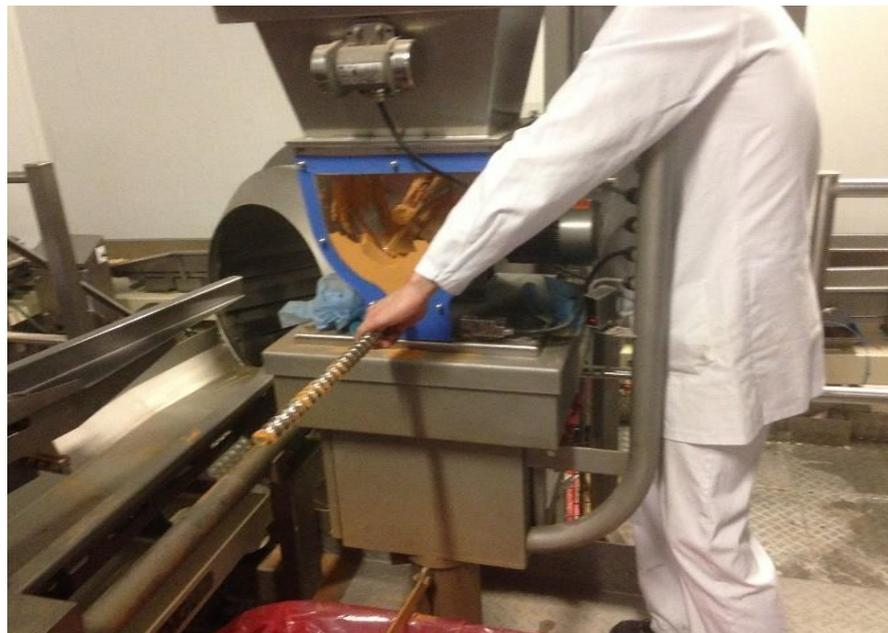
Figure 4.18 Flavour tank and its internal parts manual cleaning process
