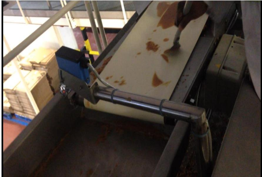
Figure 4.12 Manual removal of debris from conveyor
