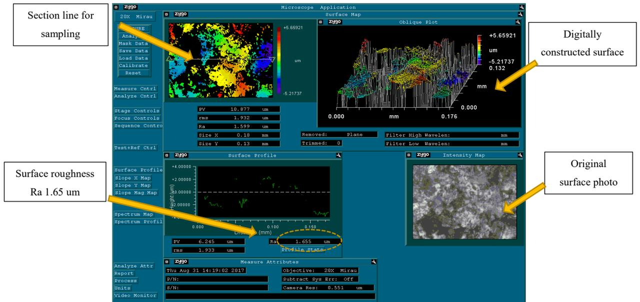
Figure 6.48 Surface roughness is 1.65 um of the existing Metal sample used in the company
