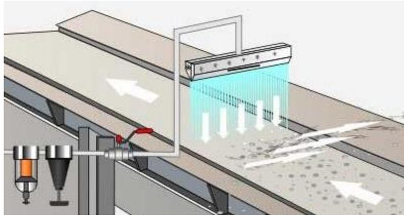
Figure 5.4 Air pressure applied to the surface [154]
