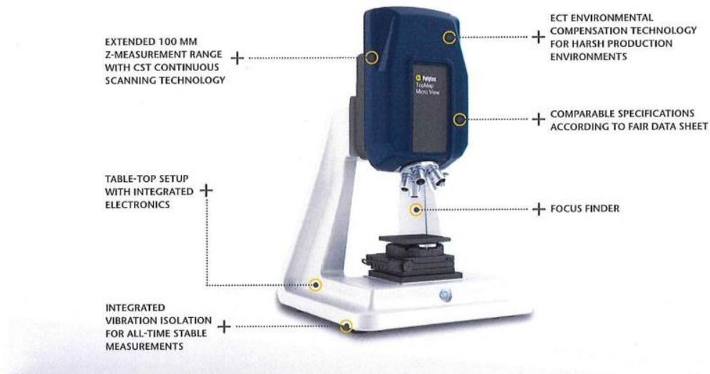
TopMap Micro.View® is an easy to use and compact optical profiler. Combine exceptional performance and affordability with this powerful metrology solution. An extended 100 mm Z-measurement range with CST Continuous Scanning Technology allows complex topographies to be measured at nm resolution. This convenient table-top setup features integrated electronics, with the smart focus finder simplifying and speeding up the measurement procedure.
