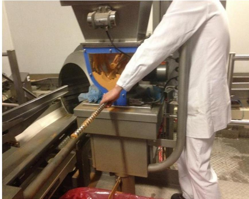
Figure 6.37 Disassembling of flavour tank
