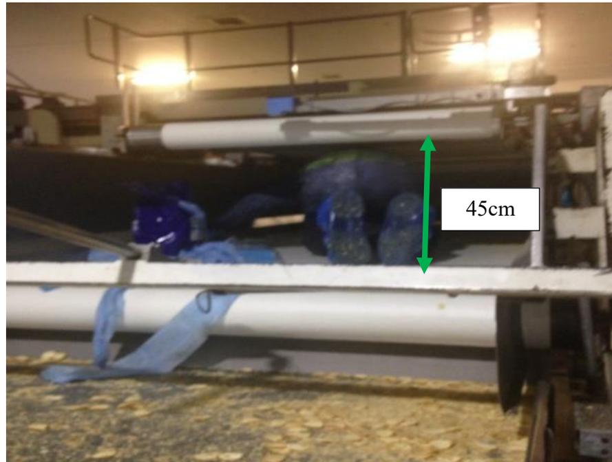
Figure 1.5 Photograph highlighting limited access during cleaning
