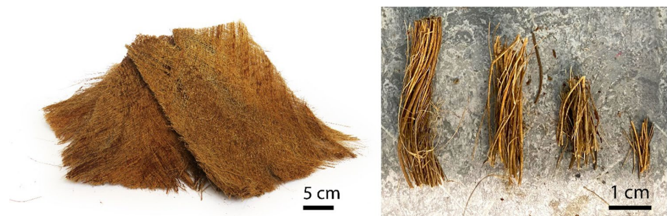
Fig. 1 DPF leaf sheath after cleaning (left) and DPF cut into different length (right)
