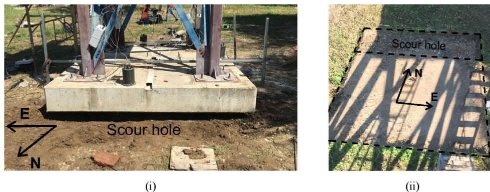
Fig. 5 i Excavation of the soil under the foundation, ii scour hole shape at the end of the final test
