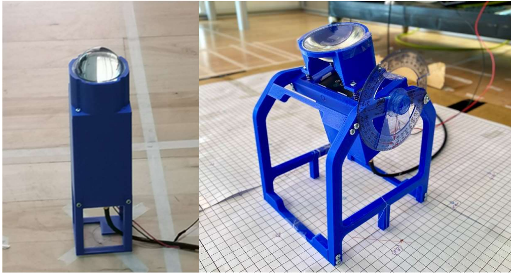
Figure 3.2 – (Left) Upright IoRL VLC receiver casing. (Right) IoRL Receiver Gimbal mounted with VLC receiver and convex lens
