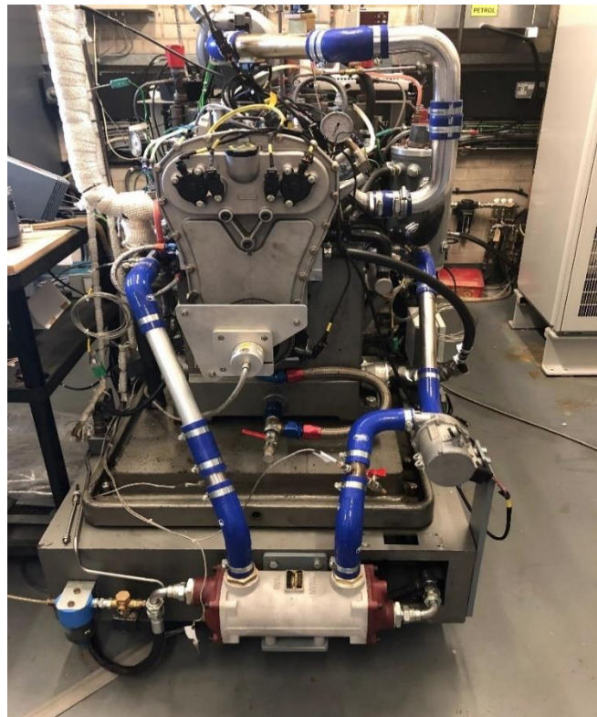
Figure 3-2 Brunel-MAHLE Single Cylinder DISI Engine on the testbed
