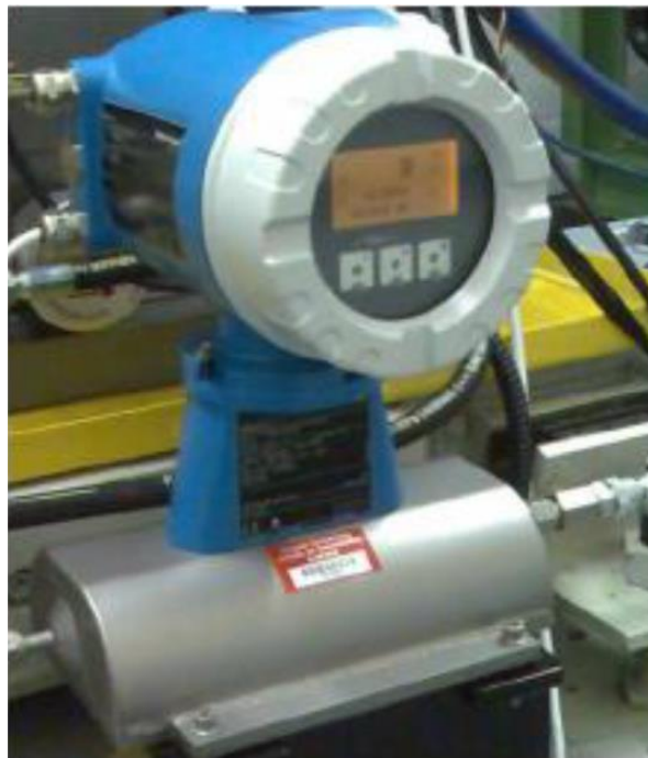
Figure 3-5 Coriolis mass flow meter by Endress+Hauser
