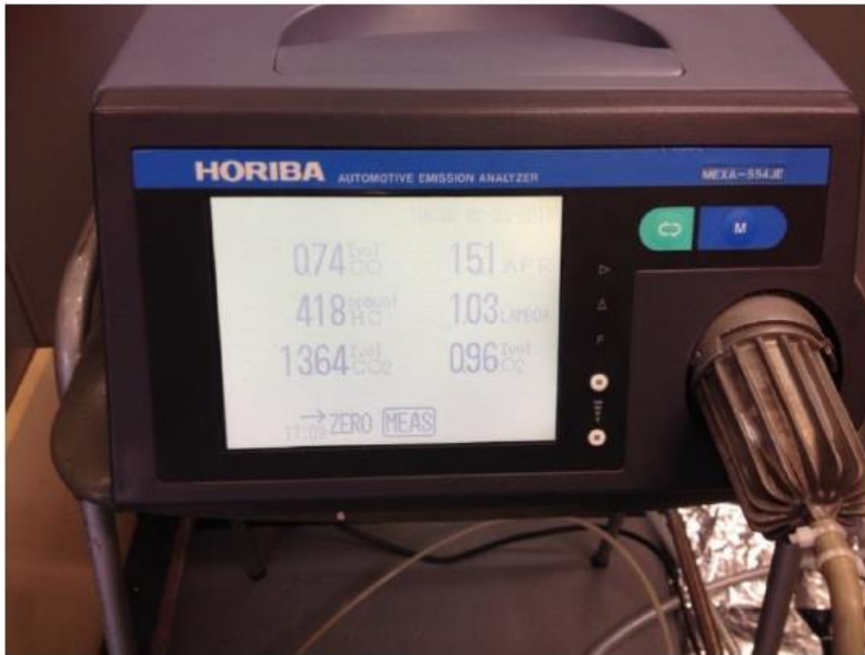
Figure 3-18 Horiba MEXA-554JE for CO, CO 2 , and O 2 measurements
