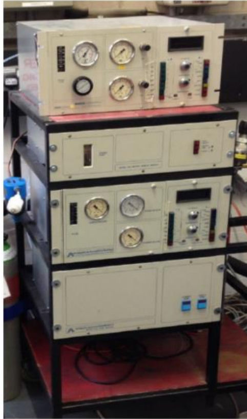
Figure 3-19 Signal Rotork Analysis model 523 FID analyser used for HC measurements (first unit at the top) and Signal Ambitech model 443 Chemiluminescent analysers used for NO/NOx measurements (bottom 3 units)
