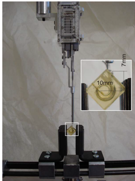
Fig. 2.14 Automated insertion tool setup with integrated force sensing unit. Figure from [27]
