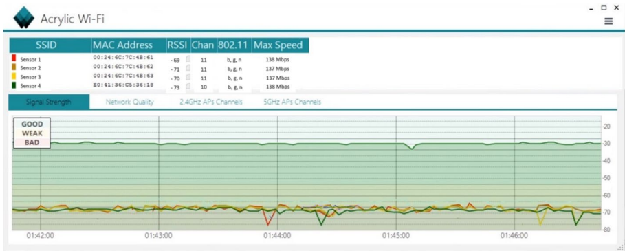
Fig. 16 RSSI and signal coverage levels after Stackelberg
