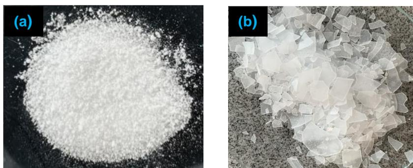
Figure 3. 2 Appearance of (a) PEG8000; and (b) PEG4000 at room temperature.
