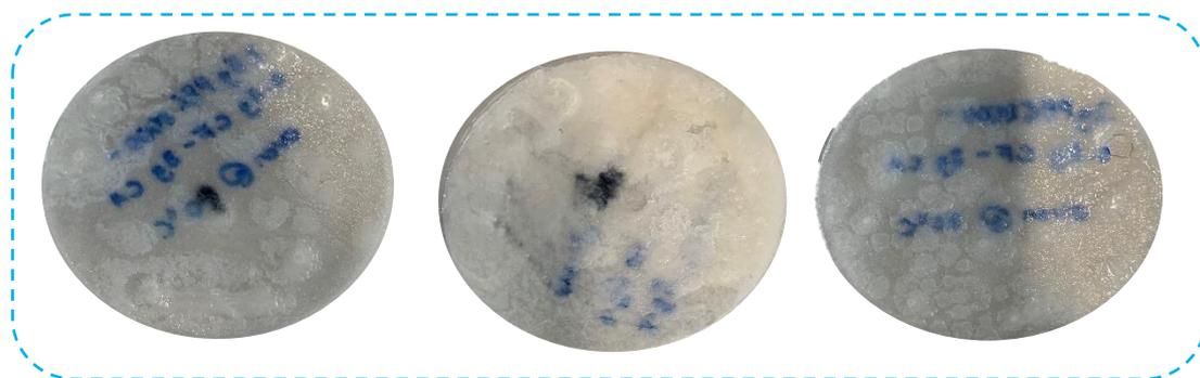
Figure 4. 1 Appearance of TCA samples cured at 50 °C for 24h.
