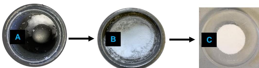
Figure 3. 21 (A) Metal jar containing ball and solid sample pieces; (B) Powder sample; and (C) XRD sample holder containing test sample.
