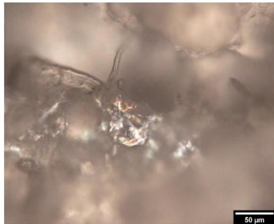
Figure 6. 17 Close-up view of the crystal morphology of the TCA crosslinked composite PCM.
