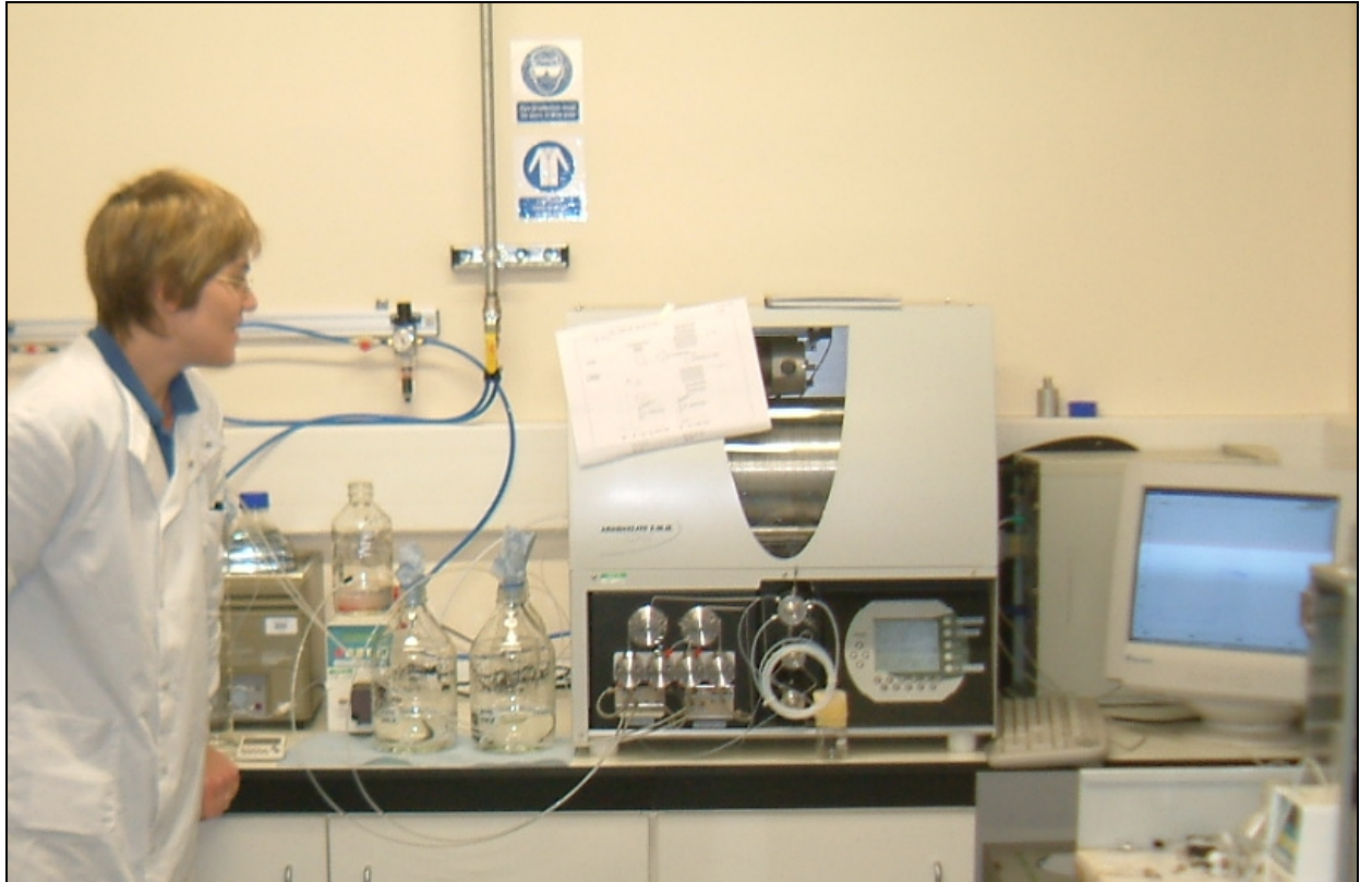
Figure 1: The 1 litre Centrifugal Partition Chromatography set up in the Advanced Bioprocessing Centre at Brunel Institute for Bioengineering, Uxbridge, UK
