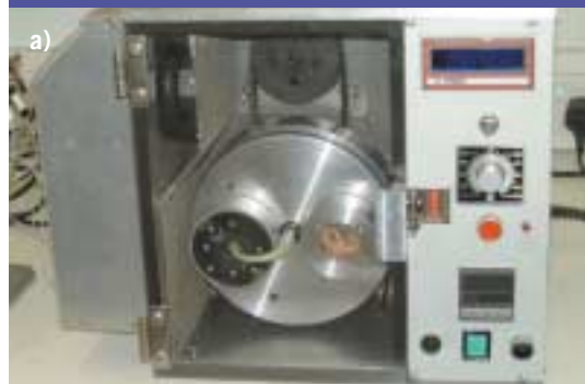
Figure 4: a) the Mini-DE (5-17ml capacity, mg scale, W35xH35xD42cm); b) the Midi-DE (0.1-1.2 litre, g scale, W65xH51xD170cm); and c) the Maxi-DE (5-15 litre, kg scale, W150xH190xD170cm)
