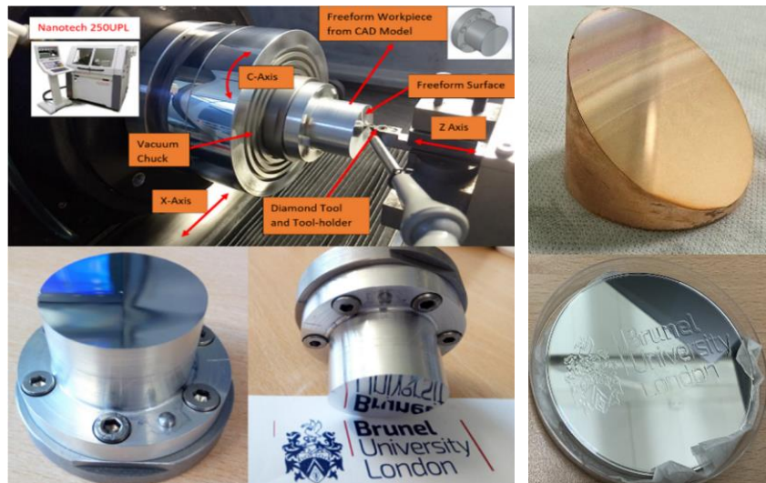
Figure 6.16 Freeform surfaced components ultraprecision machined at the diamond turning machine with further support of digital twin approach.
