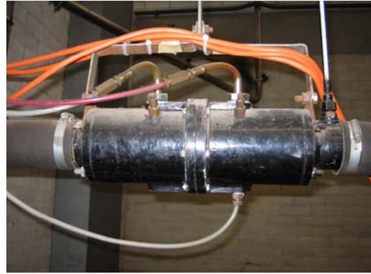
Orifice measurement part of a manometer
