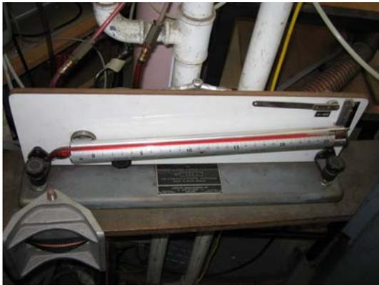
Reading meter of a manometer
