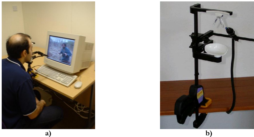
Figure 3.4: a) Power Mac G3 (9.2) ViewPoint EyeTracker, used in combination with QuickClamp Hardware b).
