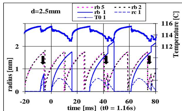
Figure 5: Radius and temperature distributions for  $d=2.5$ mm
