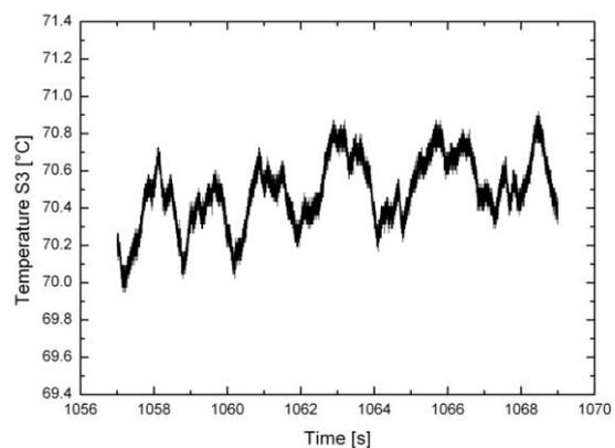
**Figure 13:** Fluctuating temperature under cavity 3 at  $16.6\ \text{kW/m}^2$
