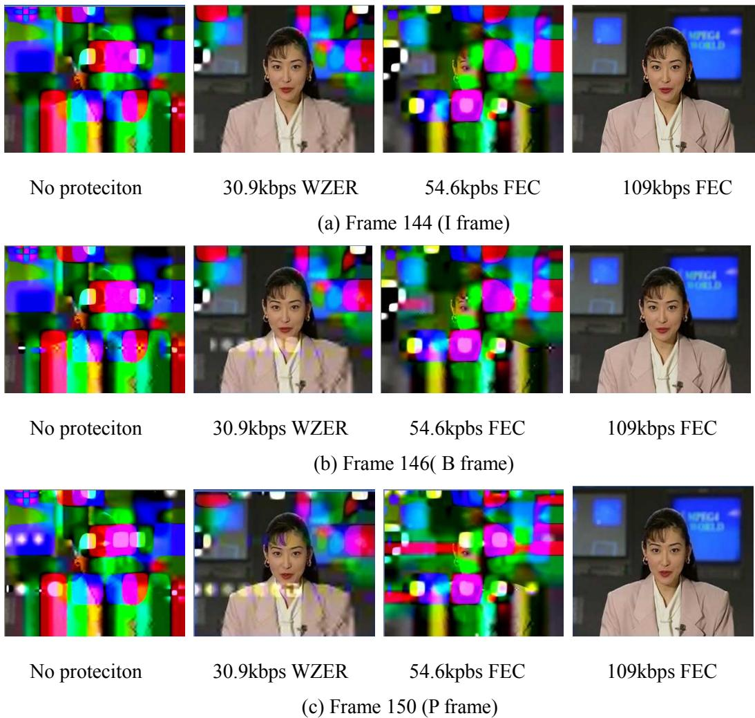
**Fig.5. 10 Perceptual comparison of I, B, P frames with WZER of Akiyo sequence**
