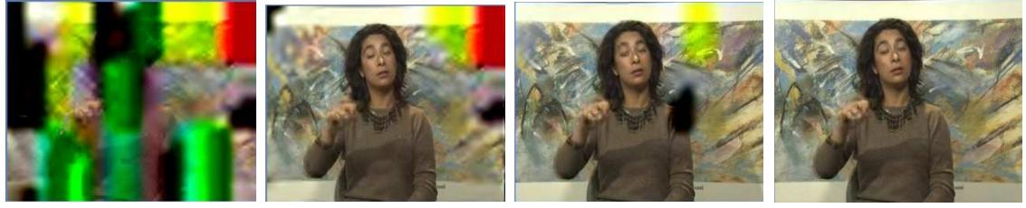
(i)No protection (ii)38.3kbps WZ stream (iii)61.6kbps full FEC (iv)123.2kbps full FEC
