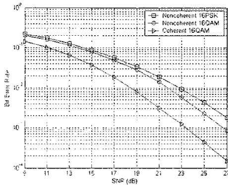
Fig. 2 Performance curves for one receive antenna.
