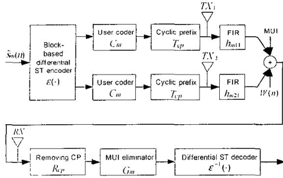
Fig. 1. Block diagram of DASTBC-OFDMA system
