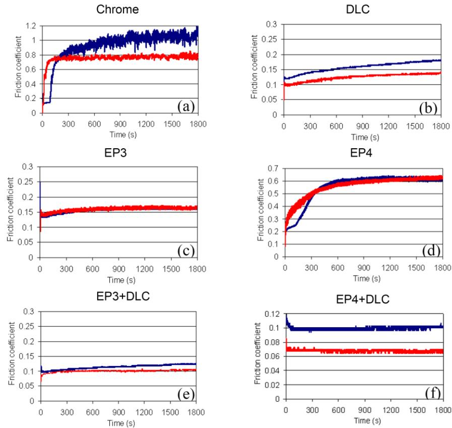
Fig. 4. (left) Comparison of friction coefficients vs. time, displaying results of two tests per condition for (a) chrome plating (b) DLC deposited directly on high strength steel substrate (c) EP3 epoxy, (d) EP4 epoxy, (e) EP3-DLC combination coating and (f) EP4-DLC combination coating.
