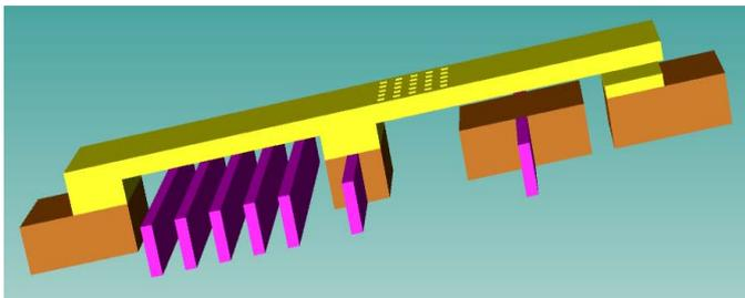
Fig.2. The proposed ohmic RF MEMS Switch.
