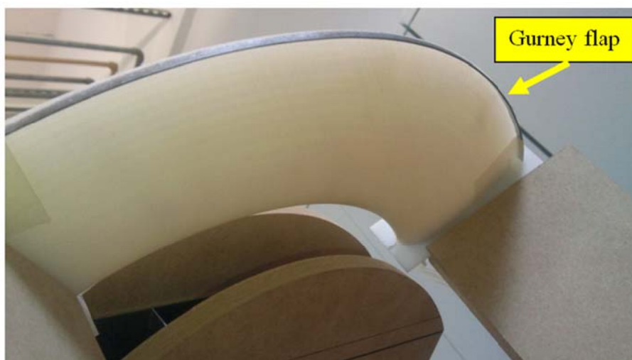
Figure 88: Depiction of arc-wing (NACA-0024) with Gurney flap attached to the lower surface.
