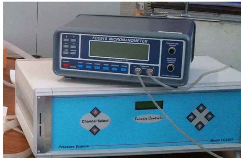
Figure 26: A photograph of pressure scanner and micro-manometer used in the experiments.
