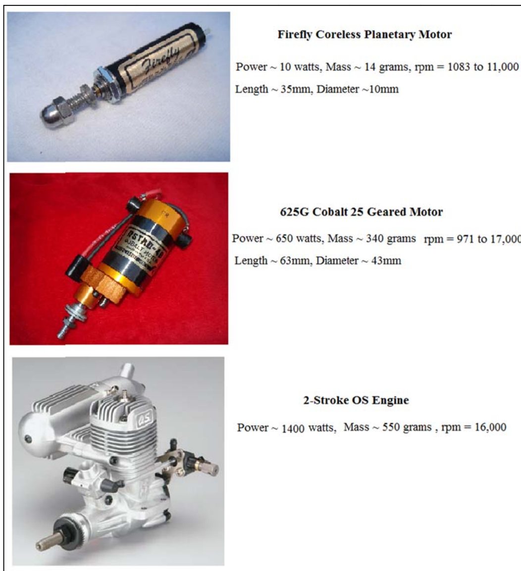
Figure 125: Common torque generator systems for micro/miniature vehicles {data source Ref [131]}.
