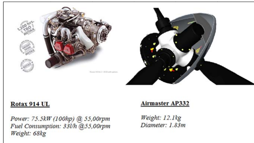
Figure 133: Engine and Propeller specifications [137].
