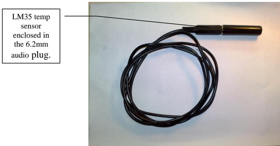
**Figure 4-47:** The temperature probe.
