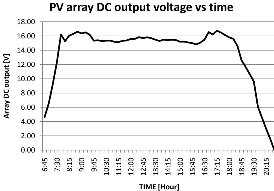
**Figure 5-7:** PV plant output voltage vs. time.
