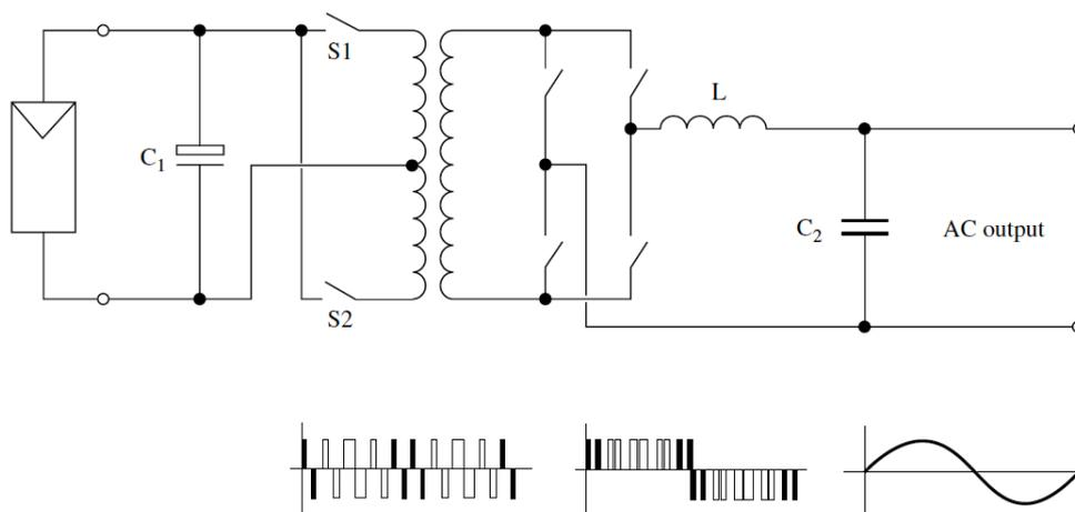
**Figure 3-17:** A sine wave inverter using a high frequency PWM signal [15]
