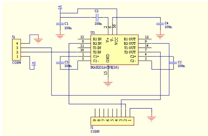
**Figure 4-71:** Schematic diagram of the RS-232 interface circuit.
