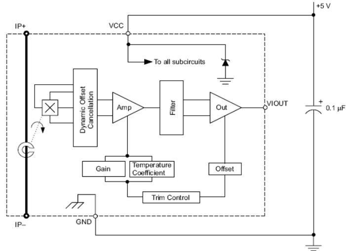
**Figure 4-26:** ACS756 block diagram [42].
