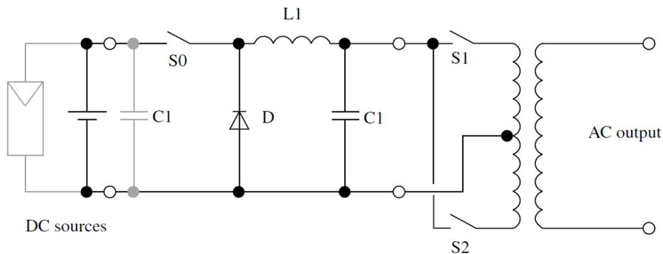
**Figure 3-16:** Simplified schematic circuit of a modified sine wave inverter [15].
