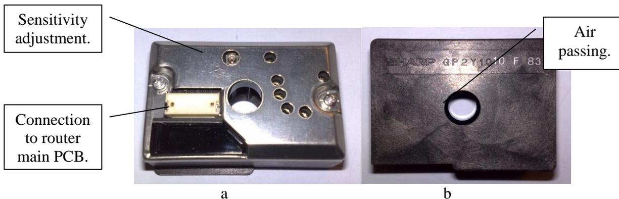
**Figure 4-56:** Back side of dust sensor (a), front side of dust sensor (b).
