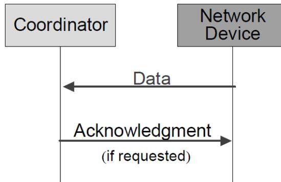
**Figure 2-22:** Communication in a nonbeacon-enabled PAN [3].
