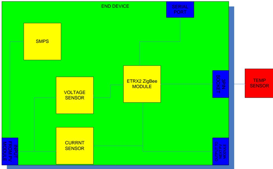
**Figure 4-68:** End device block diagram.
