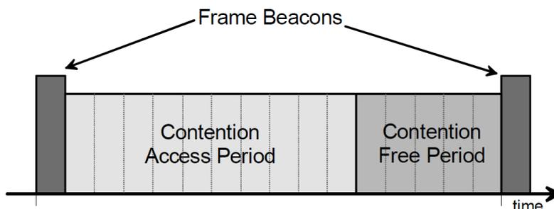
**Figure 2-20:** Superframe structure with GTSs [3].
