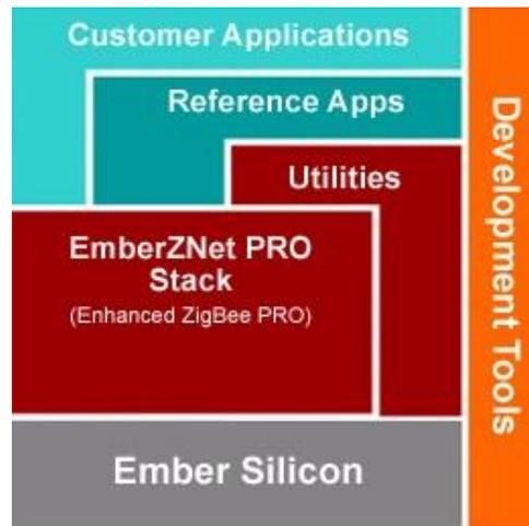
**Figure A-1:** The EmberZNet protocol stack [58].
