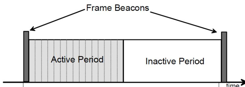
**Figure 2-19:** Superframe structure with active and inactive periods (portions) [3].
