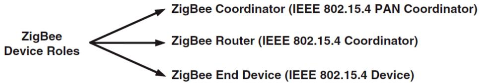
**Figure 2-28:** Correspondence of ZigBee to the IEEE802.15.4 LR-WPAN network devices [6].
