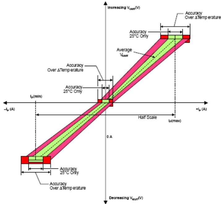
**Figure 4-27:** Output voltage versus sensed current [42].
