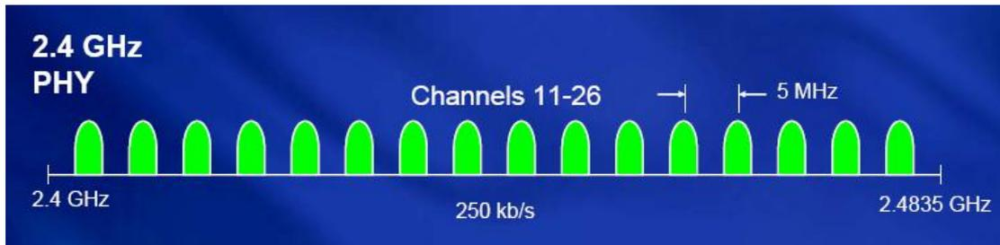
**Figure 2-12:** Available channels and data rate in the 2.4GHz ISM band [11].
