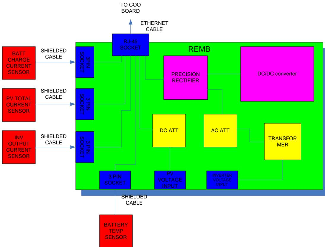
**Figure 4-19:** Block diagram of REMB.
