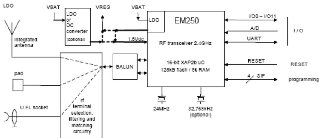
**Figure 4-6:** Block diagram of the ETRX2 ZigBee module [17].
