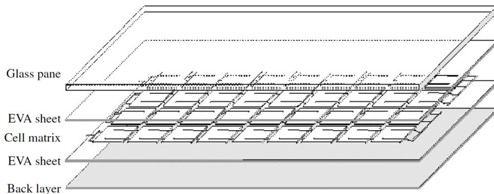
**Figure 3-5:** Structure of a PV module [15].
