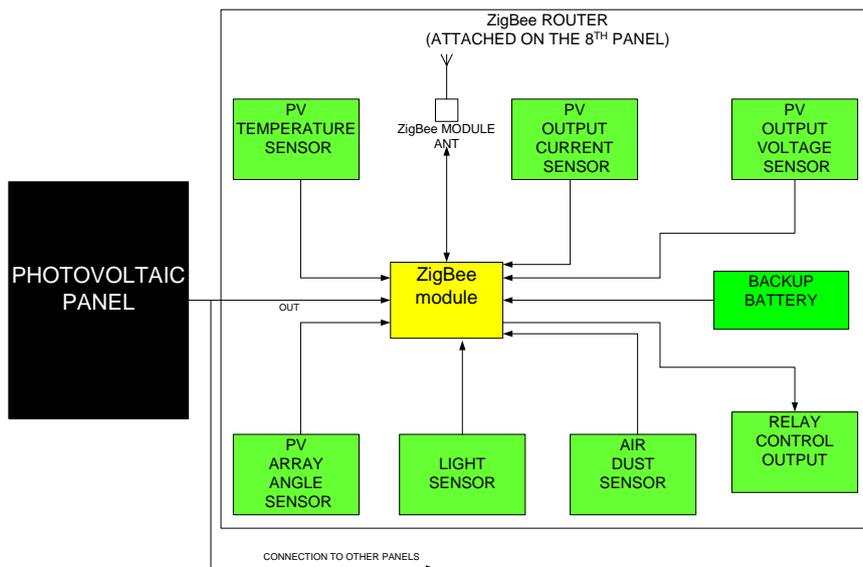
**Figure 4-3:** Simplified diagram of the router.
