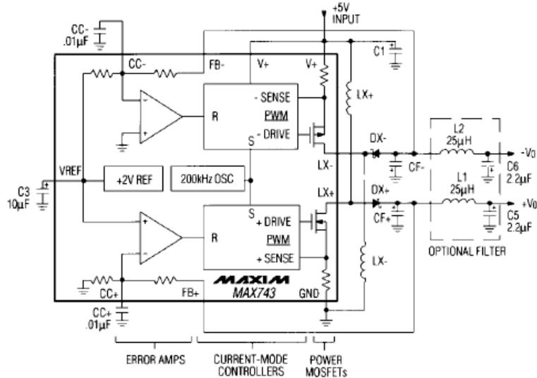
Figure 4-24: MAX743 block diagram [39].
