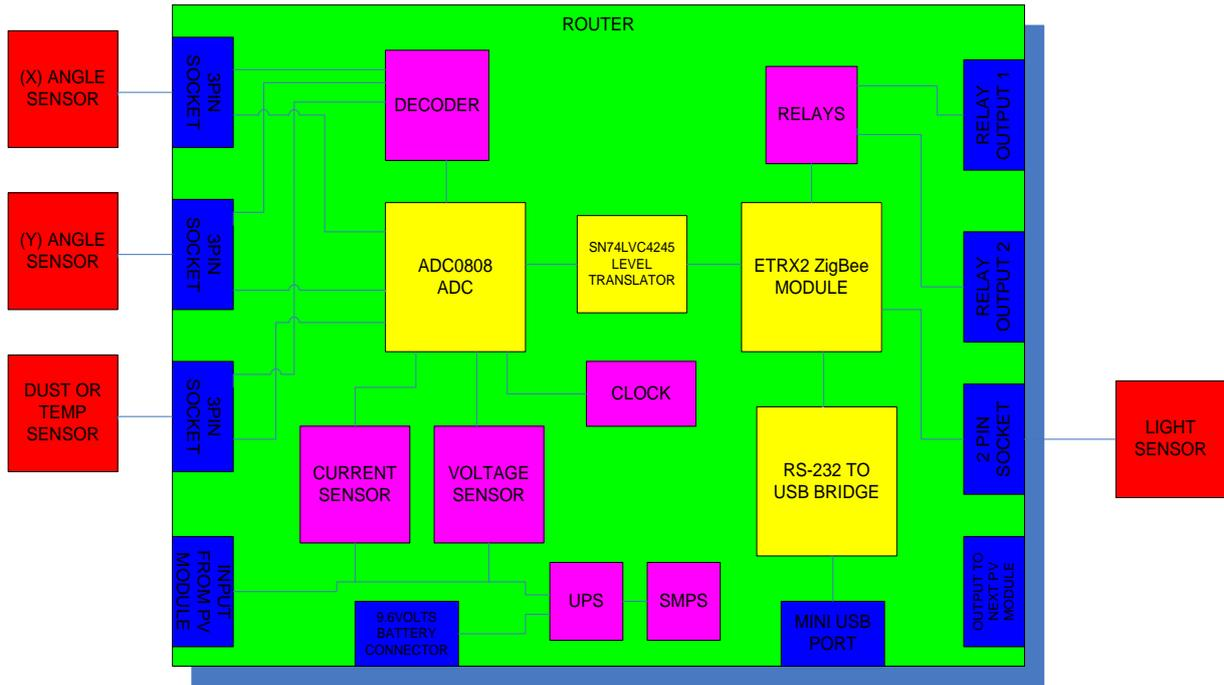
**Figure 4-48:** Block diagram of router.
