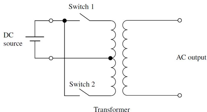
**Figure 3-14:** Simplified circuit schematic of a square wave inverter [15]
