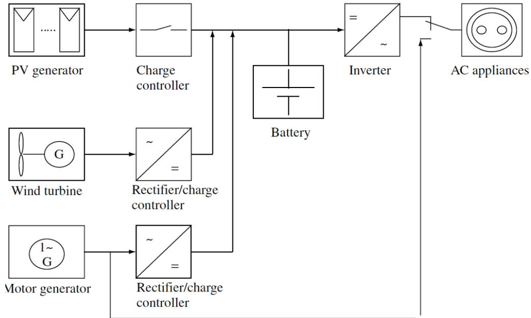
**Figure 3-7:** Block diagram of a hybrid system [15].
