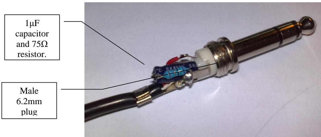
**Figure 4-46:** Components soldered into male stereo plug.
