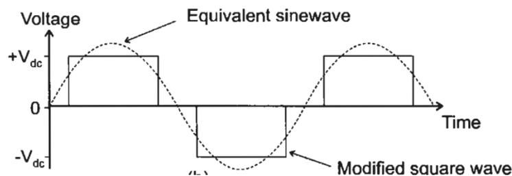
**Figure 3-15:** Output of a modified sine wave inverter [16]
