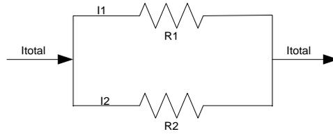
**Figure 4-28:** A simple current divider.
