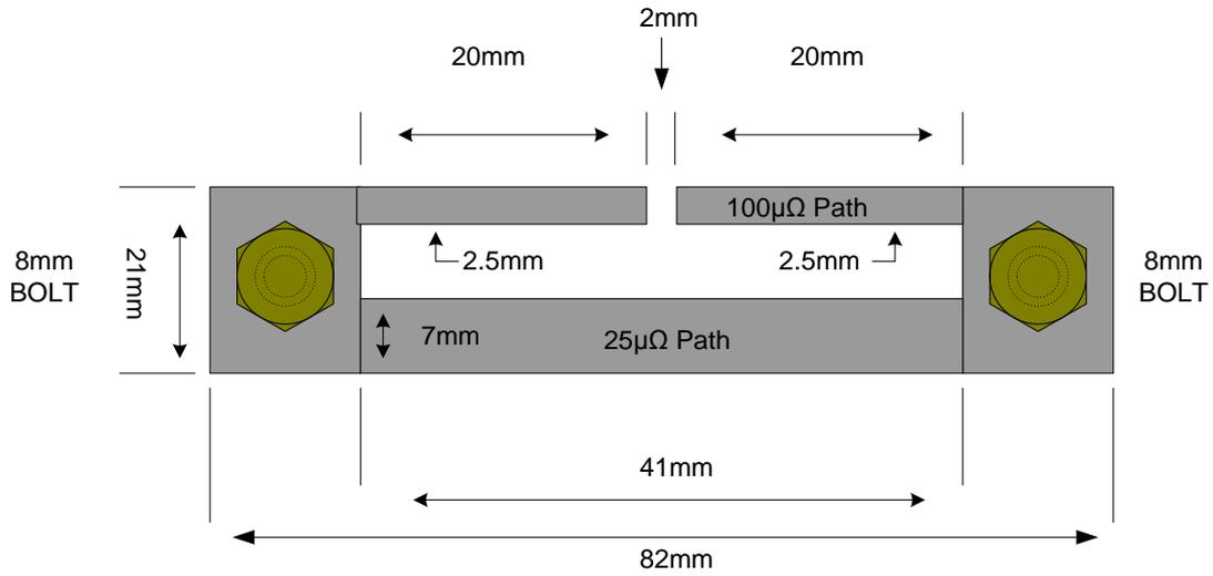
**Figure 4-32:** Mechanical drawing of the bus bar.
