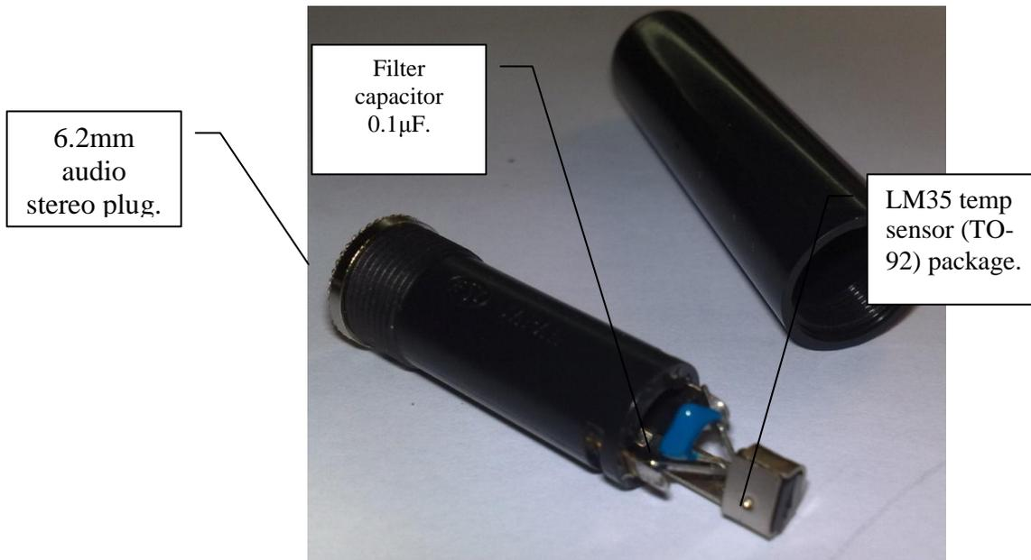
**Figure 4-45:** The LM35 in the female plug.
