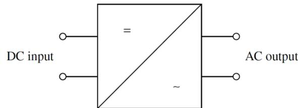
**Figure 3-11:** The schematic symbol of the inverter [15]
