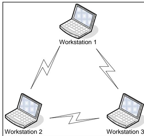
**Figure 2-6:** An independent WLAN.
