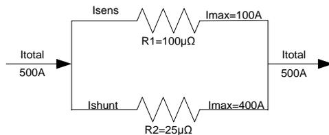
**Figure 4-31:** Final current divider equivalent circuit.
