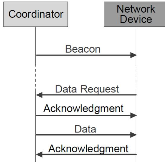
**Figure 2-23:** Communication in a beacon-enabled PAN [3].
