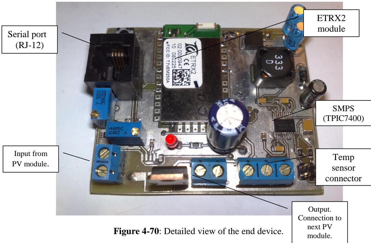
Figure 4-70: Detailed view of the end device.
