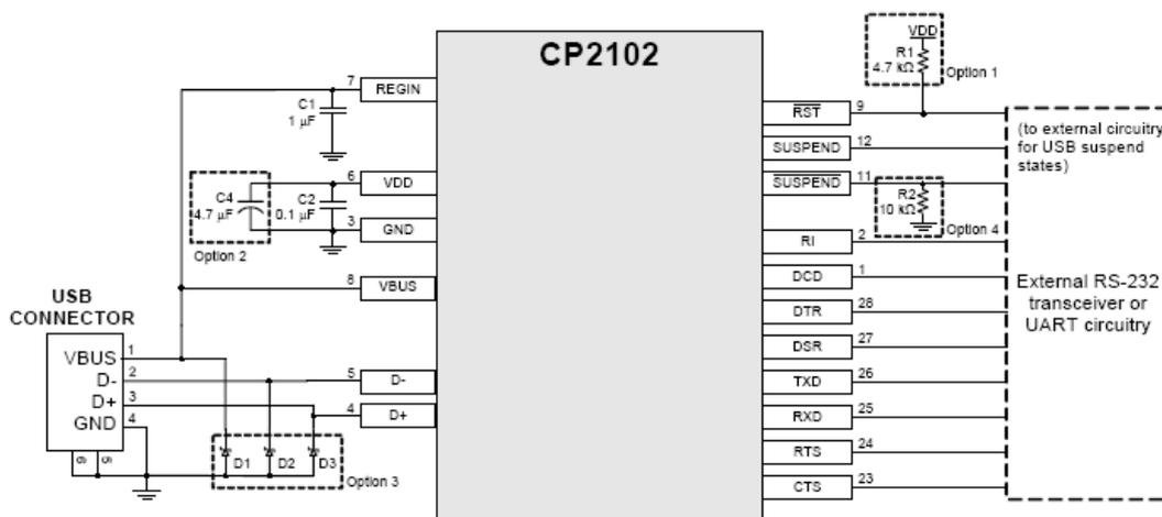
Figure 4-17: Typical connection diagram [29].
