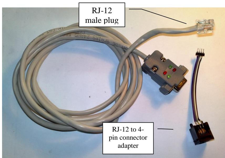
**Figure 4-74:** The serial cable and the RJ-12 to 4-pin connector adapter.
