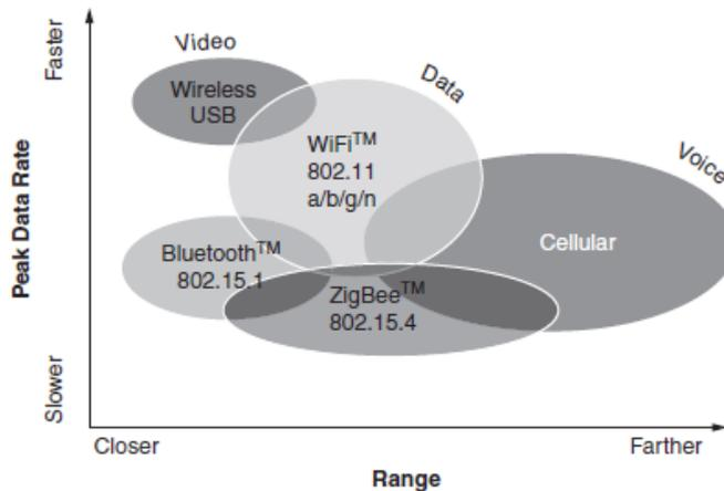
**Figure 2-37:** Comparison of ZigBee with other wireless technologies [7].
