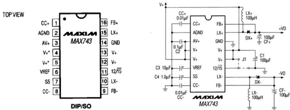
Figure 4-22: MAX743 pinout [39]. Figure 4-23: Typical connection [39].
