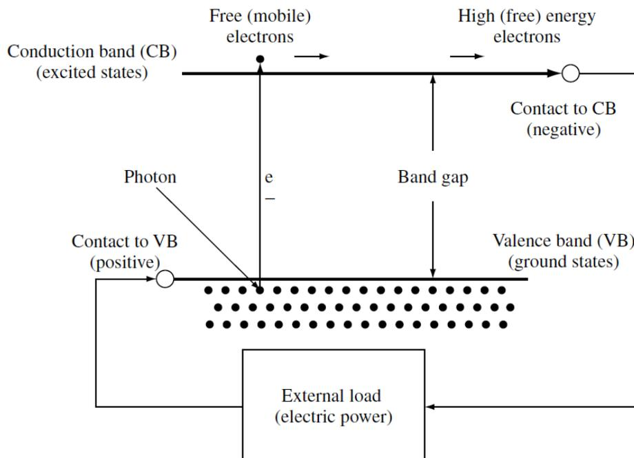
**Figure 3-1:** Basic operation of a solar cell [15].
