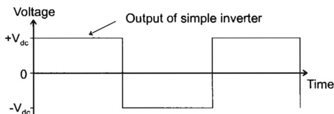
**Figure 3-13:** Output of a square wave inverter [16]
