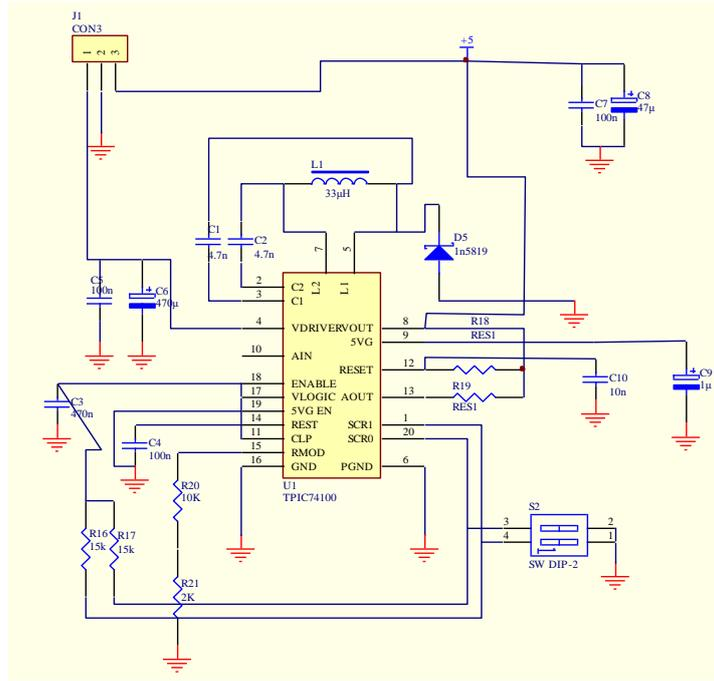
**Figure 4-64:** Schematic diagram of the 5Volts regulator.
