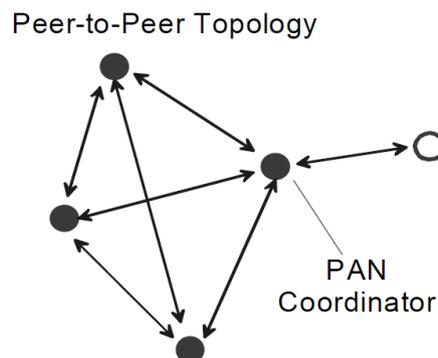
**Figure 2-16:** The Peer-to-Peer topology for the IEEE802.15.4 LR-WPAN [3]. Here too as with star topology, the first device that forms for the first time a PAN becomes the PAN coordinator. The main advantage of Peer-to-Peer networking against star is its self-organizing, self-healing capability.
