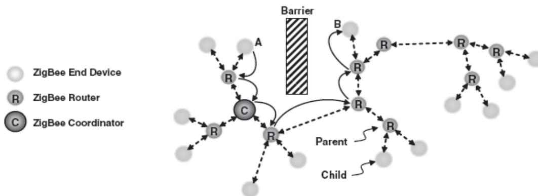
**Figure 2-32:** Example of a self-healing network [14].
