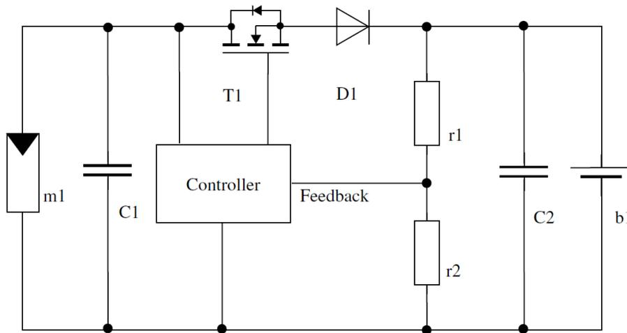
**Figure 3-9:** A series linear charge controller [15]
