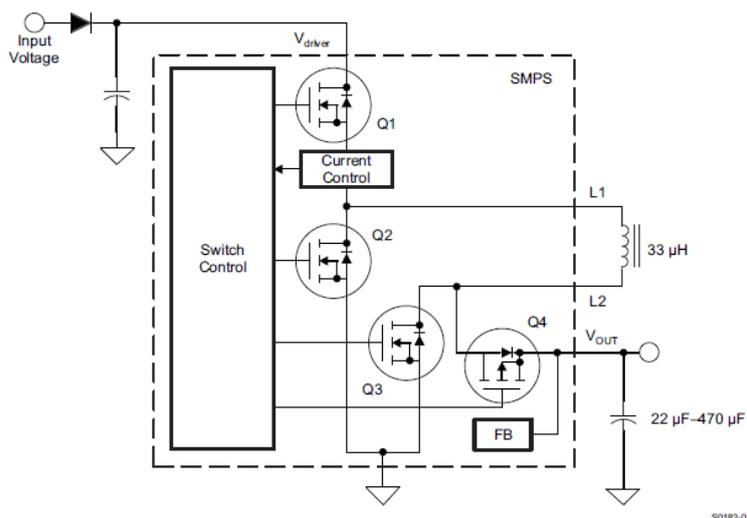
**Figure 4-63:** Buck/Boost switch mode configuration [53].
