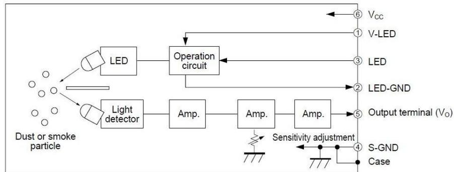
**Figure 4-54:** The GP2Y1010AU block diagram [49].
