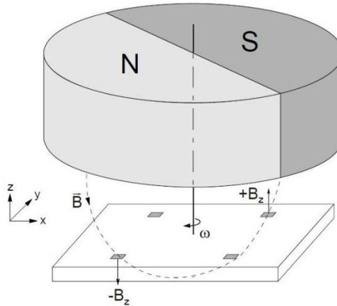
**Figure 4-58:** Principle of the magnetic field measurement using a Hall sensor [50].
