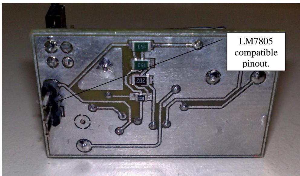
**Figure 4-67:** Back view of the voltage regulator.
