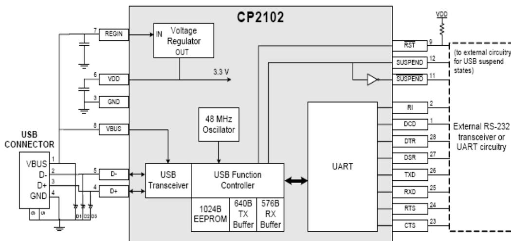
Figure 4-16: Block diagram of CP2102 [29].
