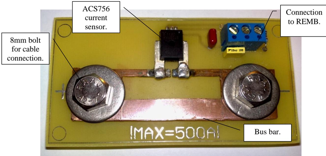
**Figure 4-34:** The finished current sensor.
