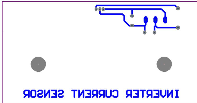
Figure 4-40: PCB layout (Bottom layer).
