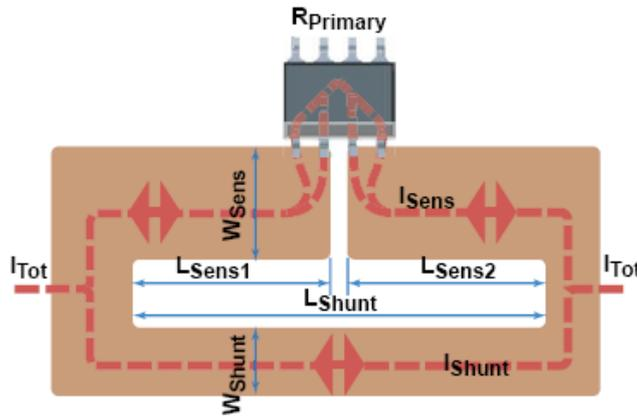
**Figure 4-30:** Reference circuit for calculation of trace layout dimensions [44].
