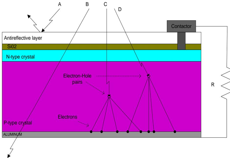
**Figure 3-2:** Infrastructure of a solar cell.
