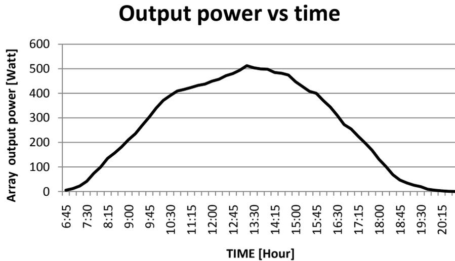
**Figure 5-8:** PV plant output power vs. time.
