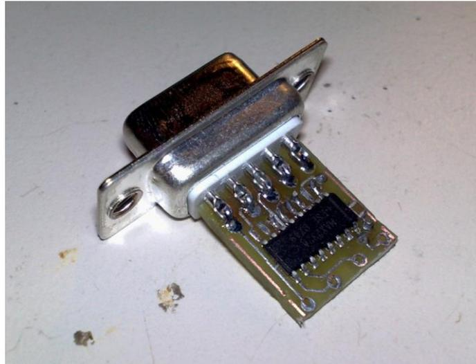
**Figure 4-73:** The PCB of the interface circuit
