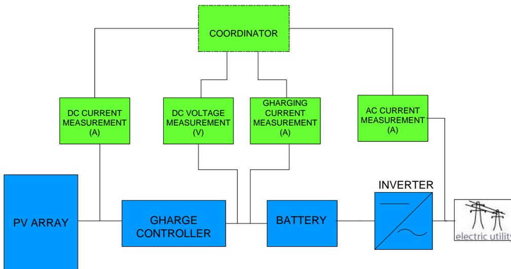
**Figure 4-5:** Measurement points at the CSS.
