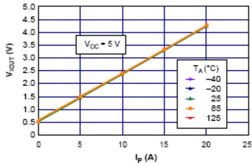
**Figure 4-36:** Output voltage versus sensed current [45].
