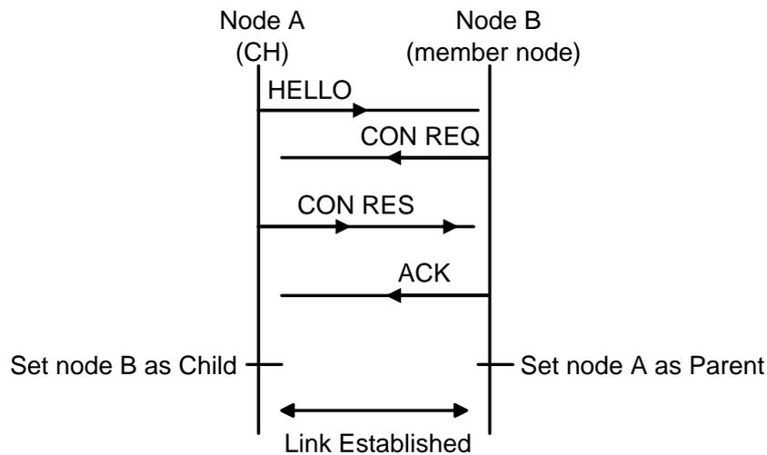
**Figure 2-36:** Link setup between CH and member node [8].
