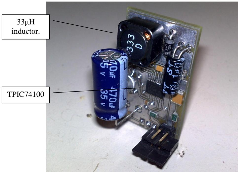
**Figure 4-66:** Photo of the 5Volts regulator.
