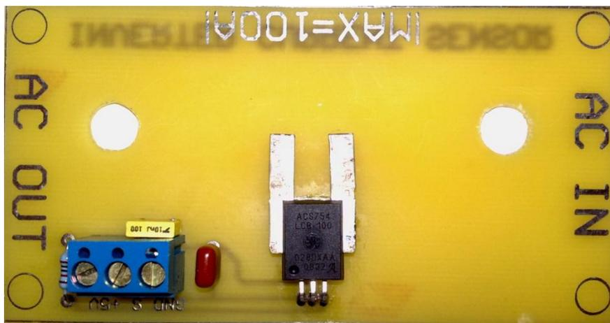
**Figure 4-42:** The inverter current sensor.
