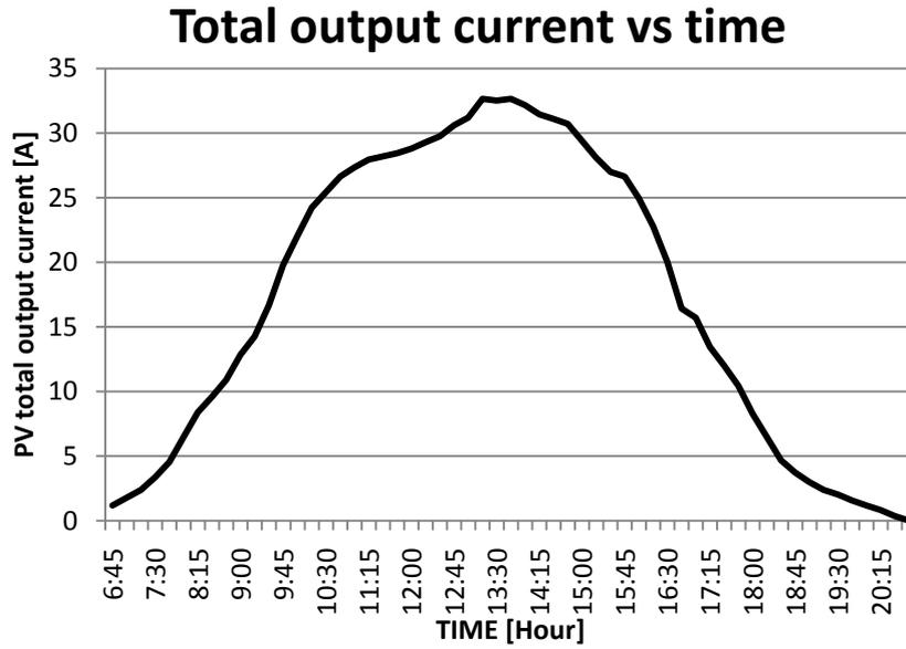
**Figure 5-6:** PV total output current vs. time.
