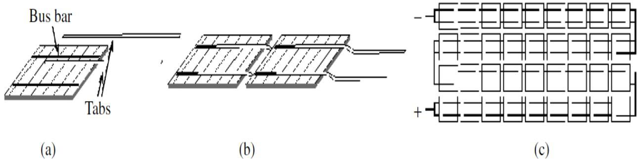
**Figure 3-4:** (a) Cell interconnection with tabs; (b) two cells in series; and (c) layout of 36 series-connected cells [15].
