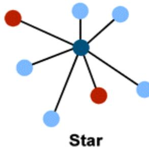
**Figure 2-29:** ZigBee star network topology [14].
