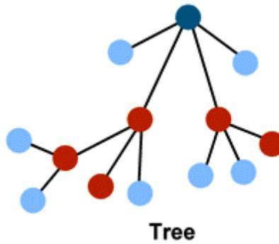
**Figure 2-30:** ZigBee cluster-tree network topology [14].
