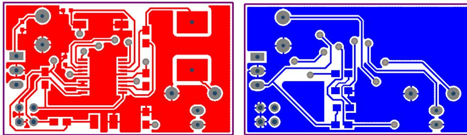
**Figure 4-65:** Top (red) and bottom (blue) layers of the 5Volts regulator.
