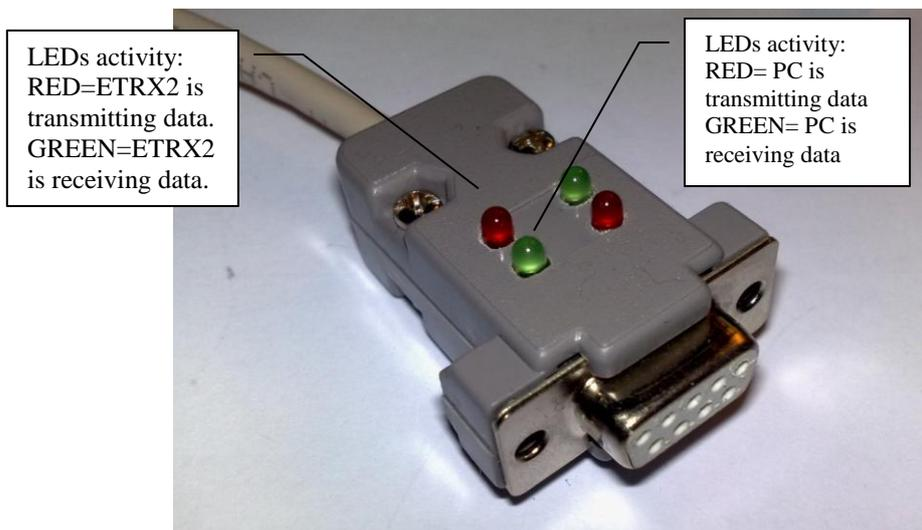
**Figure 4-72:** The RS-232 male plug with the integrated RS-232 driver/receiver.
