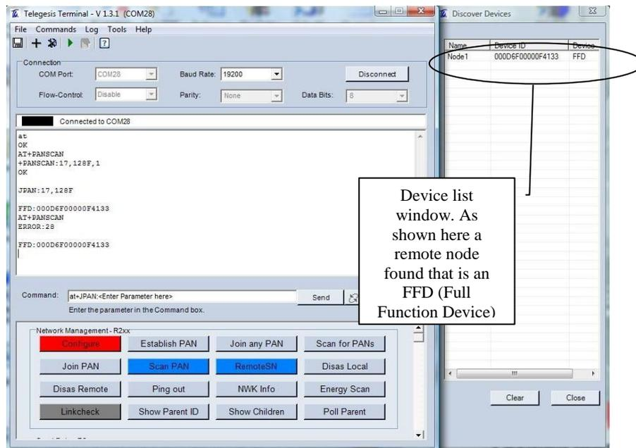
**Figure A-3:** An FFD as it is displayed in the device list window.
