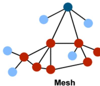
**Figure 2-31:** ZigBee mesh network topology [14].
