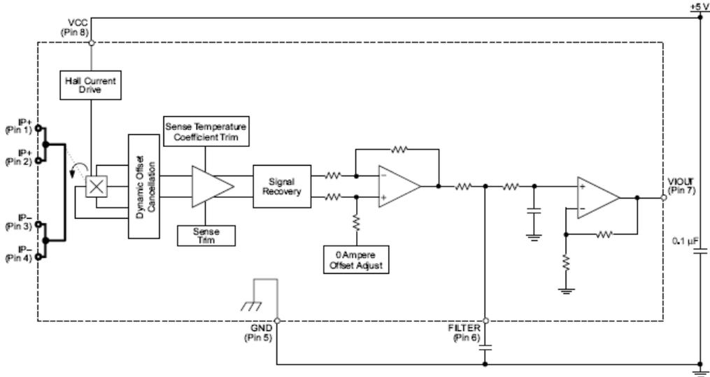
**Figure 4-35:** Block diagram of ACS713 [45].
