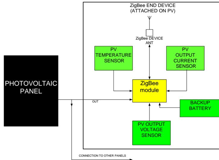
**Figure 4-2:** Simplified diagram of a ZED.
