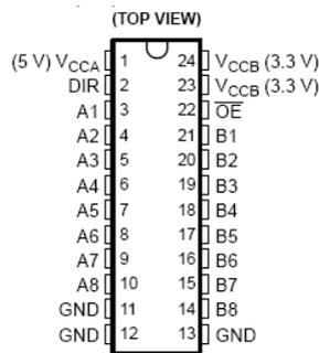
Figure 4-14: SN74LVC4245A pinout
