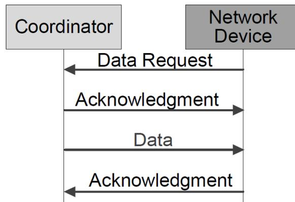
**Figure 2-24:** Communication in a nonbeacon-enabled PAN [3].
