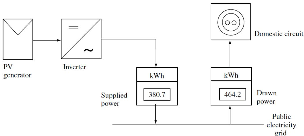
**Figure 3-8:** A grid connected PV system [15]
