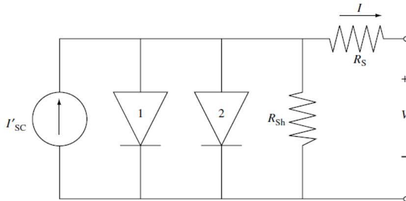
**Figure 3-3:** Equivalent circuit of a solar cell [16].
