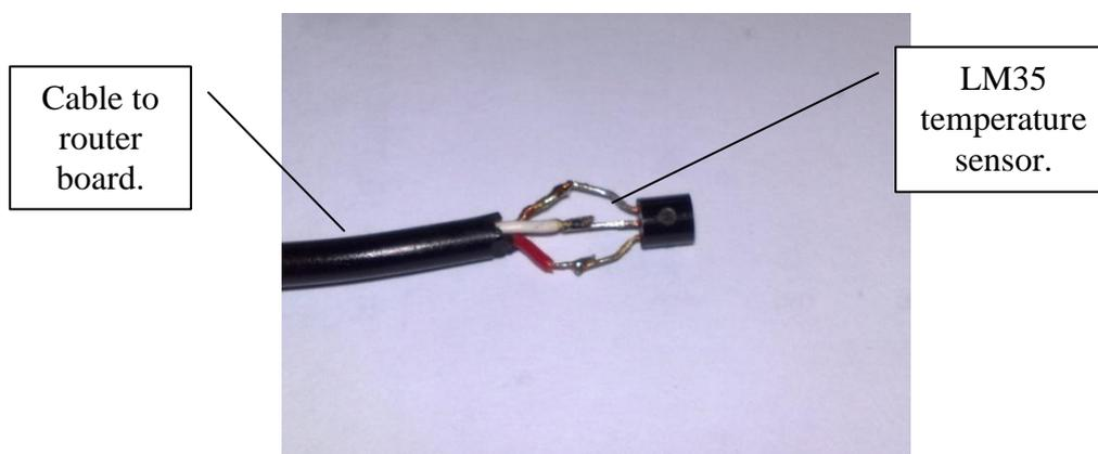
**Figure 4-53:** The PV temperature sensor.
