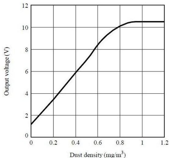
**Figure 4-55:** Output voltage versus dust density [49].
