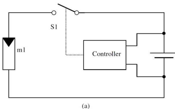
**Figure 3-10:** A series switch mode charge controller [16]
