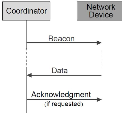
**Figure 2-21:** Communication in a beacon-enabled PAN [3].
