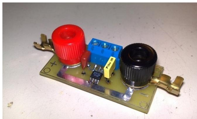
**Figure 4-39:** The battery charging current sensor
