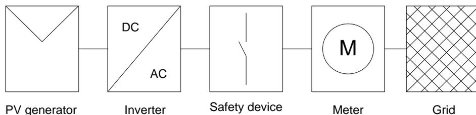
**Figure 3-12:** General structure of a grid connected photovoltaic system [15]
