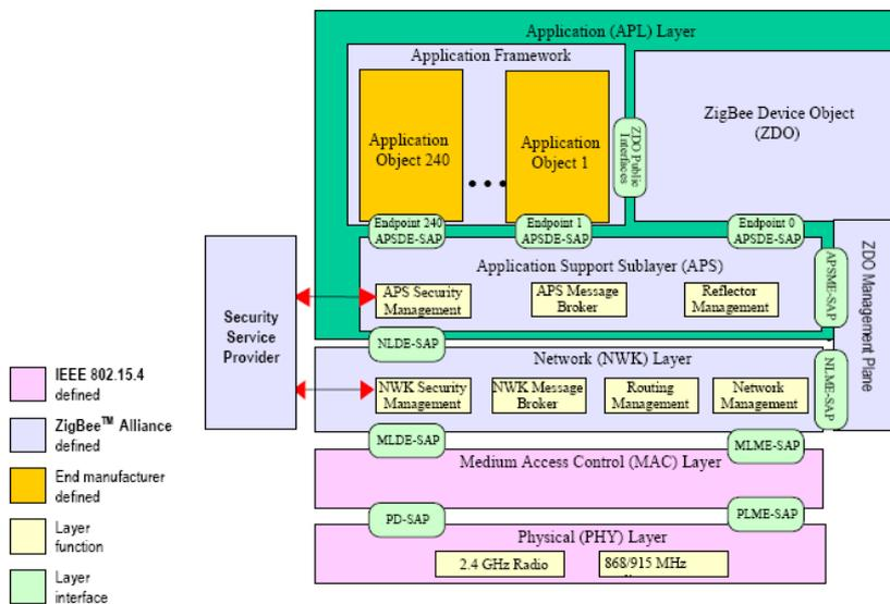
Figure 2-26: The ZigBee protocol stack architecture [10].
