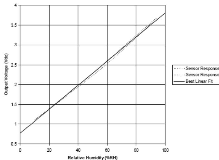
**Figure 4-18:** Typical output voltage versus relative humidity (@25C)
