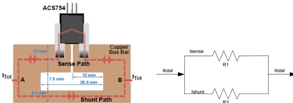
**Figure 4-29:** The copper bus bar (configuration for the ACS754 shown here) and its equivalent circuit [44].
