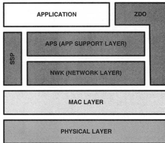
**Figure 2-27:** Simplified illustration of the ZigBee protocol stack [9].
