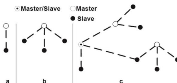
**Figure 2-10:** The piconet network topologies. a) Point-to-point connection (single slave operation), b) point-to-multipoint connection (multislave operation), c) scatter net operation [1].
