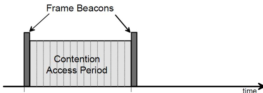
**Figure 2-18:** Superframe structure without GTSs [3].
