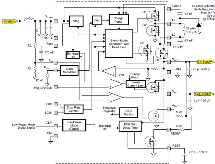
Figure 4-62: TPIC74000 block diagram [53].
