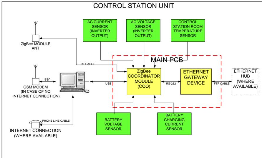
**Figure 4-4:** Block diagram of the CSS.
