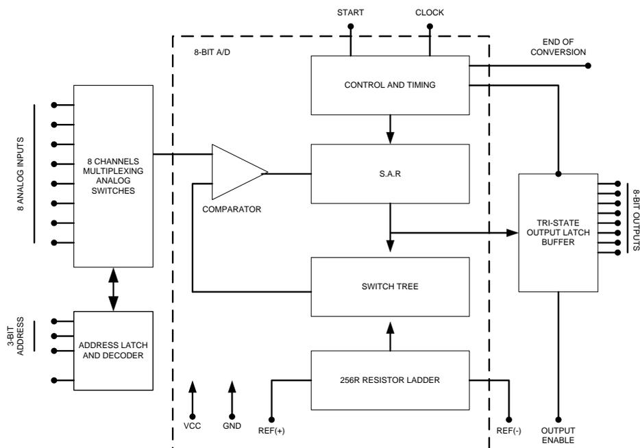
**Figure 4-12:** Block diagram of the ADC0808 [23].
