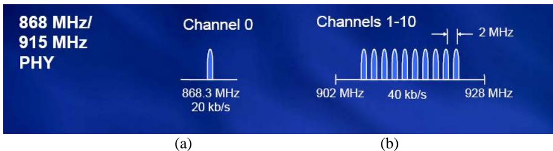
**Figure 2-13:** Available channels and data rates for the 868MHz (a) and 915MHz (b) bands [11]
