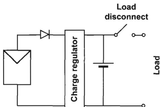
**Figure 3-6:** Typical configuration of a standalone photovoltaic system [16].
