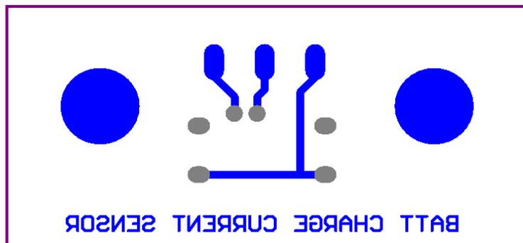
**Figure 4-38:** PCB layout (Bottom layer).
