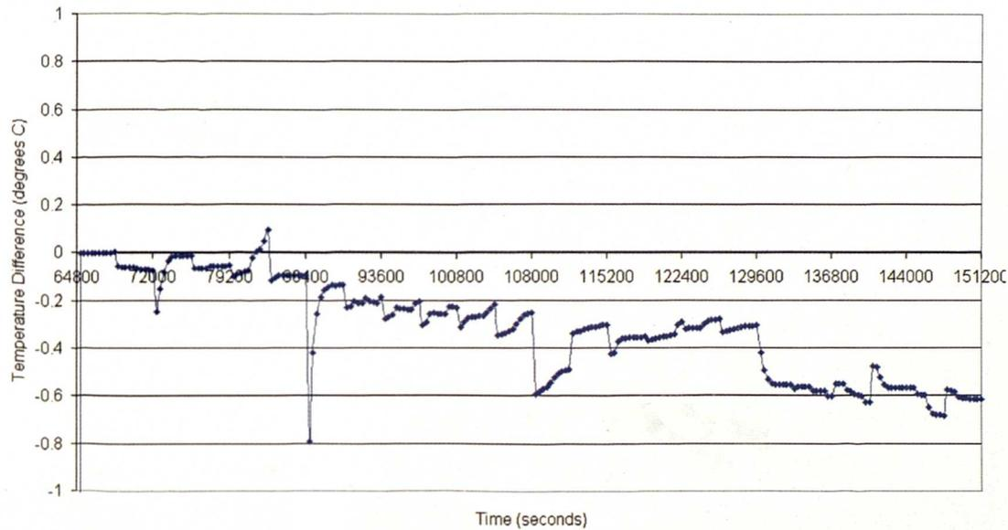
Figure 6.13: Differences between the fully transient and DTM-CFD Procedure temperature solutions generated within the centre of the enclosure
