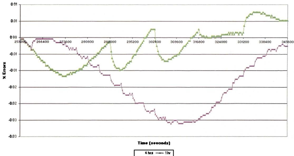
Figure 6.10: Stage 2 – Temperature Difference between Fully Transient Simulation and the DTM-CFD procedure for data collected adjacent to the wall.
