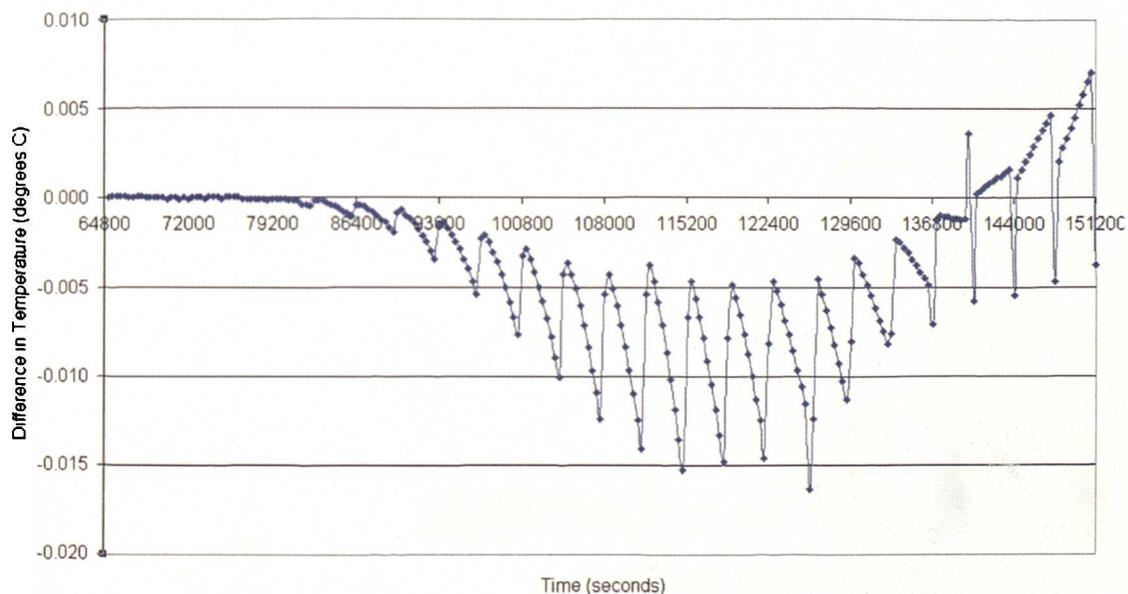
Figure 6.11: Stage 3 – Temperatures Differences between the Fully Transient and the DTM-CFD Procedure for data collected for the first air cell adjacent to the wall
