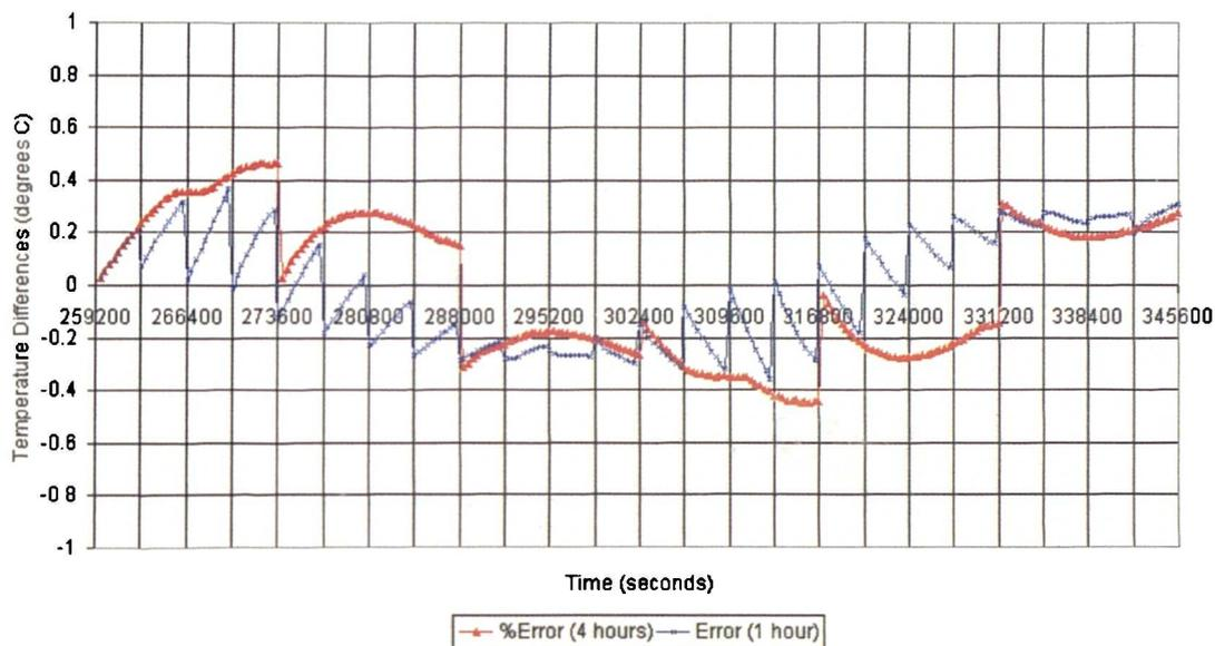
Figure 6.9: Stage 1 – Difference between Errors of Fully Transient and DTM-CFD Procedure Temperature Solutions generated at the midpoint of the enclosure
