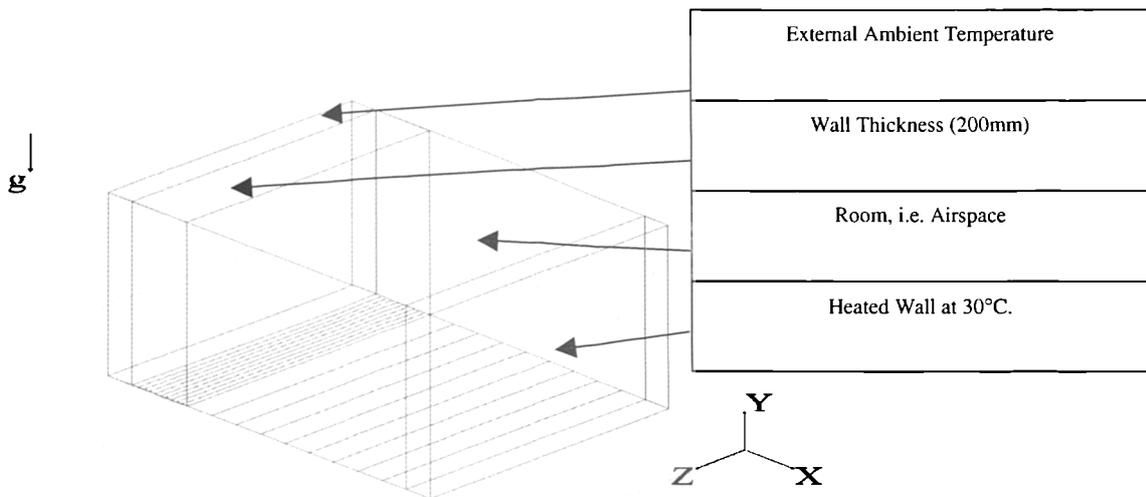
Figure 4.1: Illustration of the geometry of the enclosure (including grid construction)
