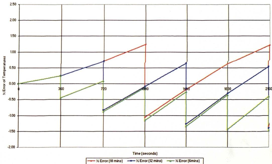
Figure 5.13: Error profiles generated by a linearly increasing ambient of  $0.06^{\circ}\text{C}/\text{min}$ .
