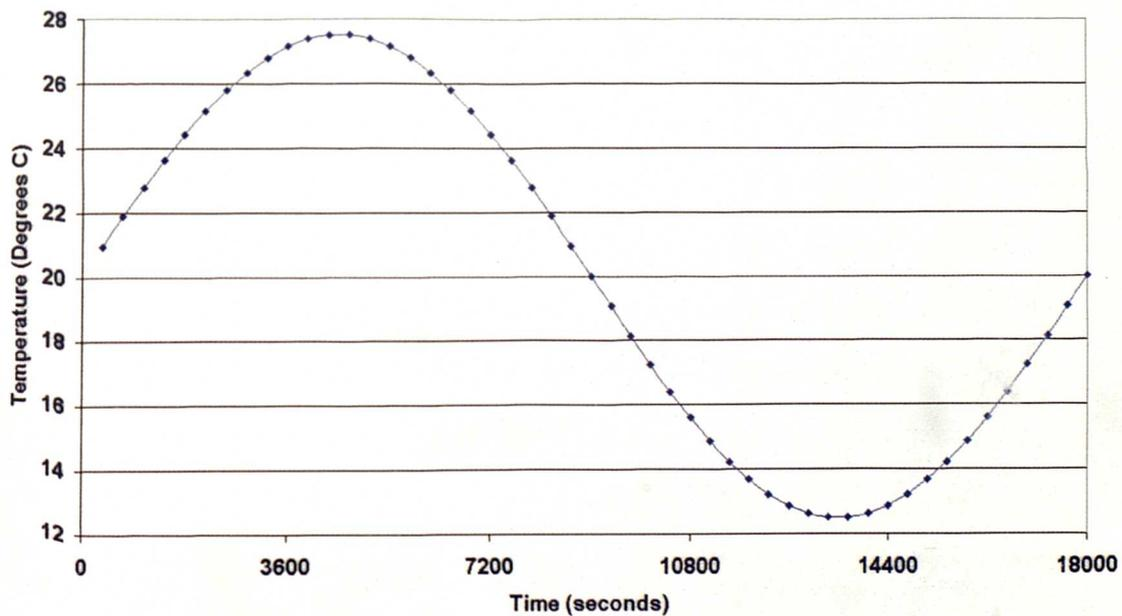
Figure 5.5: Sinusoidal Ambient Profile (15°C Amplitude and 5 hour Period)
