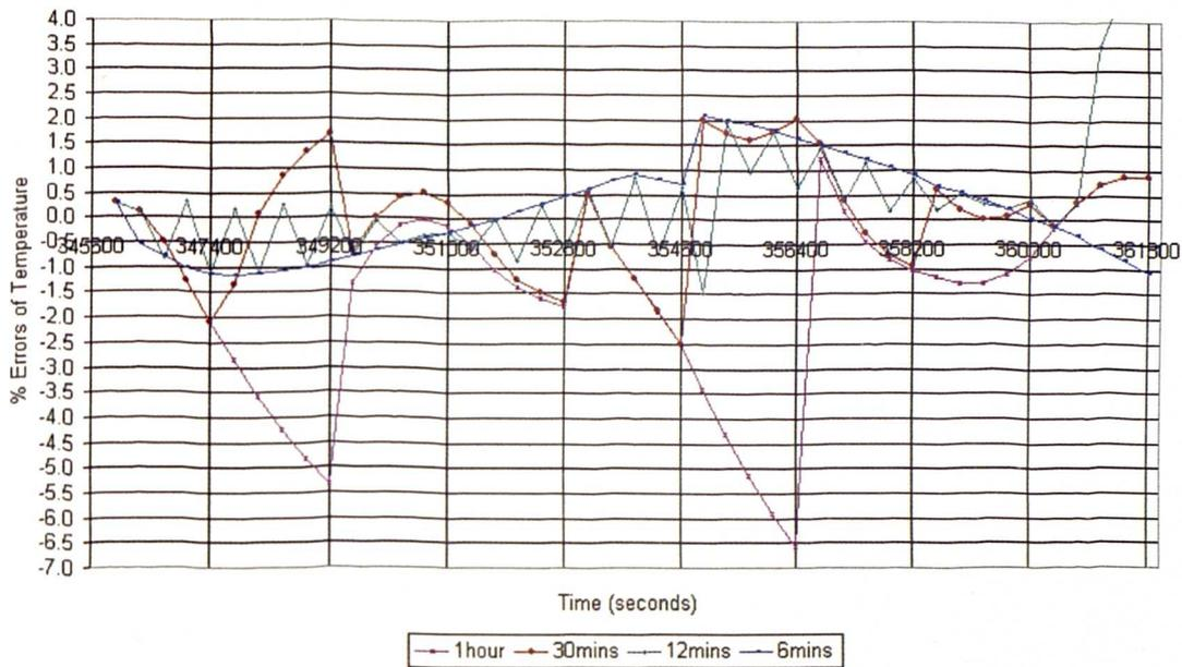
Figure 5.7: % Error of Transient Frozen Flow for a High Frequency External Ambient Sinusoid tested on Material C3W1 (TRANSIENT VALUES)
