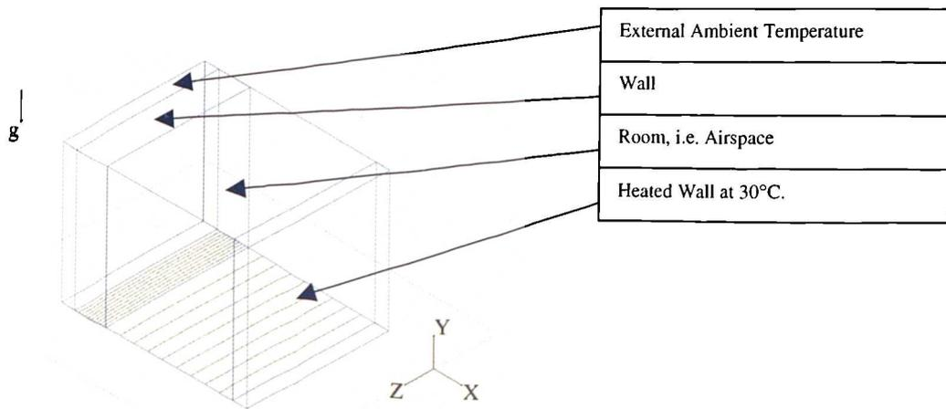
Fig B7: Geometry of Test B4
