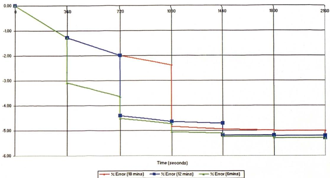
Figure 5.12: Error profiles generated by a linearly increasing ambient of  $0.125^{\circ}\text{C}/\text{min}$ .
