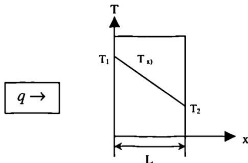
Fig.A1: One-dimensional Heat Transfer by Conduction
