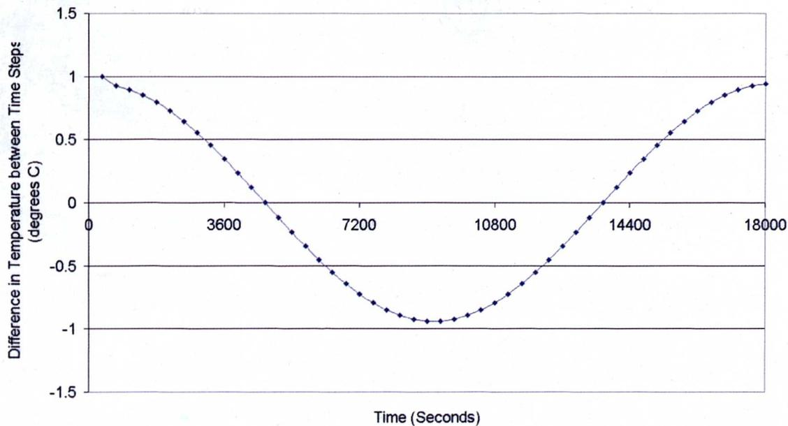
Figure 5.8: Rate of Change of Sinusoidal Ambient Profile (15°C Amplitude and 5 hour Period)
