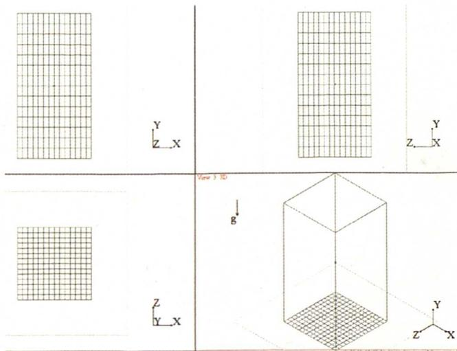
Fig A5: Cuboid including the configuration of the 3-Dimensional Grid
