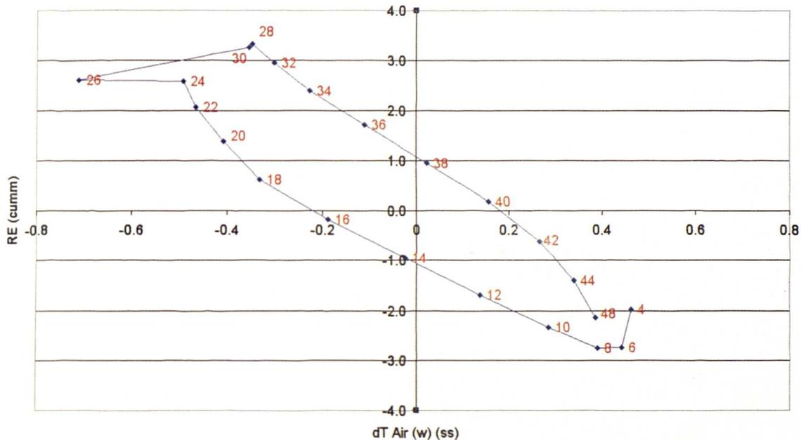
Fig. 5.10: 12-minute transient period showing the Relationship between dT Air (w) (ss) and RE (cumulative). [Note: the number labels represent the time step numbers].
