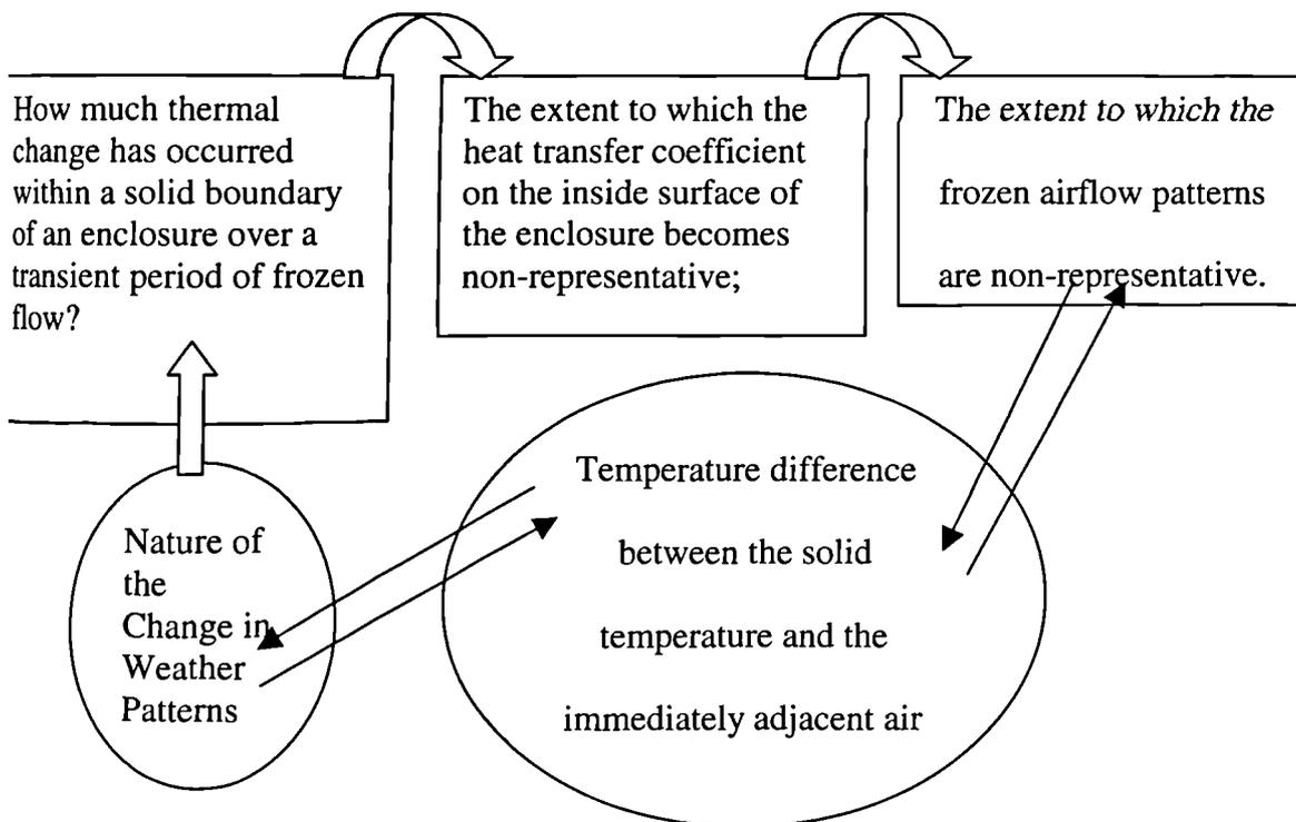
Fig C12: Flow Chart indicating the influences upon error incurred by using the DTM-CFD tool
