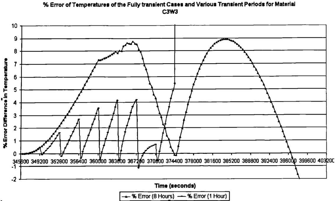
Figure C11: % Error of Temperatures of the Fully Transient Cases and Various Transient Periods for Material C3W3
