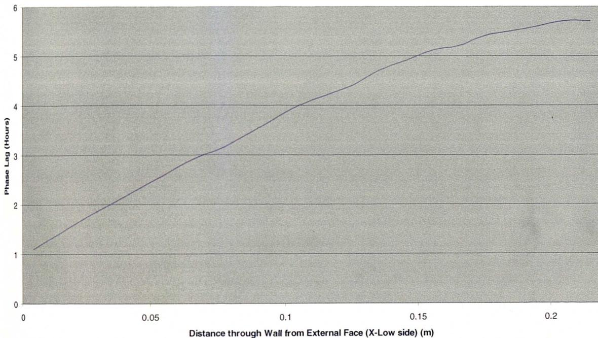
Fig B3: Phase Lag through the wall as recorded at each monitoring point within the wall, recorded at time 367200s
