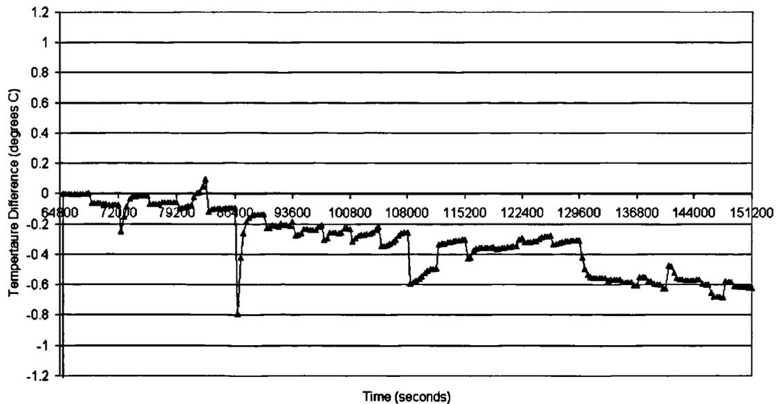
Figure 6.12: Stage 4: Temperature Difference between the Fully Transient and DTM-CFD Procedure Solution for Temperature generated within the air adjacent to the wall
