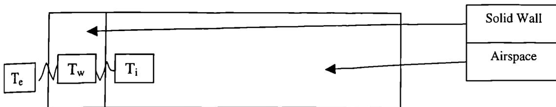
Fig C13: Cross-section of an Enclosure
