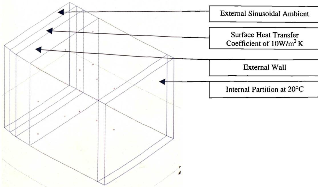
Fig B1: Geometry of Test B1
