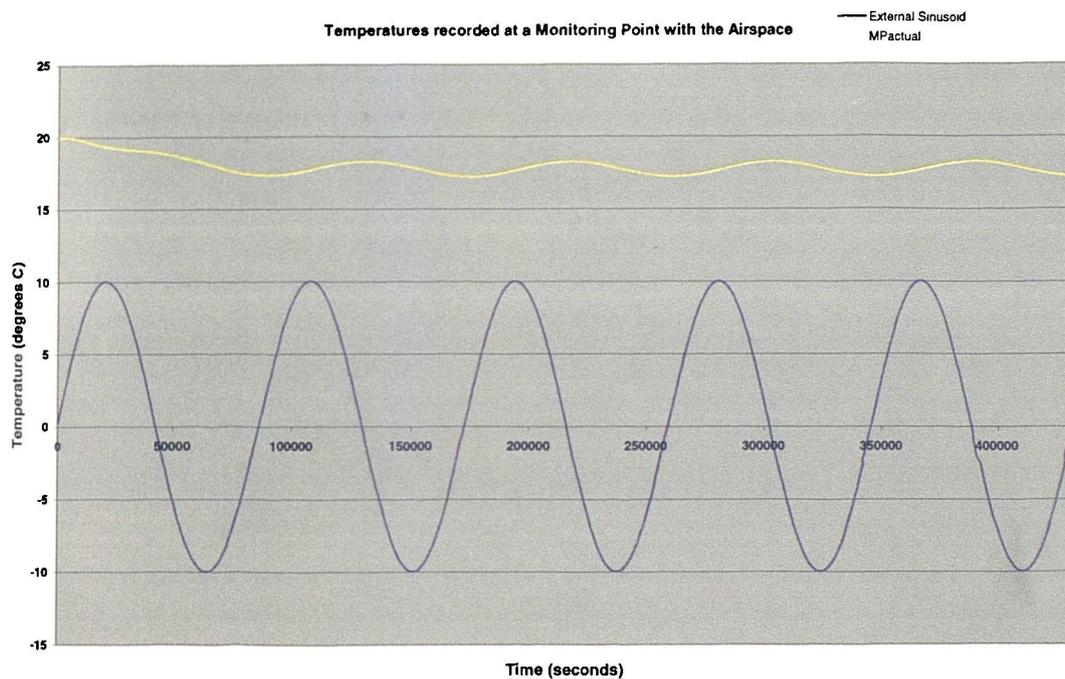
Figure B5: Graph of Temperatures recorded at a Monitoring Point located within the airspace
