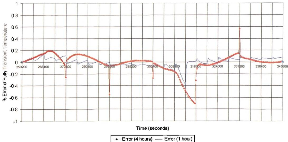
Figure 6.8: Stage 1 – Differences between Fully Transient and DTM-CFD Procedure Temperature Solutions generated at the first cell of air adjacent to the wall
