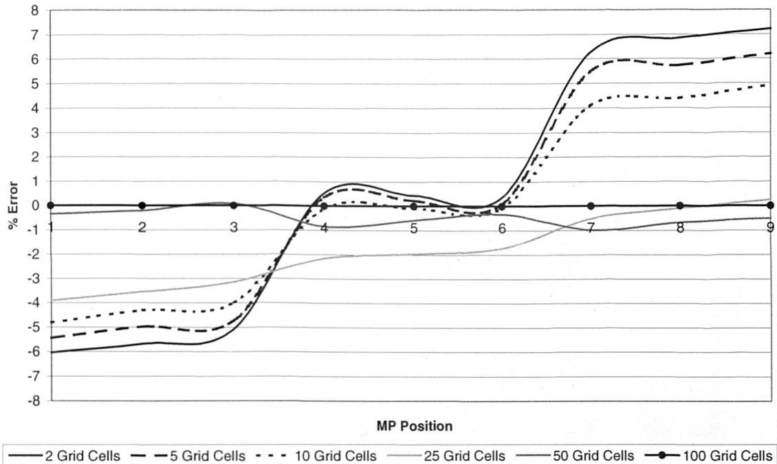
Figure 4.2: % Error of Temperature within  $1\text{m}^3$  Enclosure using various Grid Cell Numbers (in the space)
