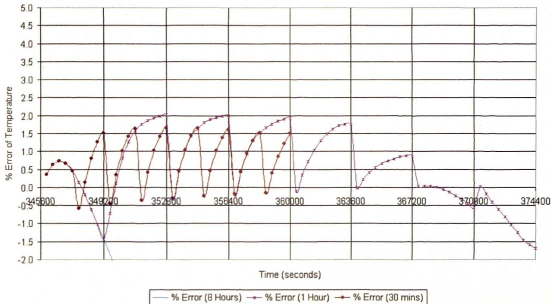
Figure 5.4: % Error of Transient 'Frozen Flow' Period for Material C3W1, using a Double Amplitude Sinusoid
