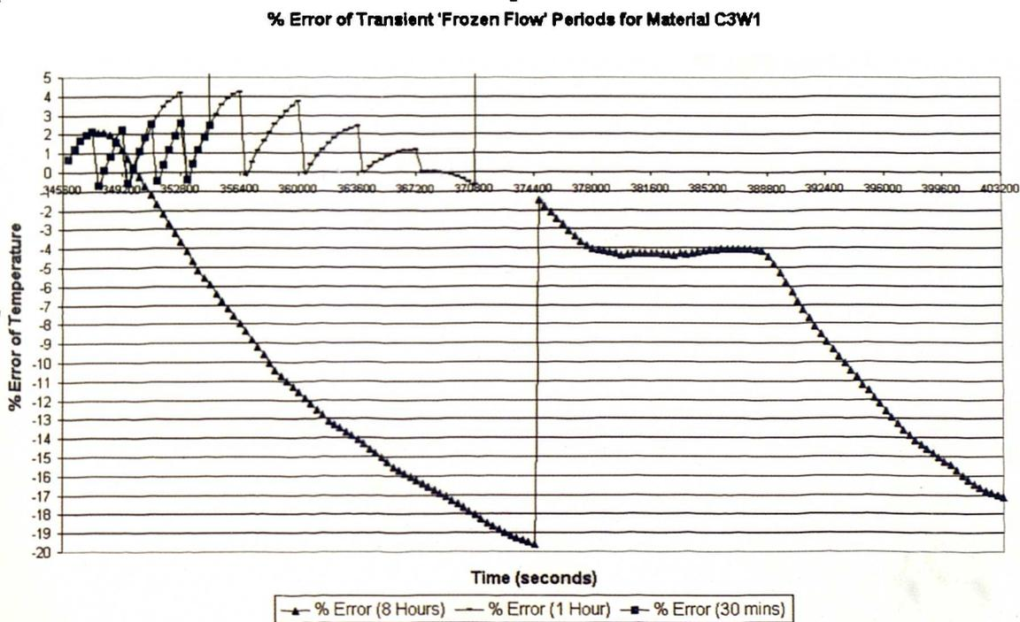
Figure C9: % Error of Transient 'Frozen Flow' Periods for Material C3W1
