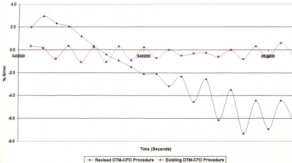
Fig C14: Comparison between Simulation Results Collected for the Existing and Revised DTM-CFD Procedure using 12 min transient periods of Frozen Flow
