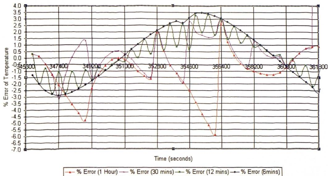
Figure 5.6: % Error of Transient Frozen Flow for a High Frequency External Ambient Sinusoid tested on Material C3W1 (STEADY STATE VALUES)
