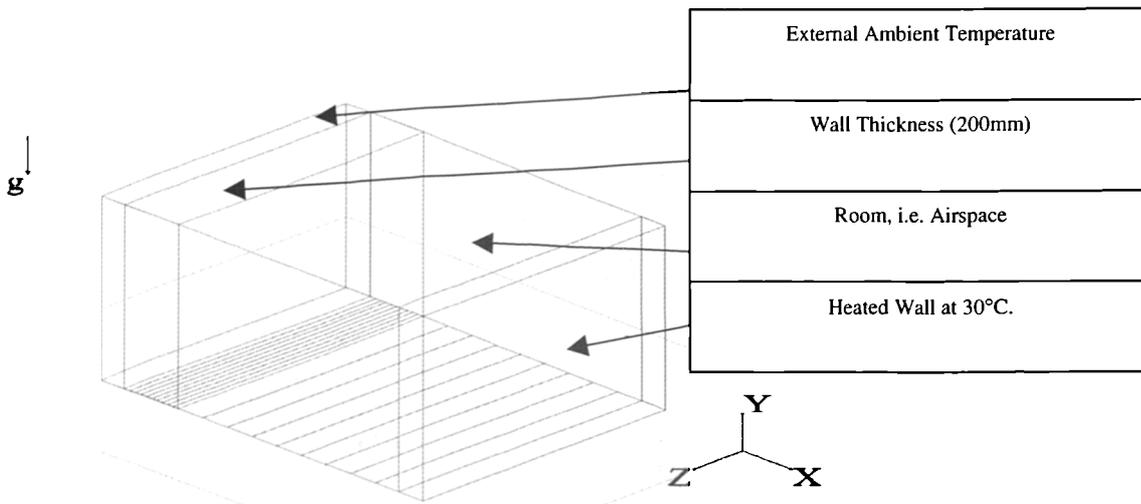
Fig C1: Test Geometry used to assess the performance of the 'Freeze Flow' Function
