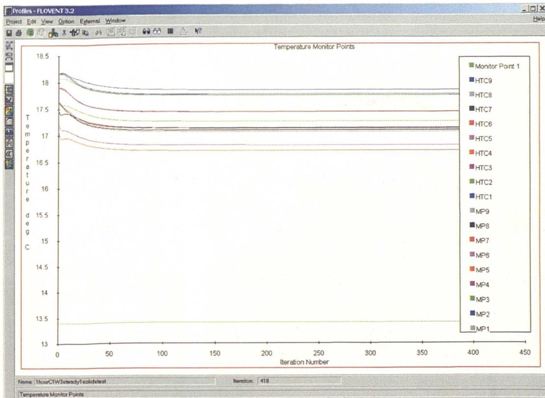
Fig C2: Temperature profiles of the Temperature data collection points within the Enclosure
