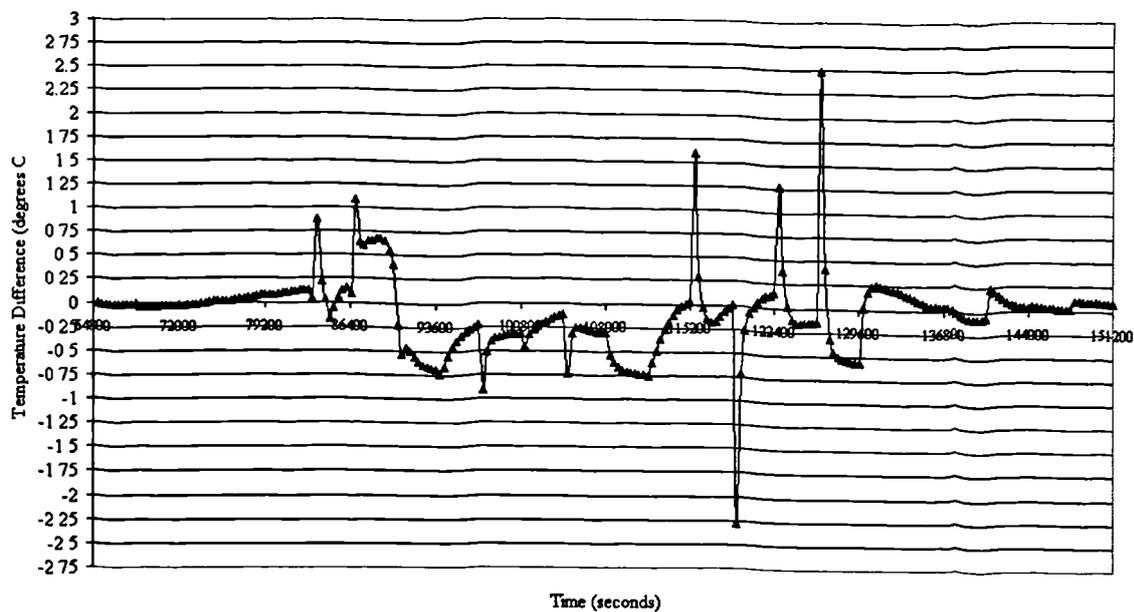
Figure 6.14: Comparison of the Fully Transient and DTM-CFD Procedure Temperature Results within the air adjacent to the wall
