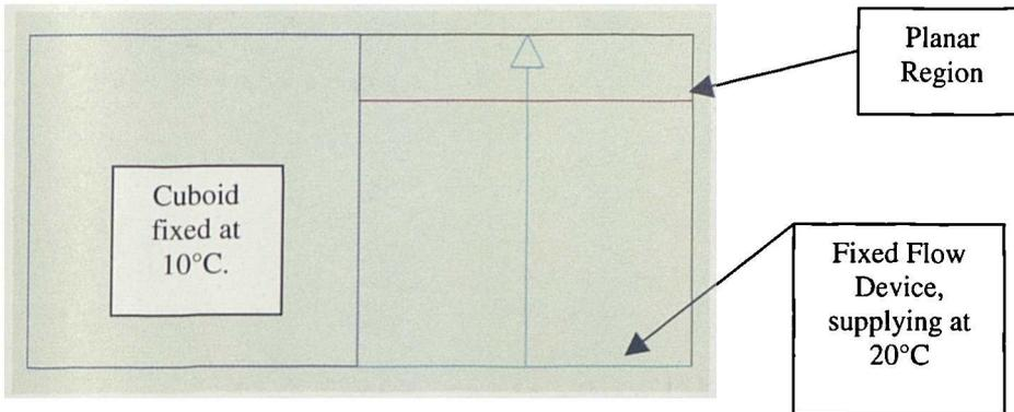
Fig. A3: Geometry of Convection Test Case, as constructed within FLOVENT
