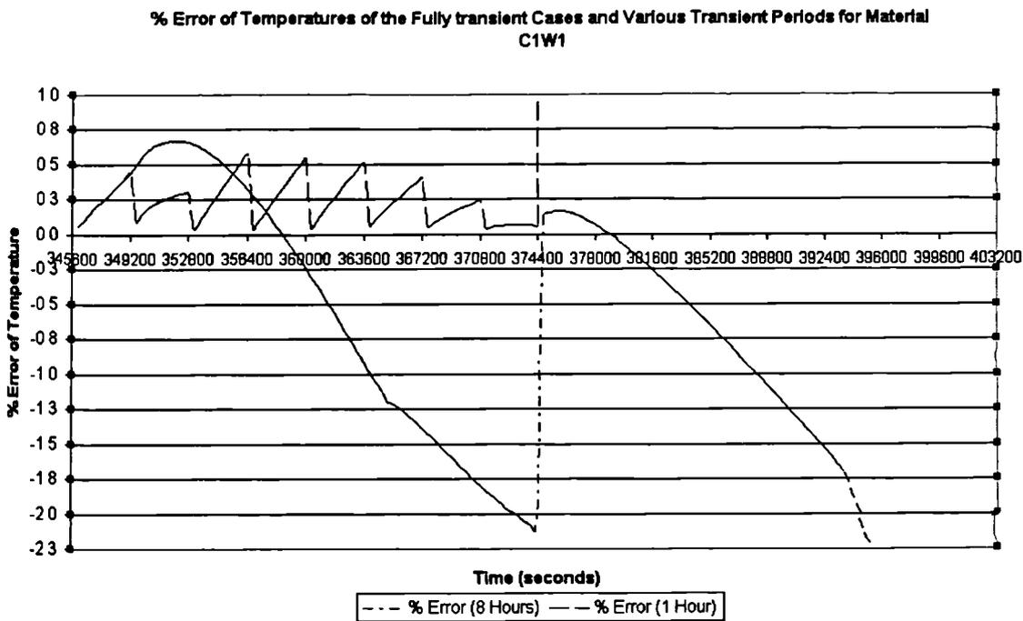
Figure C3: % Errors of Transient ‘Frozen Flow’ Periods for Material C1W1
