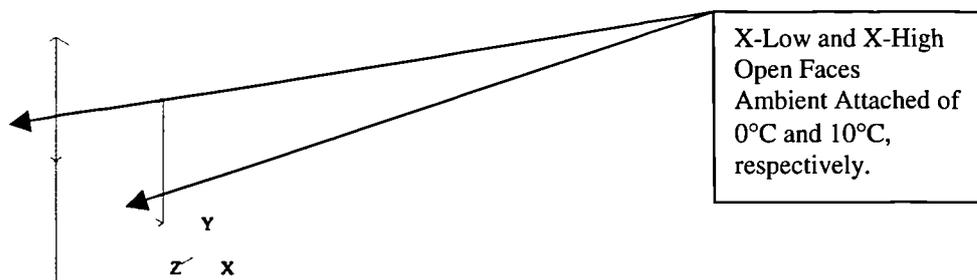
Fig. A2: Geometry of Conduction Test
