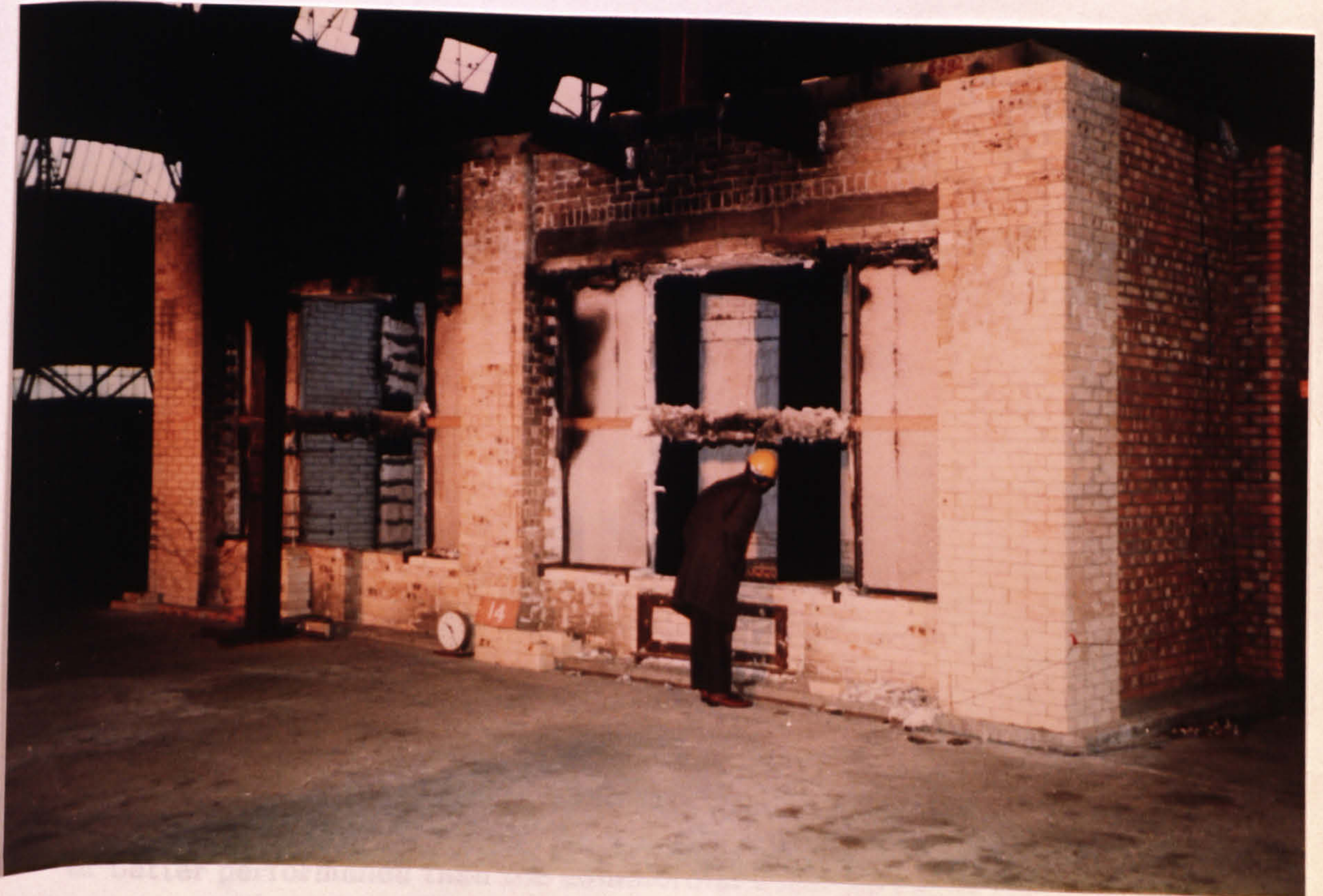
The plates were then placed in the test rig alongside 21 column sections with column sections of 203 mm x 203 mm x 30 mm
