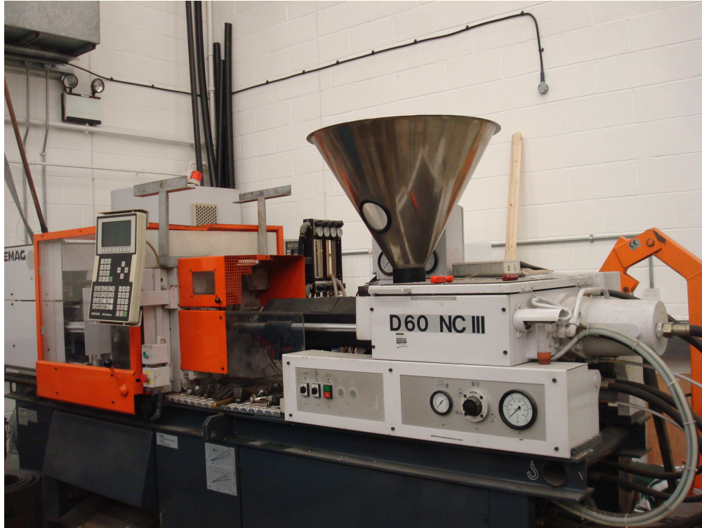
Figure 3.2 Injection moulding machine D60NCIII in operation under the given conditions to make tensile test bars
