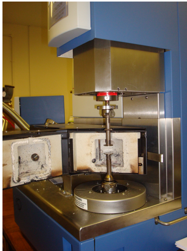
Figure 3.14 Two parallel plates of ARES inside the furnace where sample was placed to make a small disc
