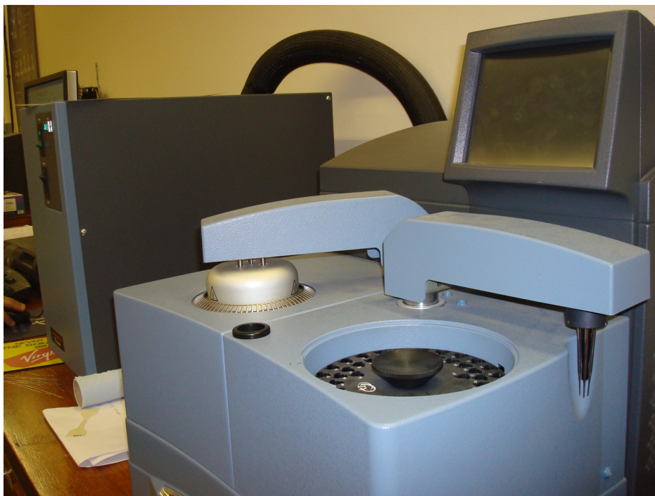
Figure 3.8 Sample holder of the DSC where sample is placed before transferring to the cell
