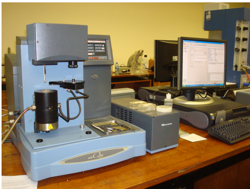
Figure 3.10 Platinum pan with the sample holds by the beam balance before placed in the oven
