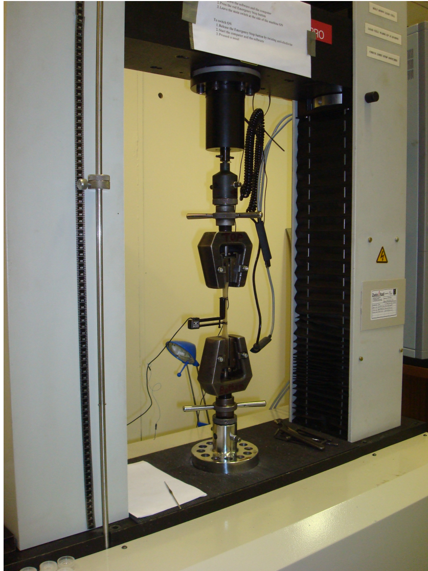
Figure 3.5 A dumbbell specimen set up in the tensometer before the test
