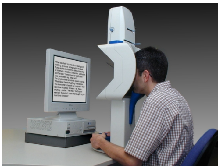
Figure 3.5: Eye tracking device used in the research (source from SensoMotoric Instruments GmbH)
