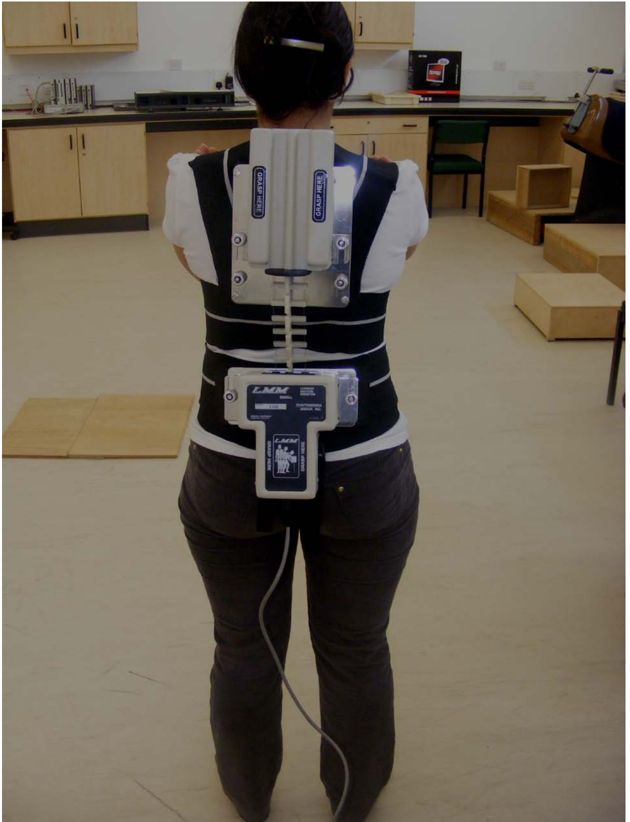
Fig. 3.1: The Lumbar Motion Monitor exoskeleton
