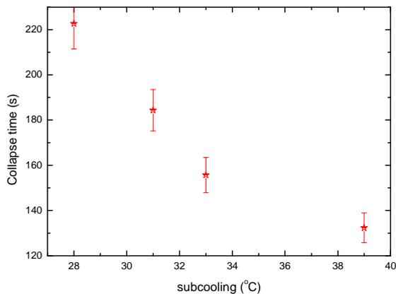
Figure 5: Final collapse time of a bubble of FC-72 vapour as a function of the degree of subcooling  $\Delta T_{sub}$ .
