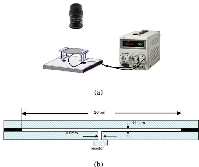
Figure 2: (a) A sketch of the test rig and power source, and (b) a diagram showing the location of the resistor and the geometry of the plate.
