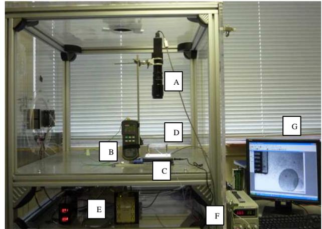
Figure 1: Experimental apparatus: (A) high speed CCD camera, (B) thermocouple and digital thermometer, (C) backlight, (D) test rig, (E) thermal regulation system, (F) power supply, and (G) image processing system.
