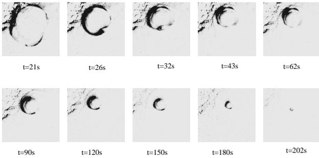
Figure 3: Images showing the collapse of a bubble of FC-72 vapour in the case  $\Delta T_{sub} = 36.1^\circ\text{C}$ .
