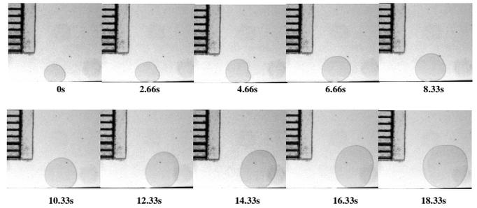
Figure 6: Images showing the expansion of a bubble of FC-72 vapour in the case  $\Delta T_{sup} = 3.9^\circ\text{C}$ .
