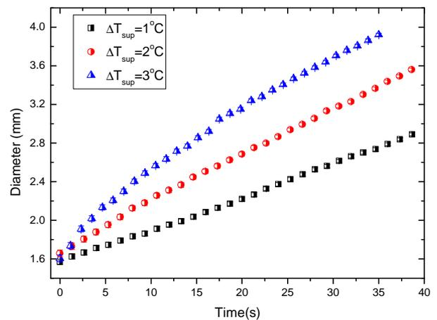
Figure 7: Evolution of the diameter of a bubble of FC-72 vapour as a function of time in the superheated case.
