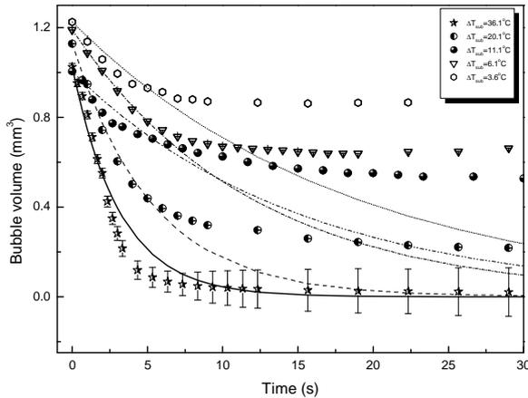
Figure 9: Comparison between the experimentally measured values of the volume of the bubble (symbols) and the corresponding fitted theoretical predictions given by equation (6) (curves) for a range of values of the subcooling  $\Delta T_{sub}$ .
