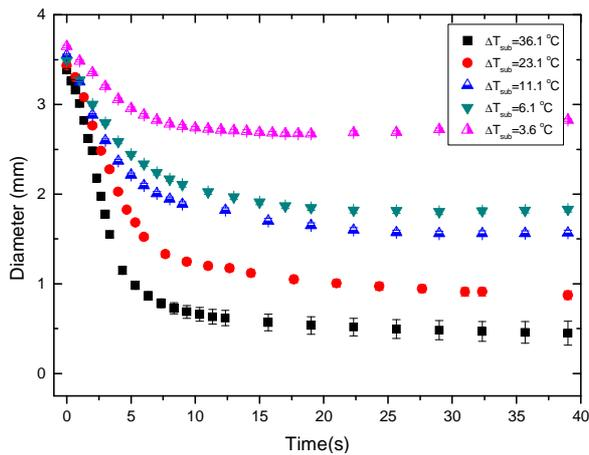
Figure 4: Evolution of the diameter of a bubble of FC-72 vapour as a function of time in the subcooled case.
