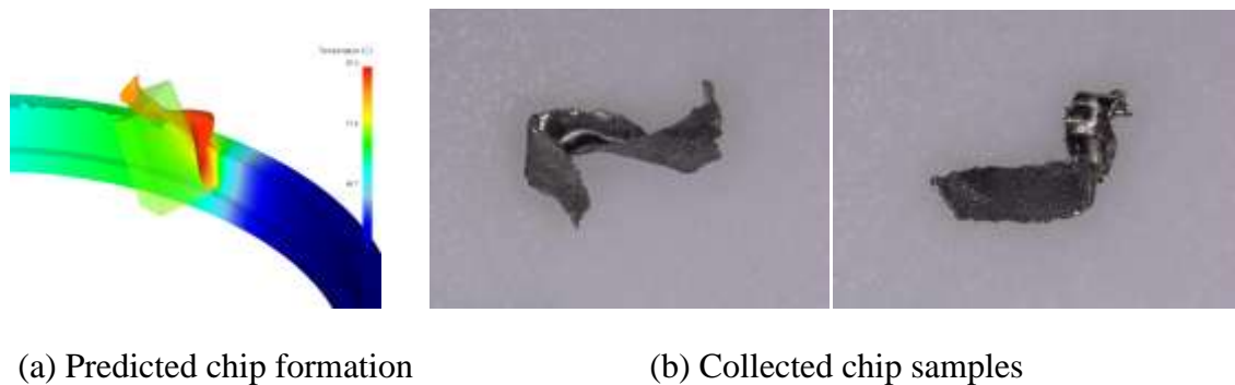
Fig. 3.14 Comparison of predicted chip formation with collected chip samples
