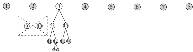
Figure 6.4: Coarsening of elements 9 and 10.
