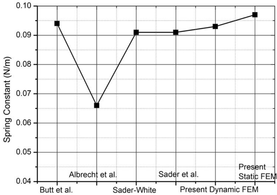
254 Fig. 9 Comparison of the stiffness of the V-shaped beam obtained by different methods.
